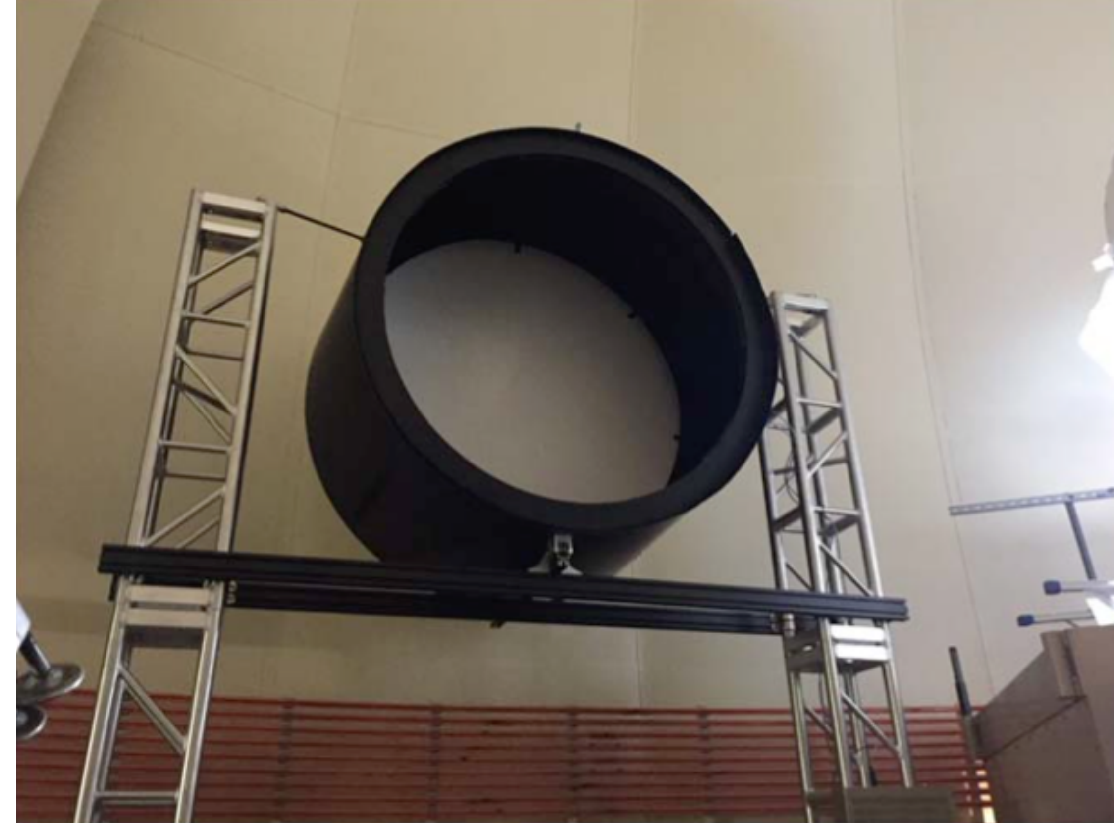
Flat-field illuminator (32 pulsed LEDs per colour)
