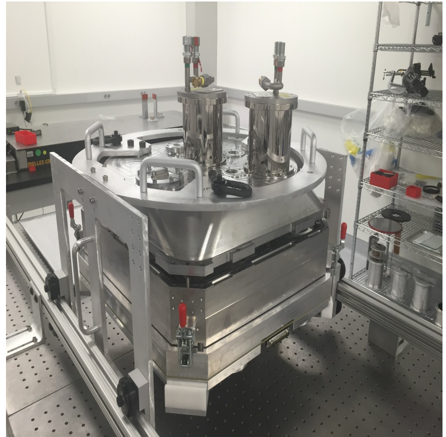
Sliding rig for backplate and lifting fixture for enclosure.
