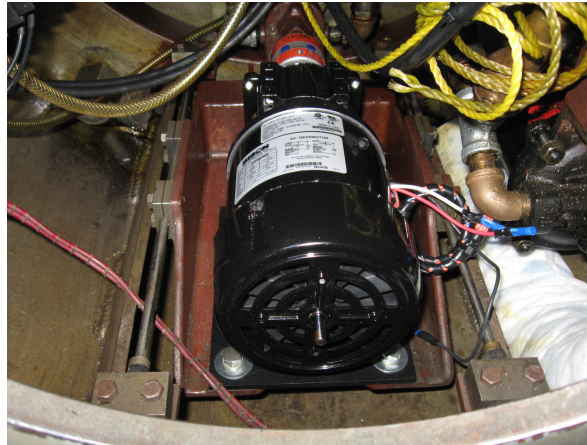
New oil pump for Dec drive worm gear
