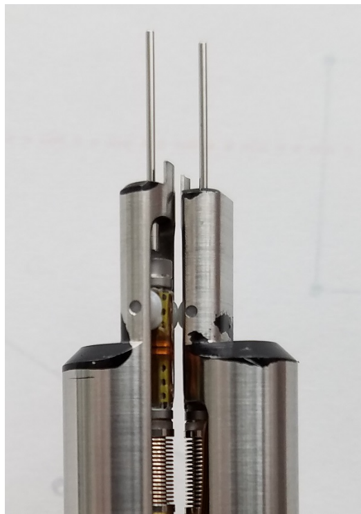
Fig 1: Two Cobras making contact with each other when installed in adjacent positions on 2 separate rails on COB
