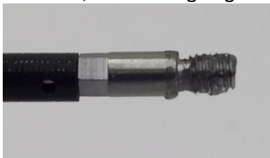
Fig 5: An example of greased stud
