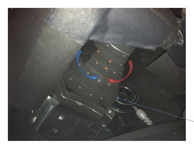
Collimator assembly can rotate over a range of about 15deg before flange lobes come in contact with the v-block (extreme CW direction shown by red arrow) or the shutter (extreme CCW direction shown by blue arrow).
