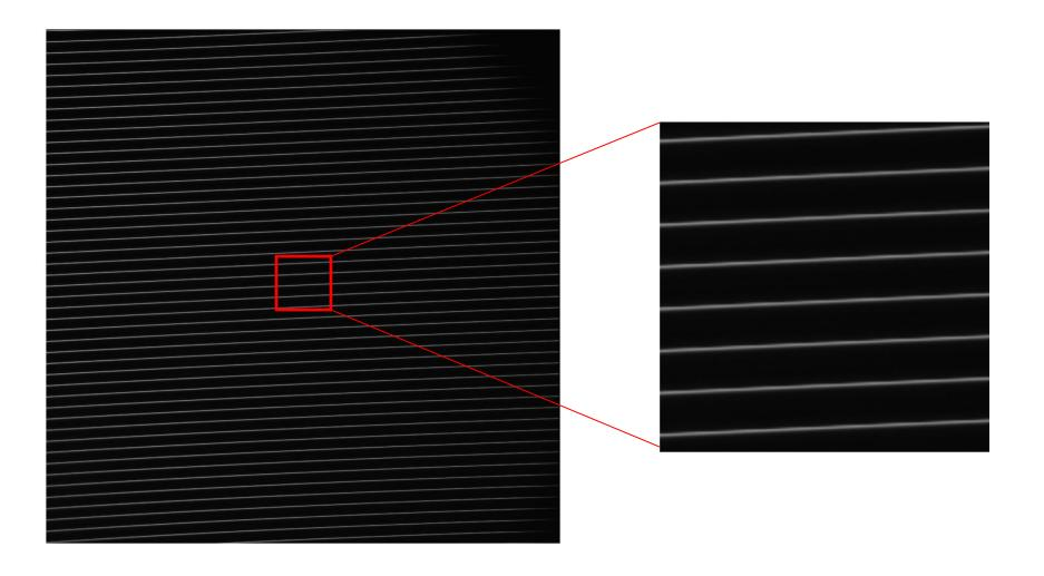
For the test exposure (~11am on 5/12/2016) the collimator was oriented near the CCW limit to provide a separation of about 15 pixels (Halogen lamp image below) required for data pipeline background subtraction to work.
