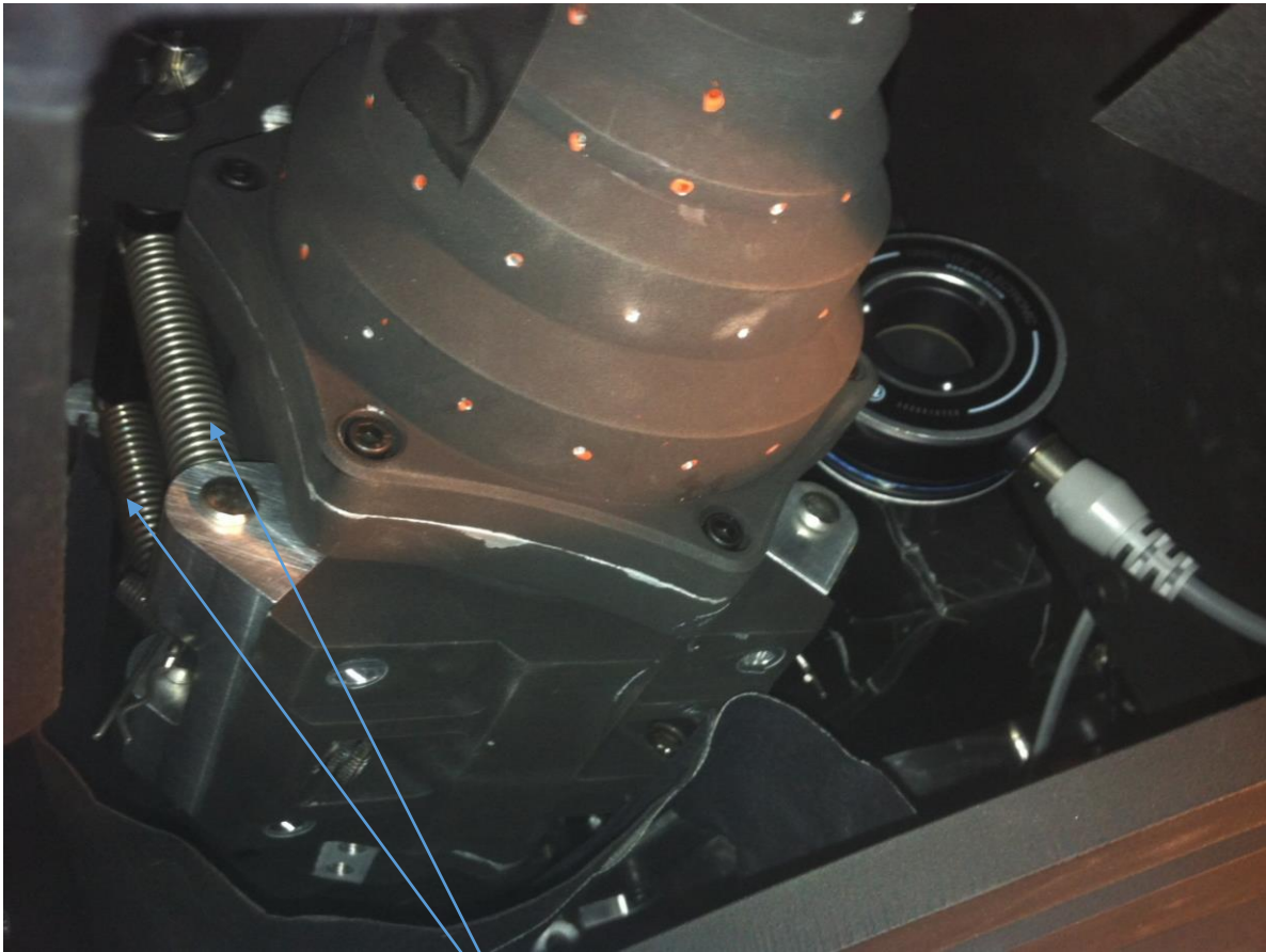
Original configuration – collimator clamped with tension springs
