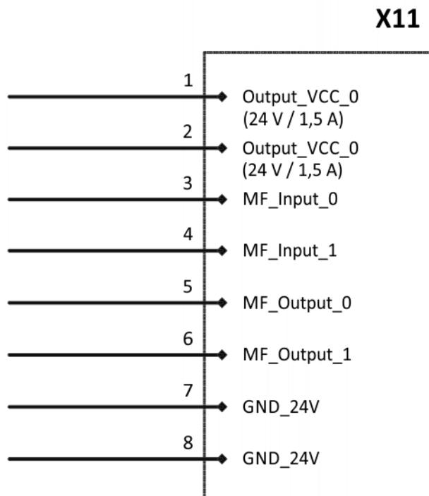
Fig. 6-12: Wiring diagram, MF IO pneumatic, X11
