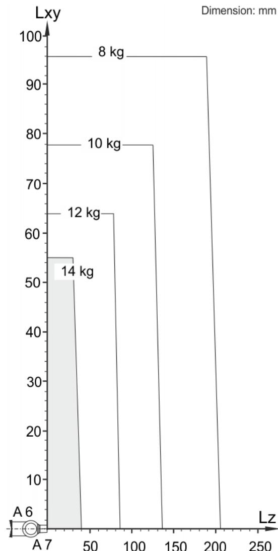
**Fig. 4-56: Payload diagram, LBR iiwa 14 R820**
