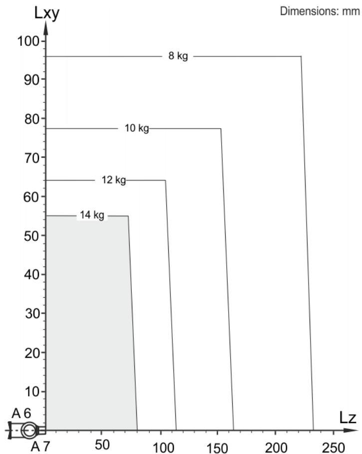
**Fig. 4-86: LBR iiwa 14 R820 payload diagram**
