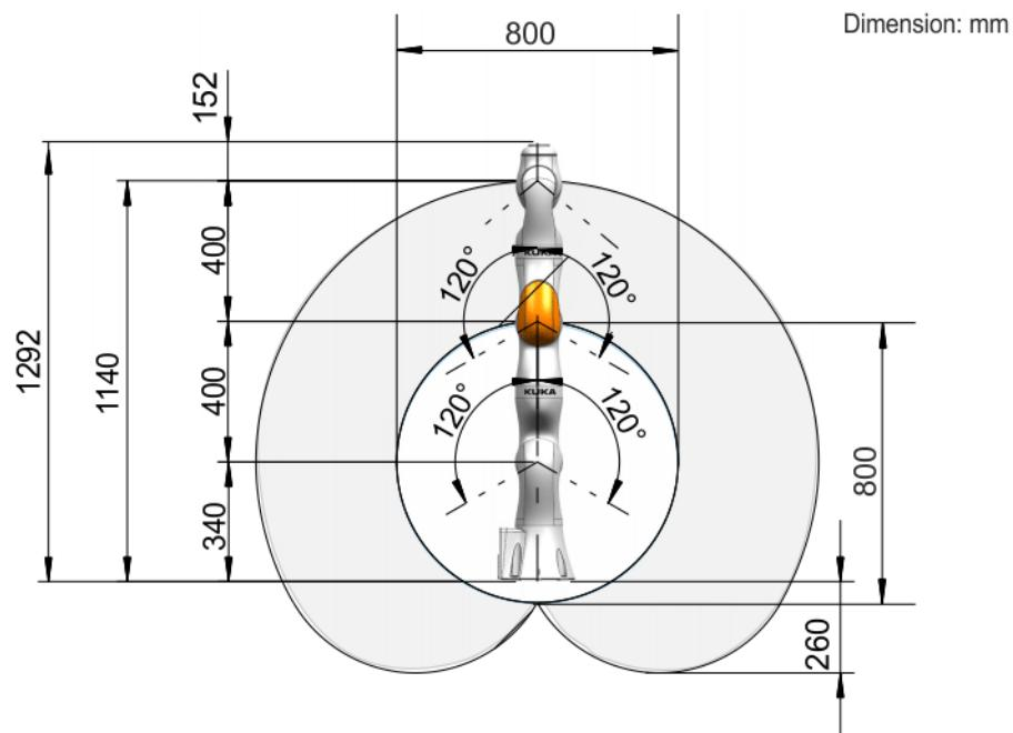
**Fig. 4-77: Working envelope, LBR iiwa 7 R800, side view**
