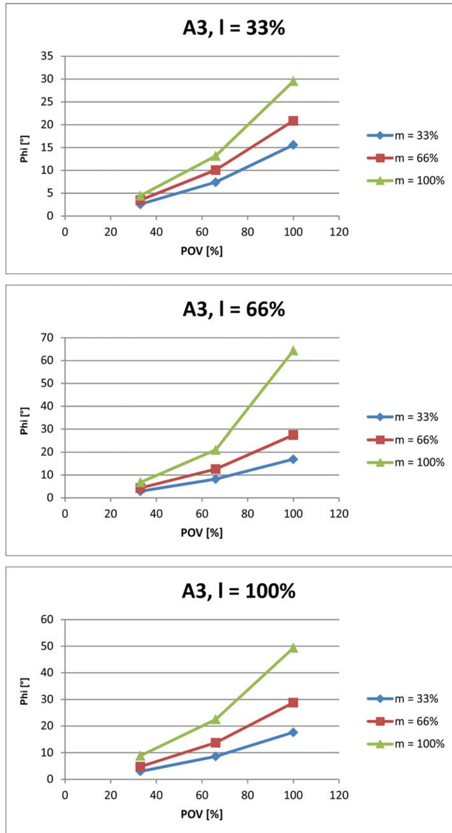
**Fig. 4-133: Stopping distances for STOP 1, axis 3**
