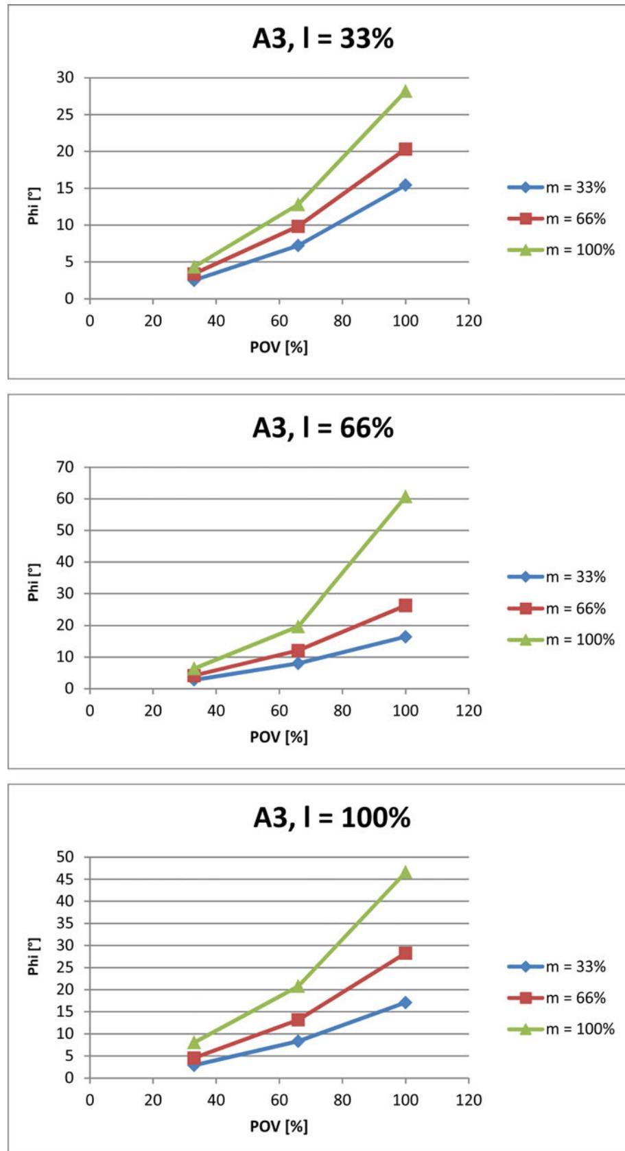
**Fig. 4-117: Stopping distances for STOP 1, axis 3**
