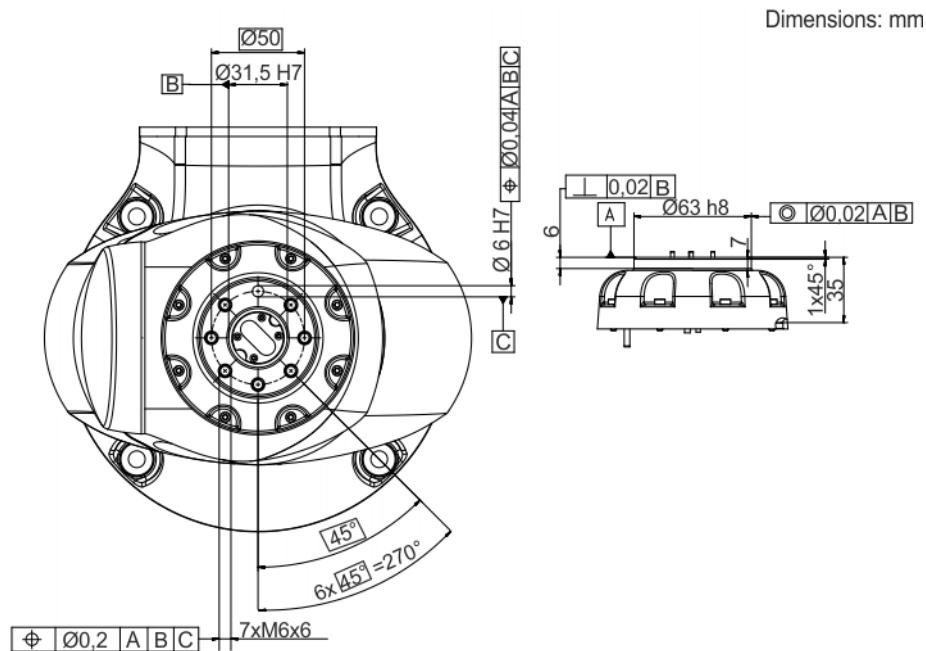
**Fig. 4-81: Dimensions, media flange Inside electrical**
