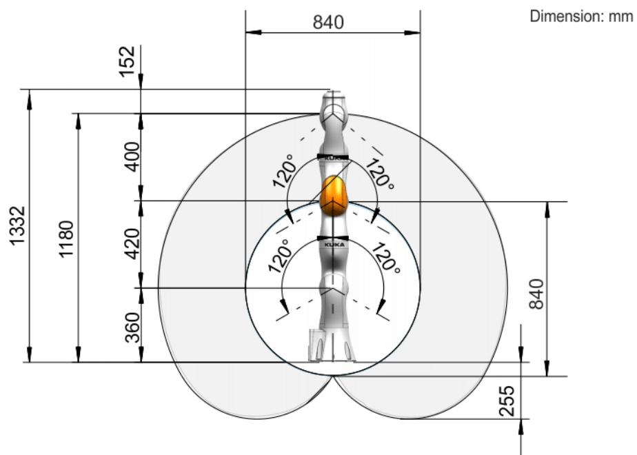
Fig. 4-49: Working envelope, LBR iiwa 14 R820, side view
