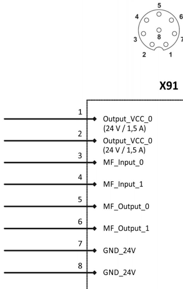
Fig. 6-33: Wiring diagram, connection X91
