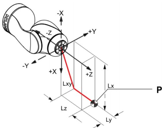
**Fig. 4-93: Load center of gravity**
