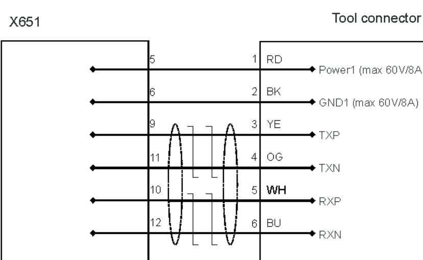
**Fig. 6-38: Wiring diagram, MF Inside electrical, X651, tool connector**
