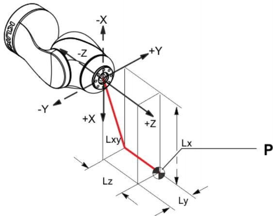
**Fig. 4-95: Load center of gravity**
