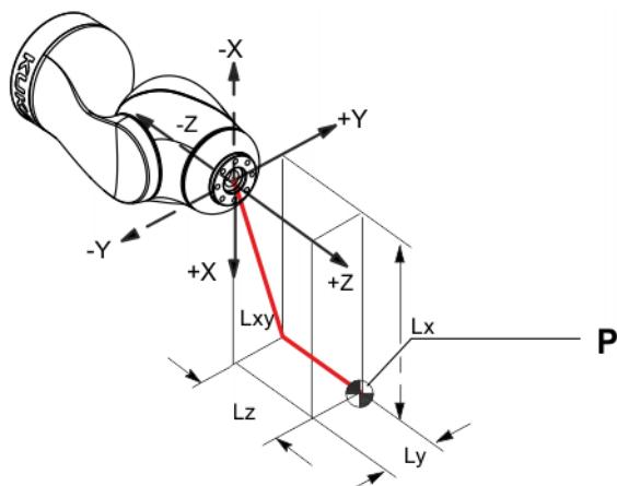
Fig. 4-23: Load center of gravity
