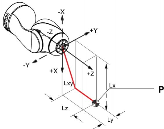
**Fig. 4-63: Load center of gravity**
