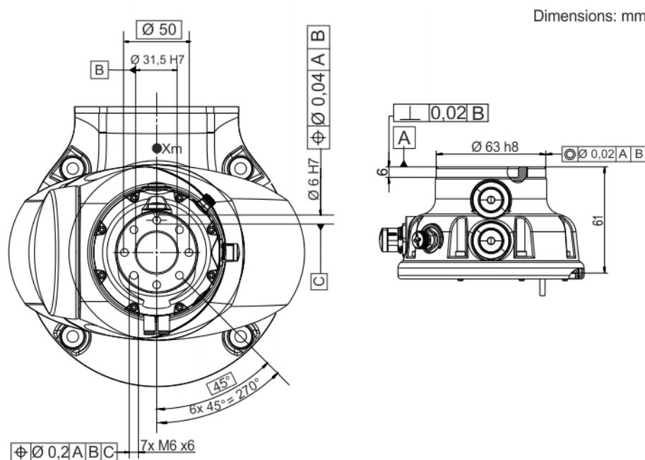
**Fig. 4-41: Dimensions, media flange Touch pneumatic**
