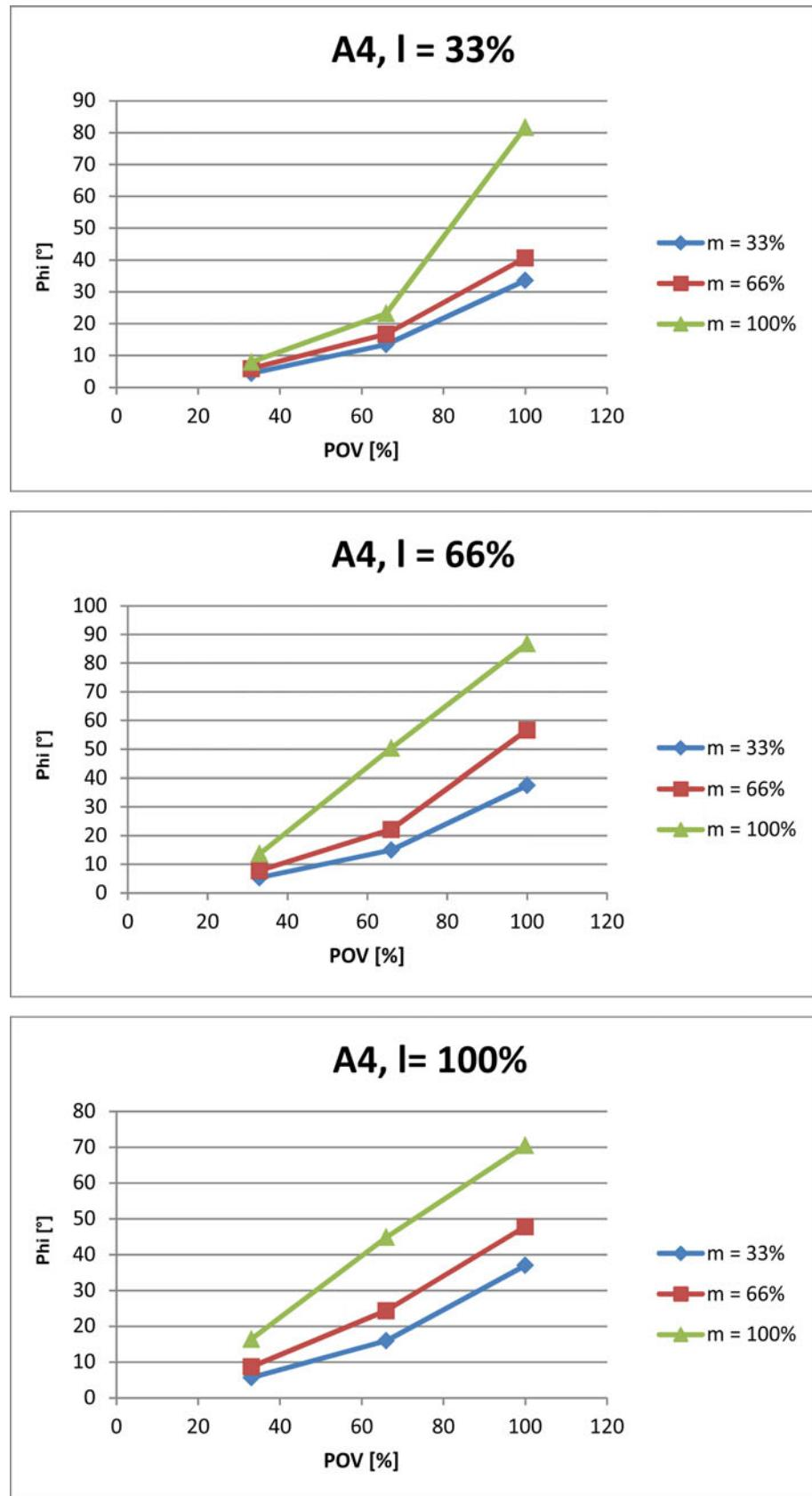
Fig. 4-127: Stopping distances for STOP 1, axis 4
