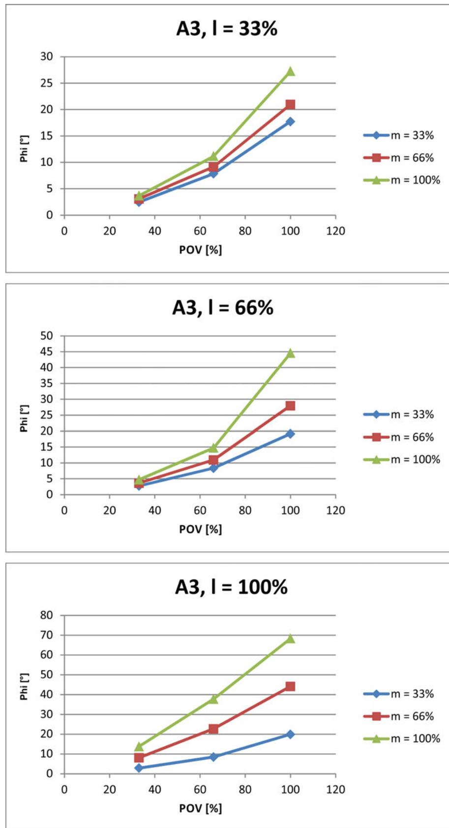
Fig. 4-109: Stopping distances for STOP 1, axis 3
