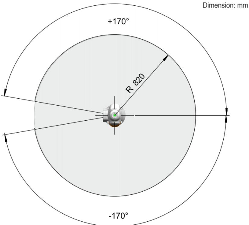
Fig. 4-70: LBR iiwa 14 R820 working envelope, top view
