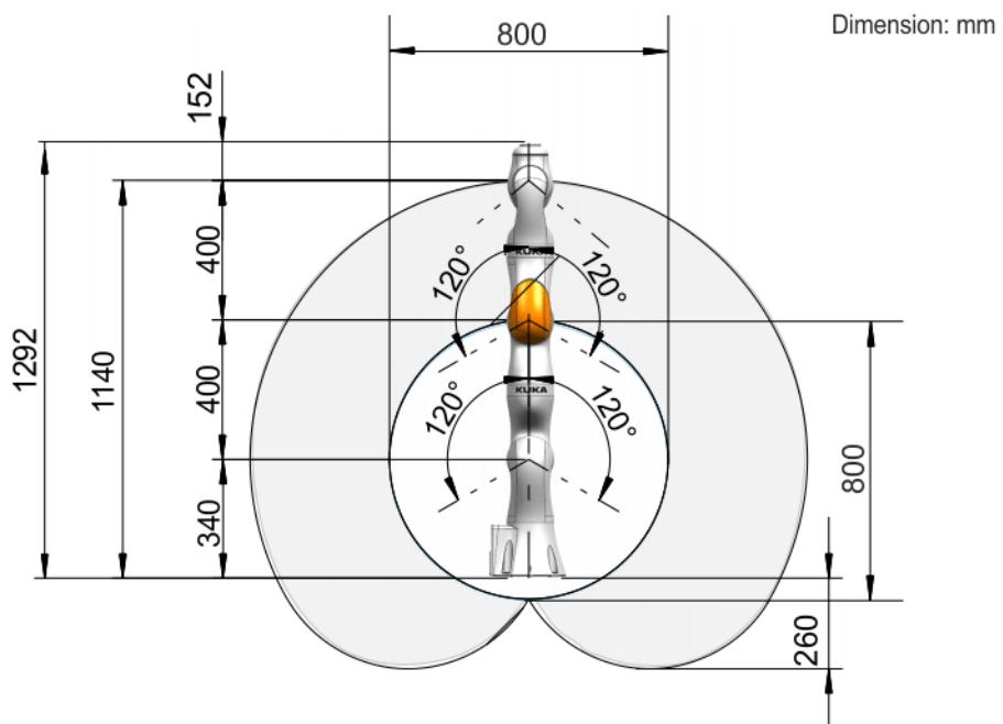
Fig. 4-47: Working envelope, LBR iiwa 7 R800, side view
