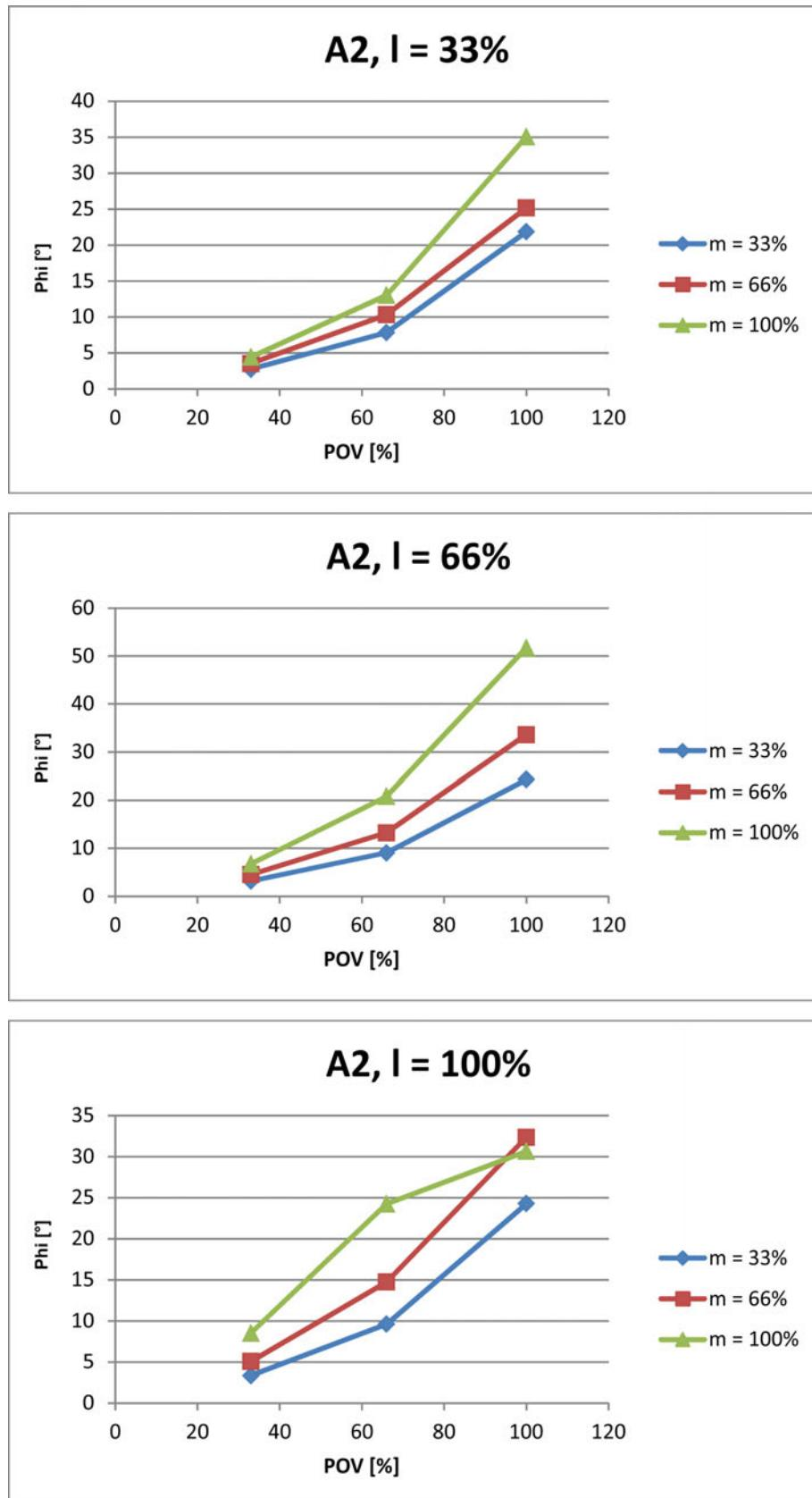
Fig. 4-115: Stopping distances for STOP 1, axis 2
