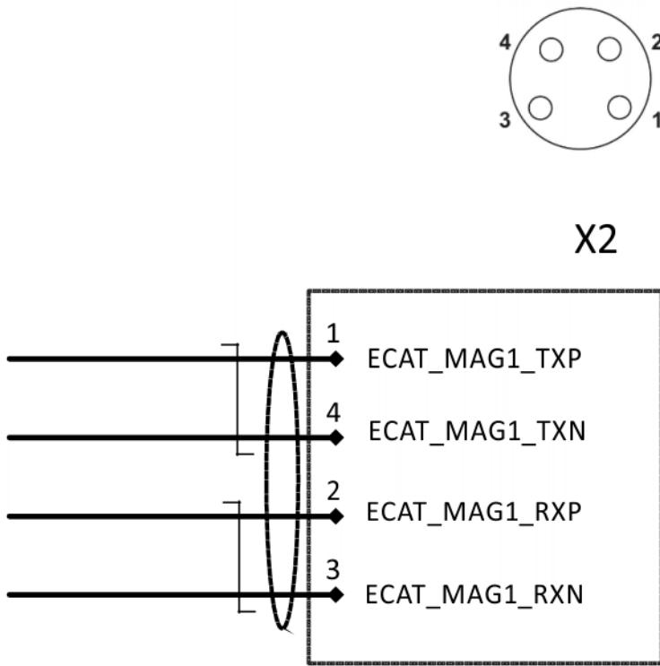
Fig. 6-36: Wiring diagram, connection X2
