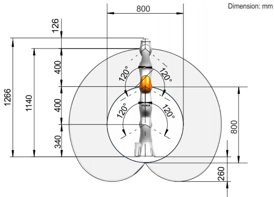
Fig. 4-7: Working envelope, LBR iiwa 7 R800, side view
