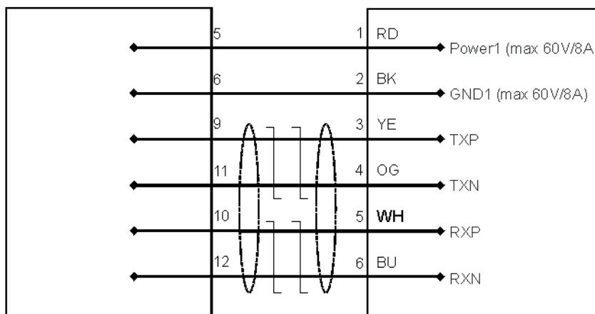
Fig. 6-41: Wiring diagram, MF Inside pneumatic, X651, tool connector
