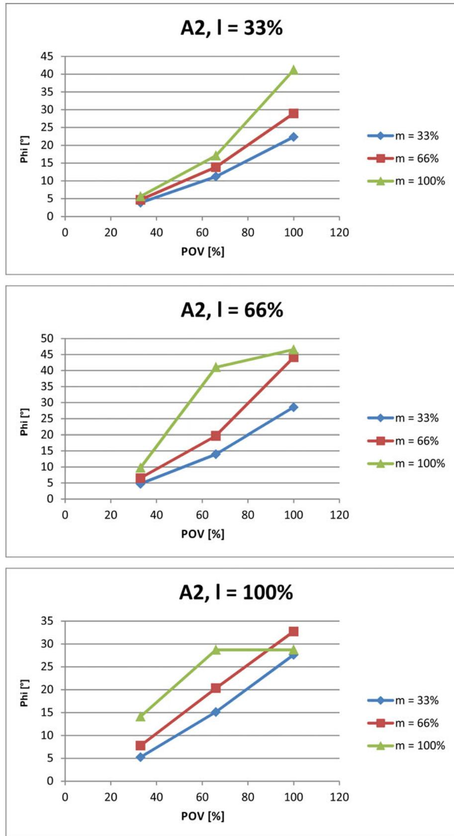
Fig. 4-107: Stopping distances for STOP 1, axis 2
