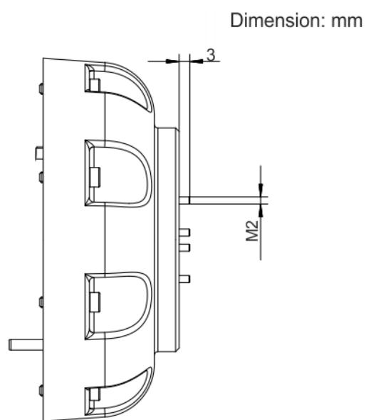
**Fig. 6-46: Dimensions, tool connector, side view****6.2.13 Tool connector, media flange Inside pneumatic****Description**
