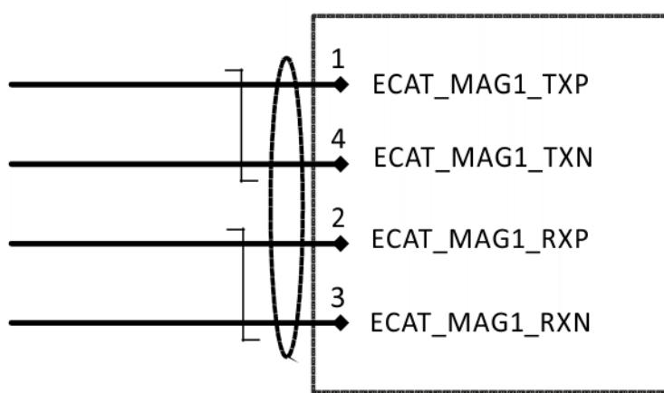
Fig. 6-15: Wiring diagram, connection X2
