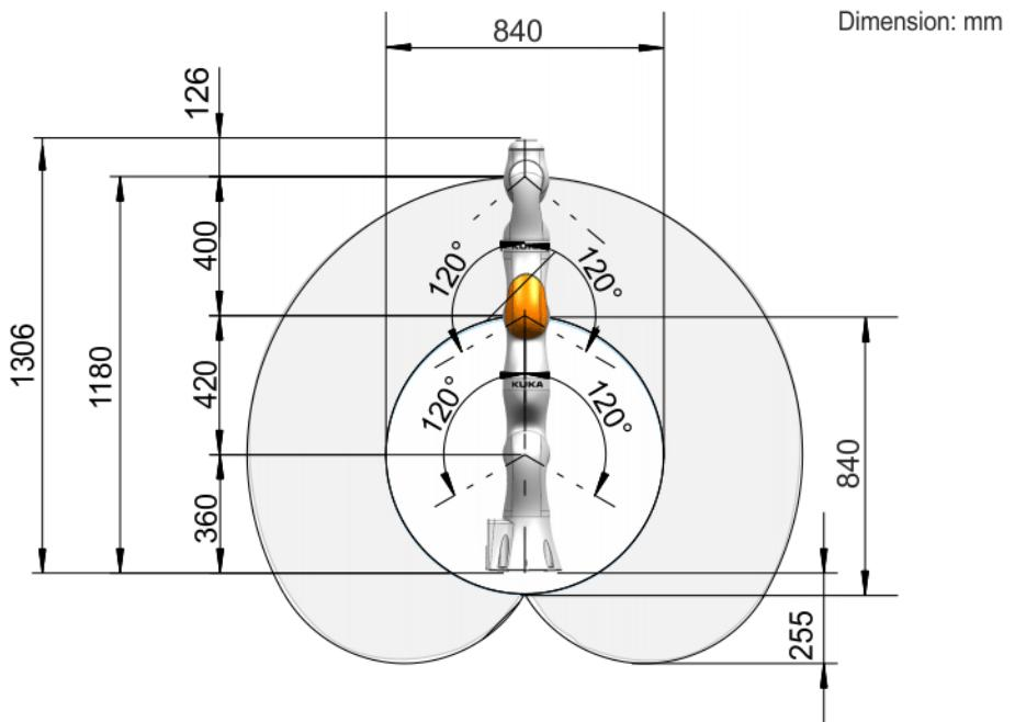
Fig. 4-99: Working envelope, LBR iiwa 14 R820, side view
