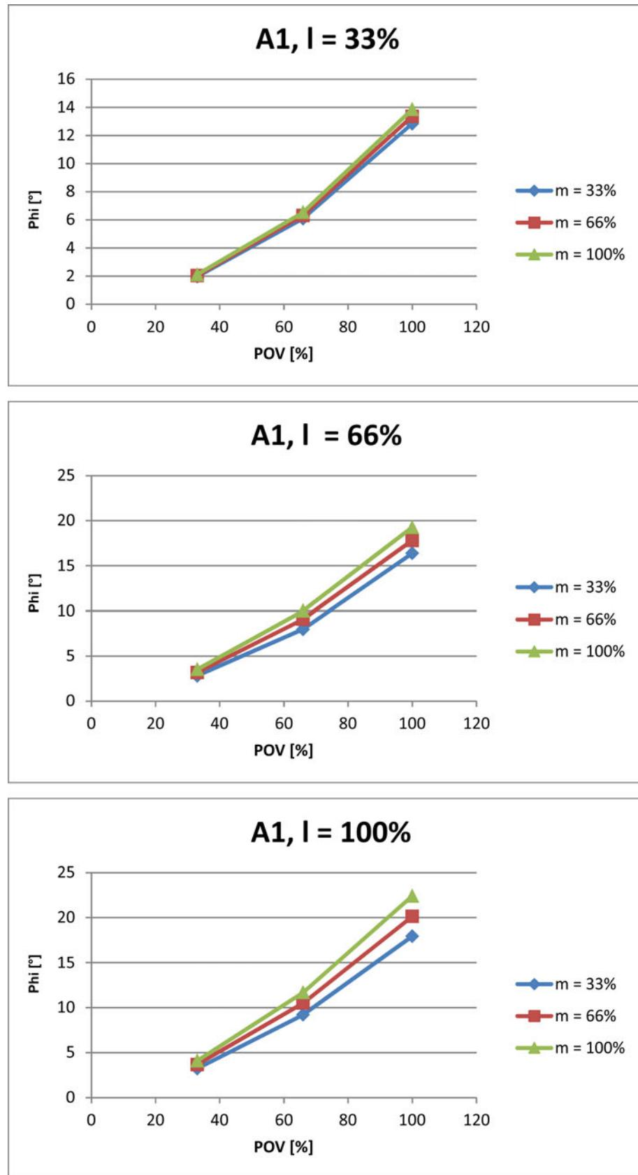
Fig. 4-121: Stopping distances for STOP 1, axis 1
