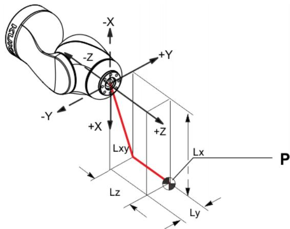
**Fig. 4-45: Load center of gravity**
