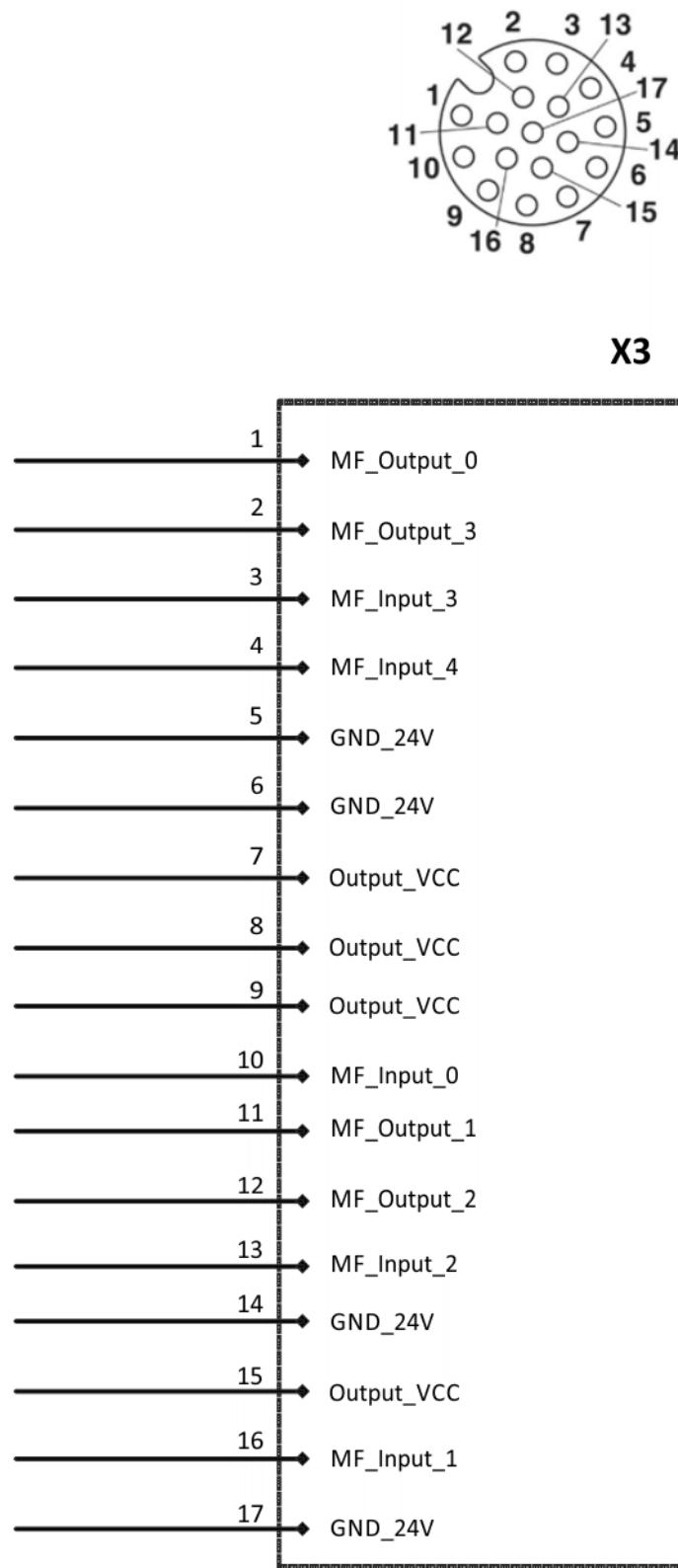
Fig. 6-20: Wiring diagram, connection X3
