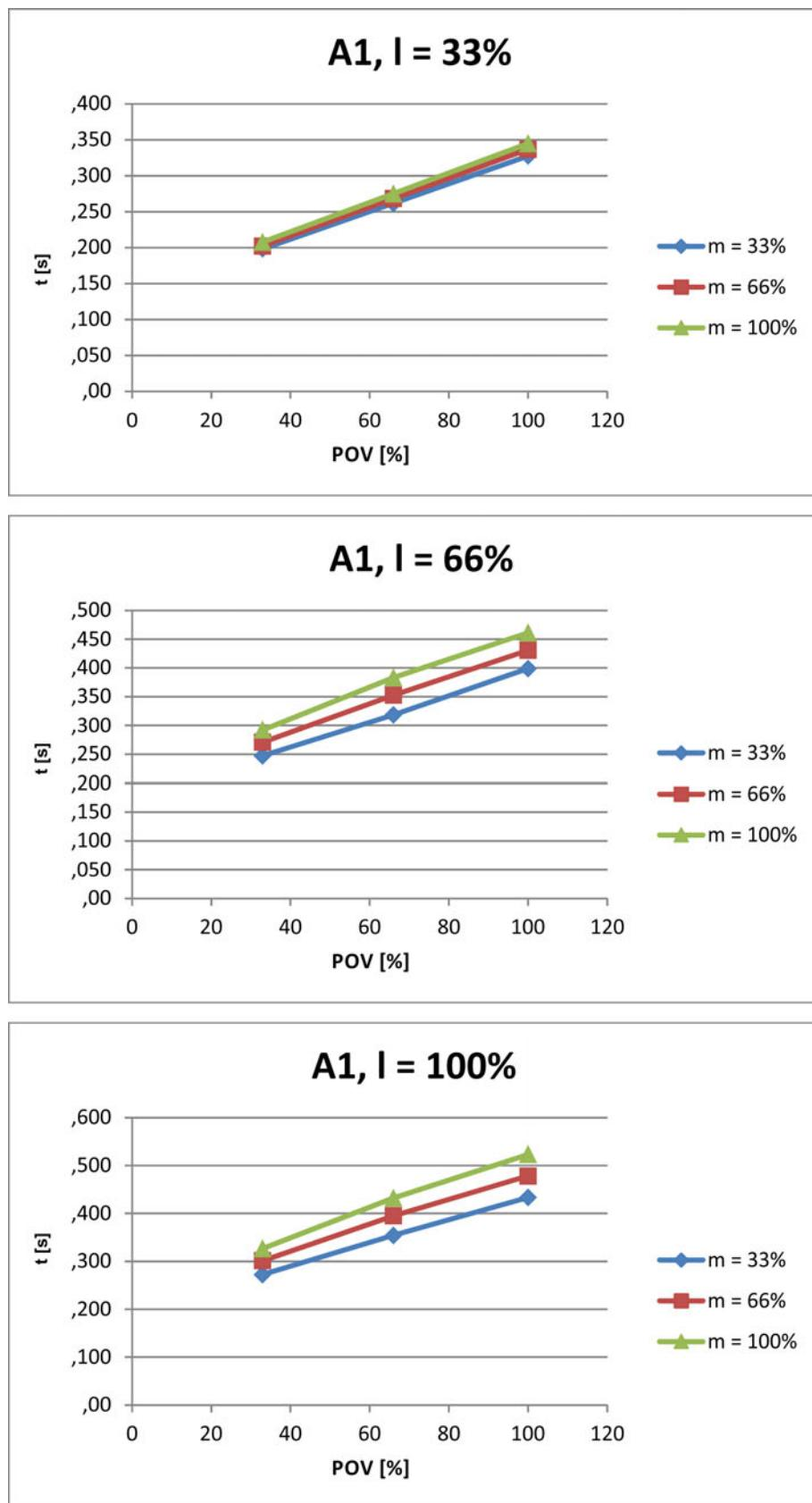
Fig. 4-106: Stopping times for STOP 1, axis 1
