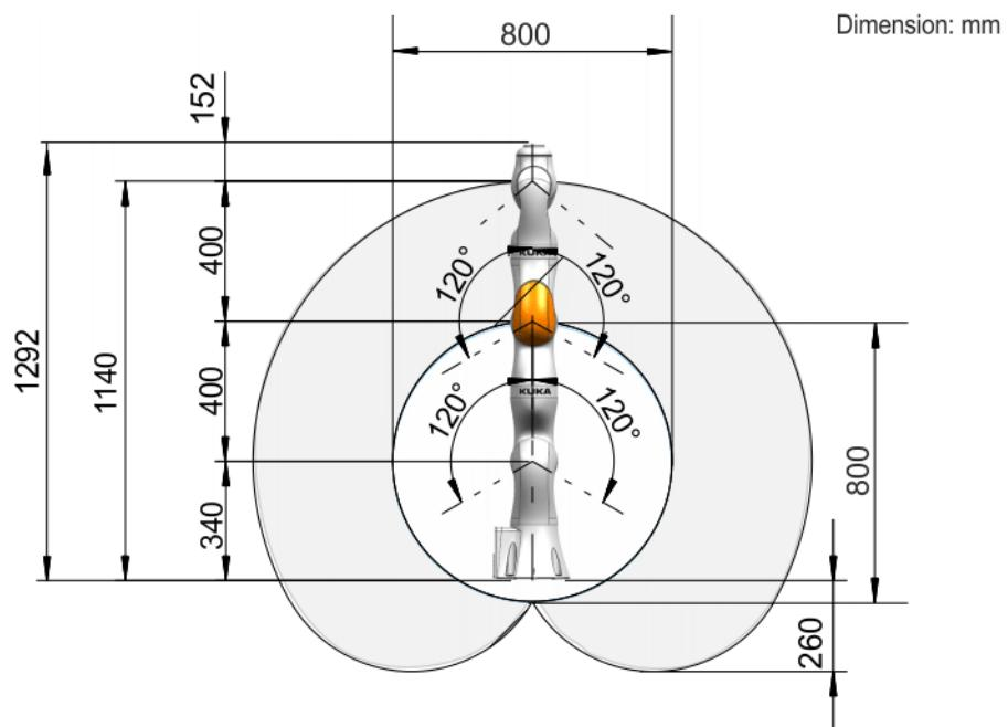
Fig. 4-57: Working envelope, LBR iiwa 7 R800, side view
