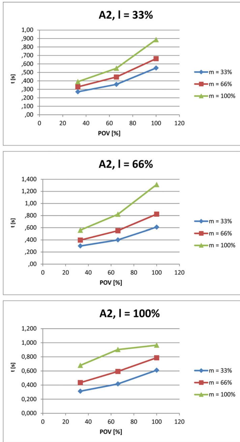
Fig. 4-116: Stopping times for STOP 1, axis 2
