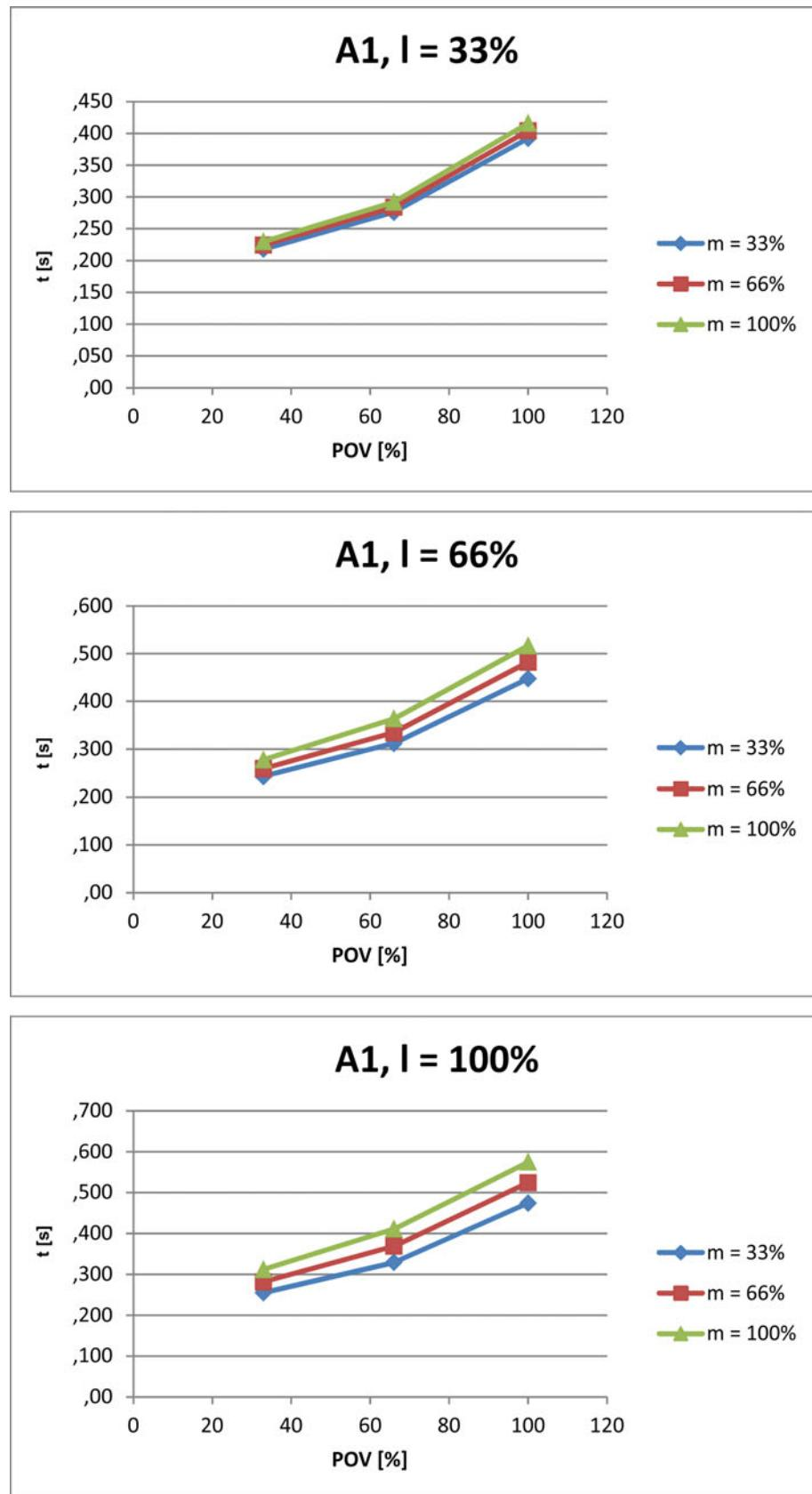
Fig. 4-130: Stopping times for STOP 1, axis 1
