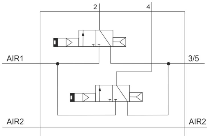
Fig. 6-32: Circuit diagram of pneumatic valves
