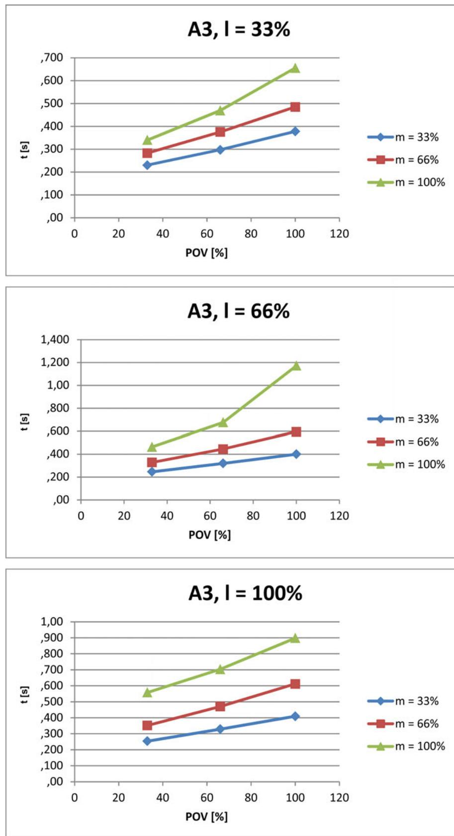
Fig. 4-118: Stopping times for STOP 1, axis 3
