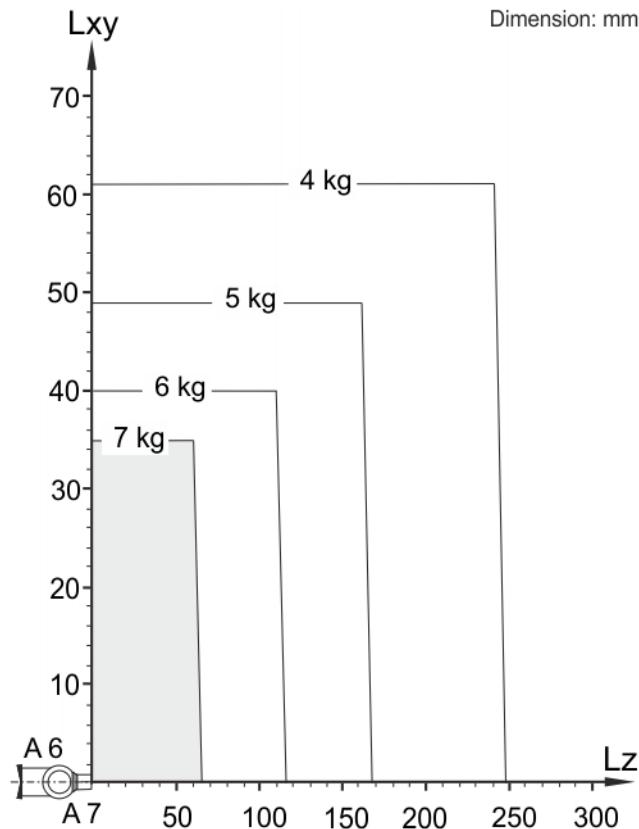
**Fig. 4-54: Payload diagram, LBR iiwa 7 R800**
