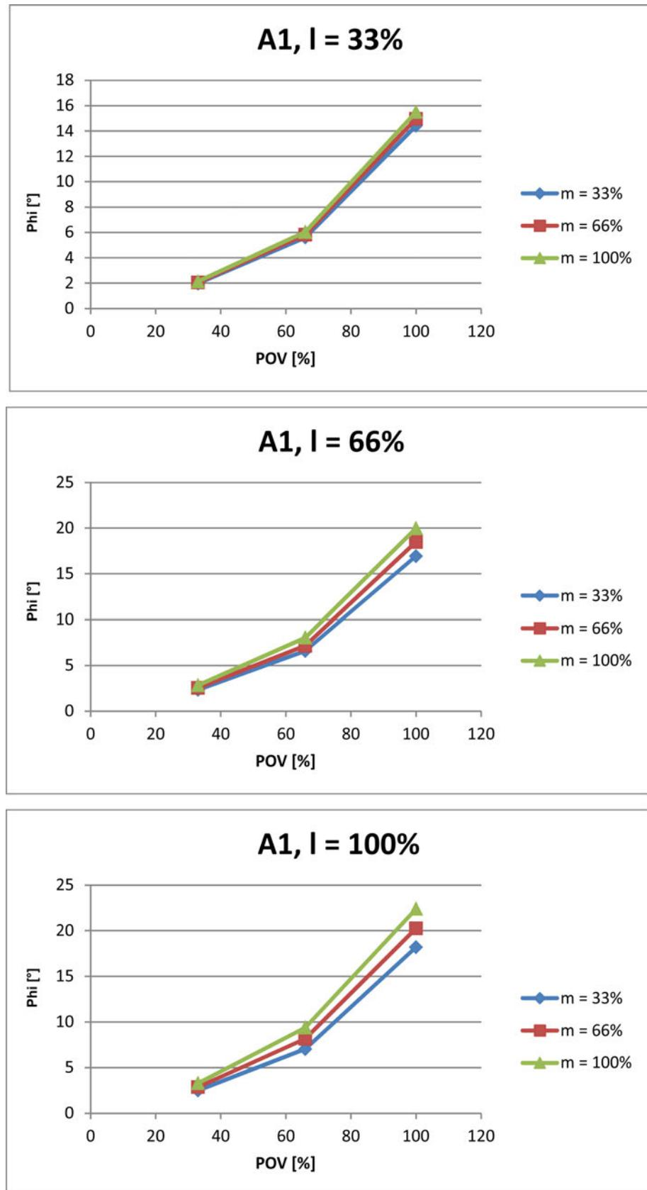
Fig. 4-129: Stopping distances for STOP 1, axis 1
