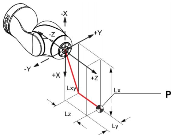
**Fig. 4-55: Load center of gravity**
