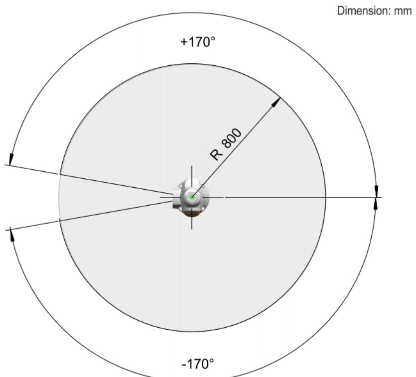
Fig. 4-8: LBR iiwa 7 R800 working envelope, top view
