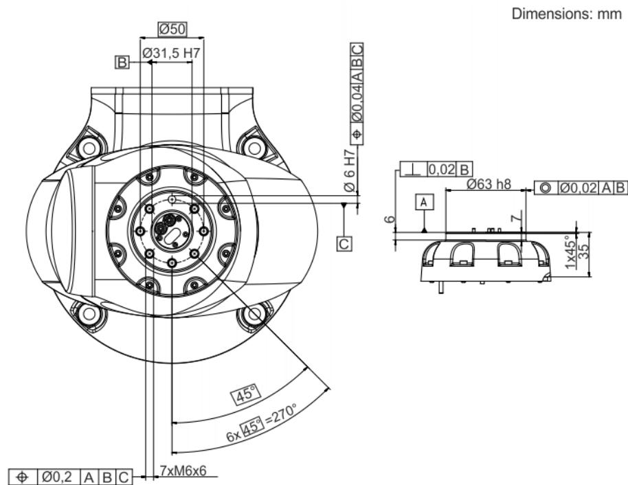
**Fig. 4-91: Dimensions, media flange Inside pneumatic**
