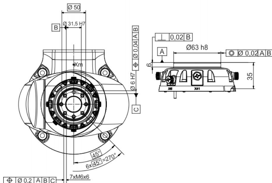
Fig. 4-61: Dimensions, media flange IO electrical
