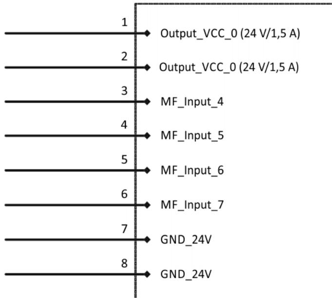
Fig. 6-14: Wiring diagram, MF IO pneumatic, X13
