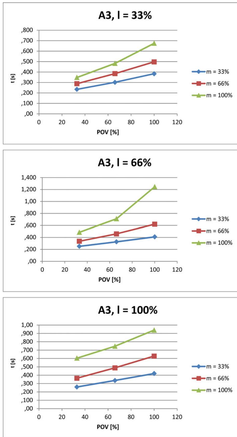
Fig. 4-134: Stopping times for STOP 1, axis 3
