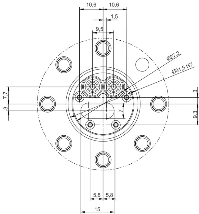
**Fig. 6-48: Dimensions, tool connector, top view**
