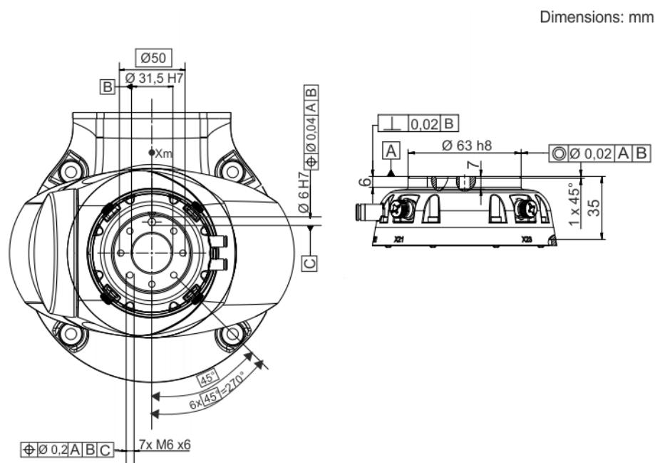
Fig. 4-21: Dimensions, media flange pneumatic
