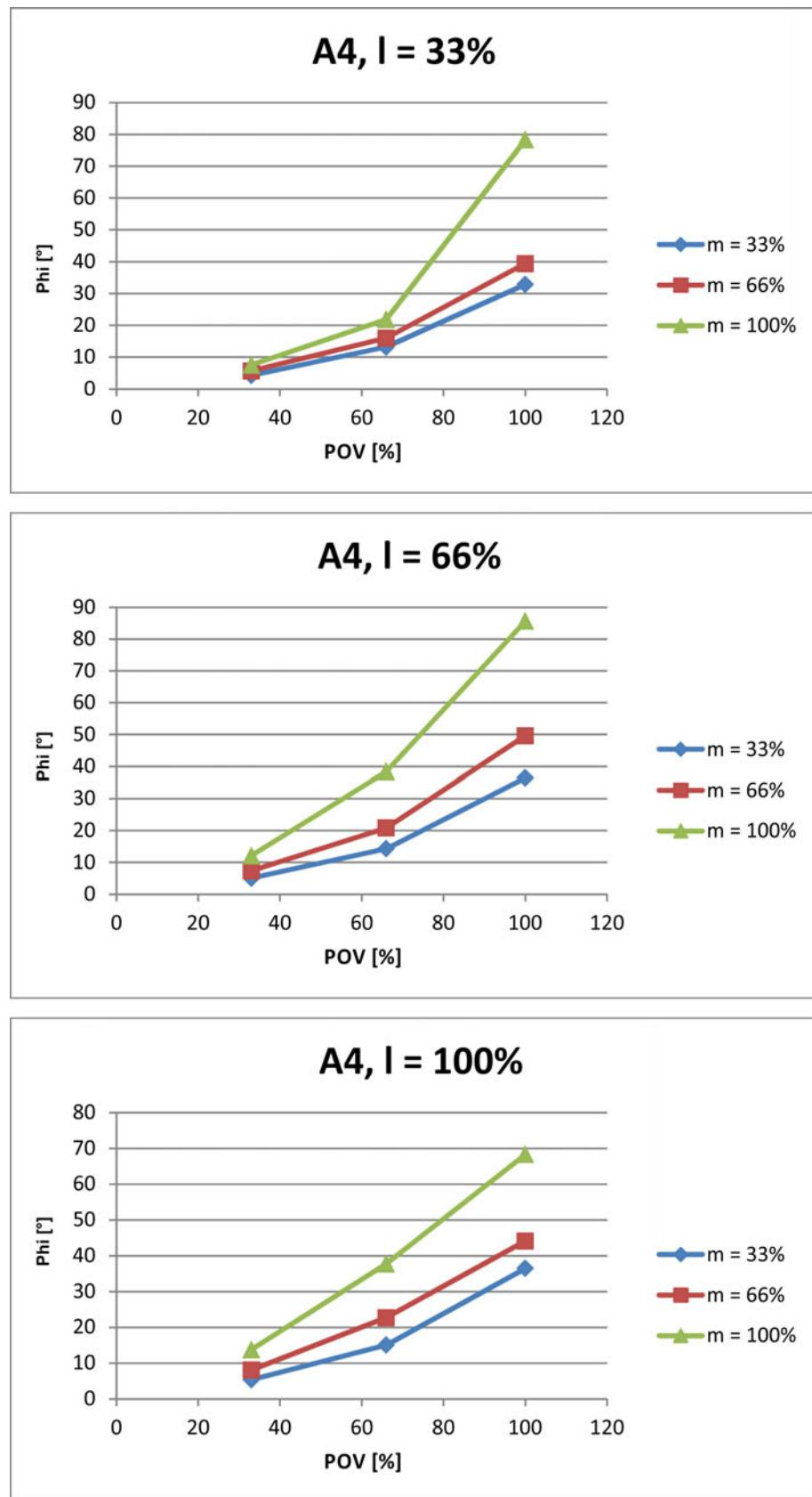
Fig. 4-111: Stopping distances for STOP 1, axis 4
