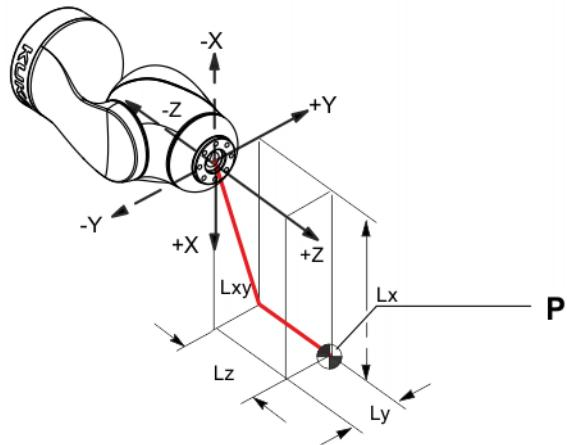
**Fig. 4-53: Load center of gravity**
