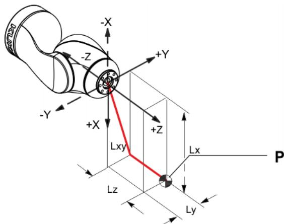
**Fig. 4-33: Load center of gravity**
