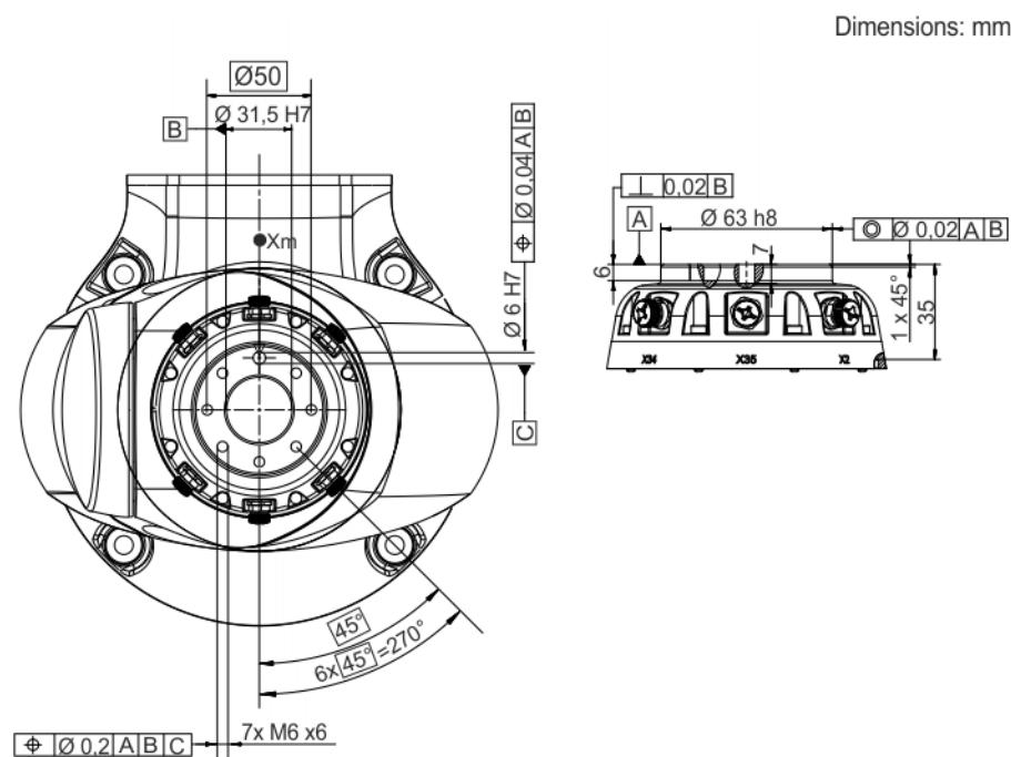
Fig. 4-11: Dimensions, media flange electrical
