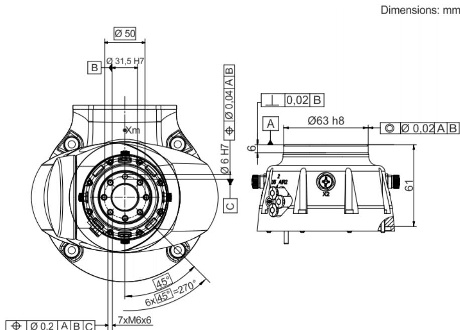
**Fig. 4-71: Dimensions, media flange IO valve pneumatic**
