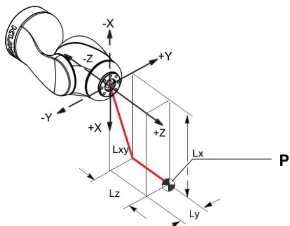
Fig. 4-73: Load center of gravity
