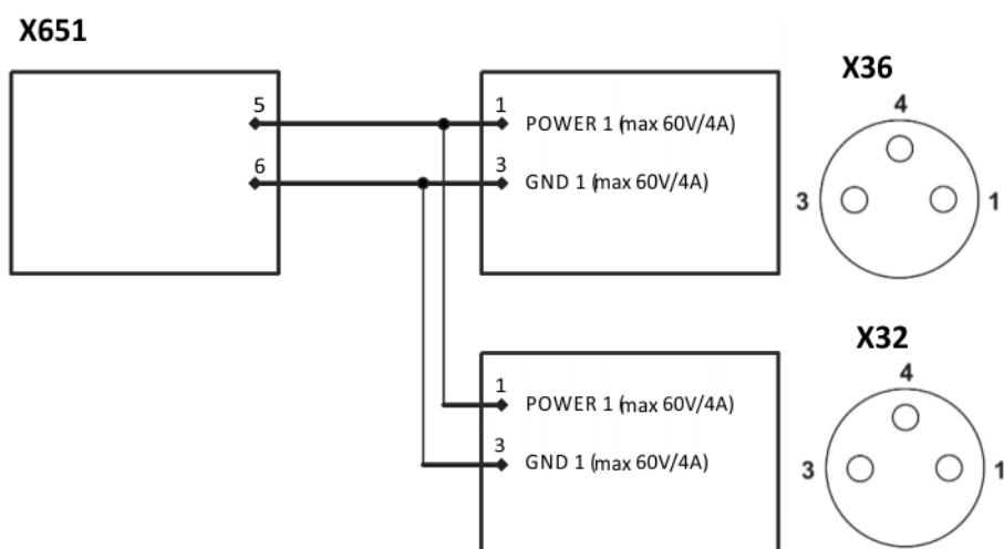
Fig. 6-4: Wiring diagram, MF electrical, X651, X32, X36
