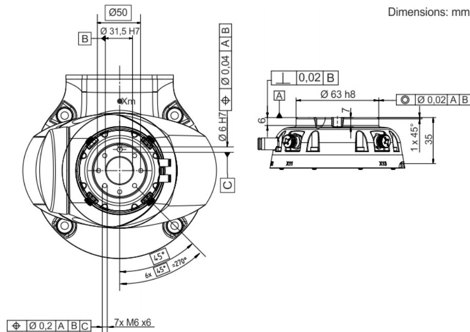
Fig. 4-31: Dimensions, media flange IO pneumatic
