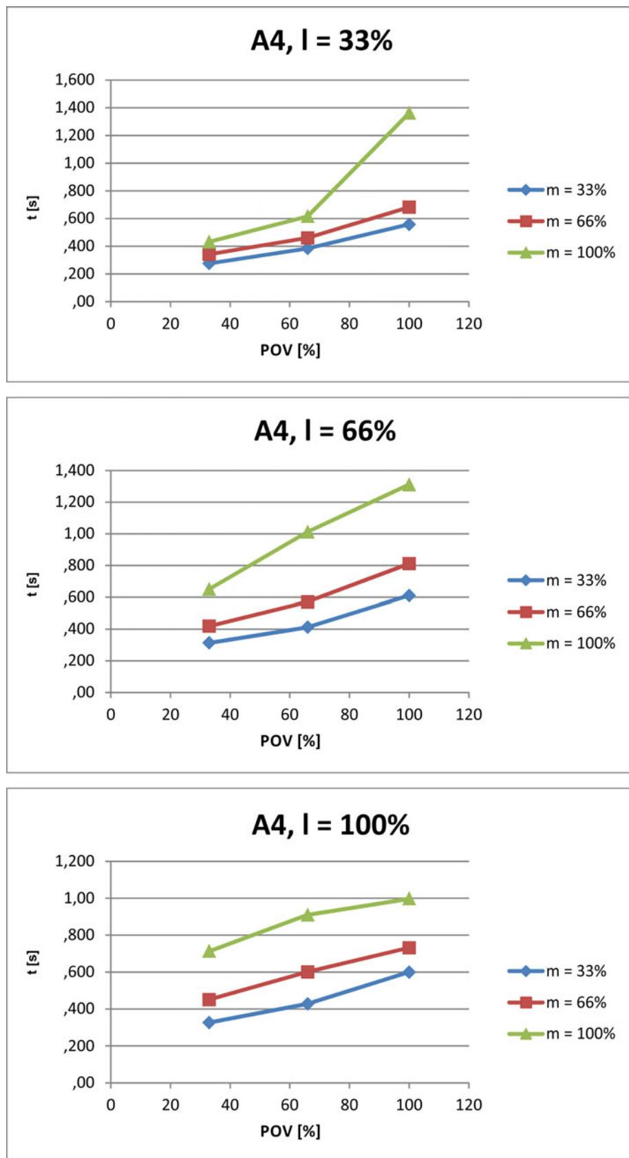
Fig. 4-112: Stopping times for STOP 1, axis 4
