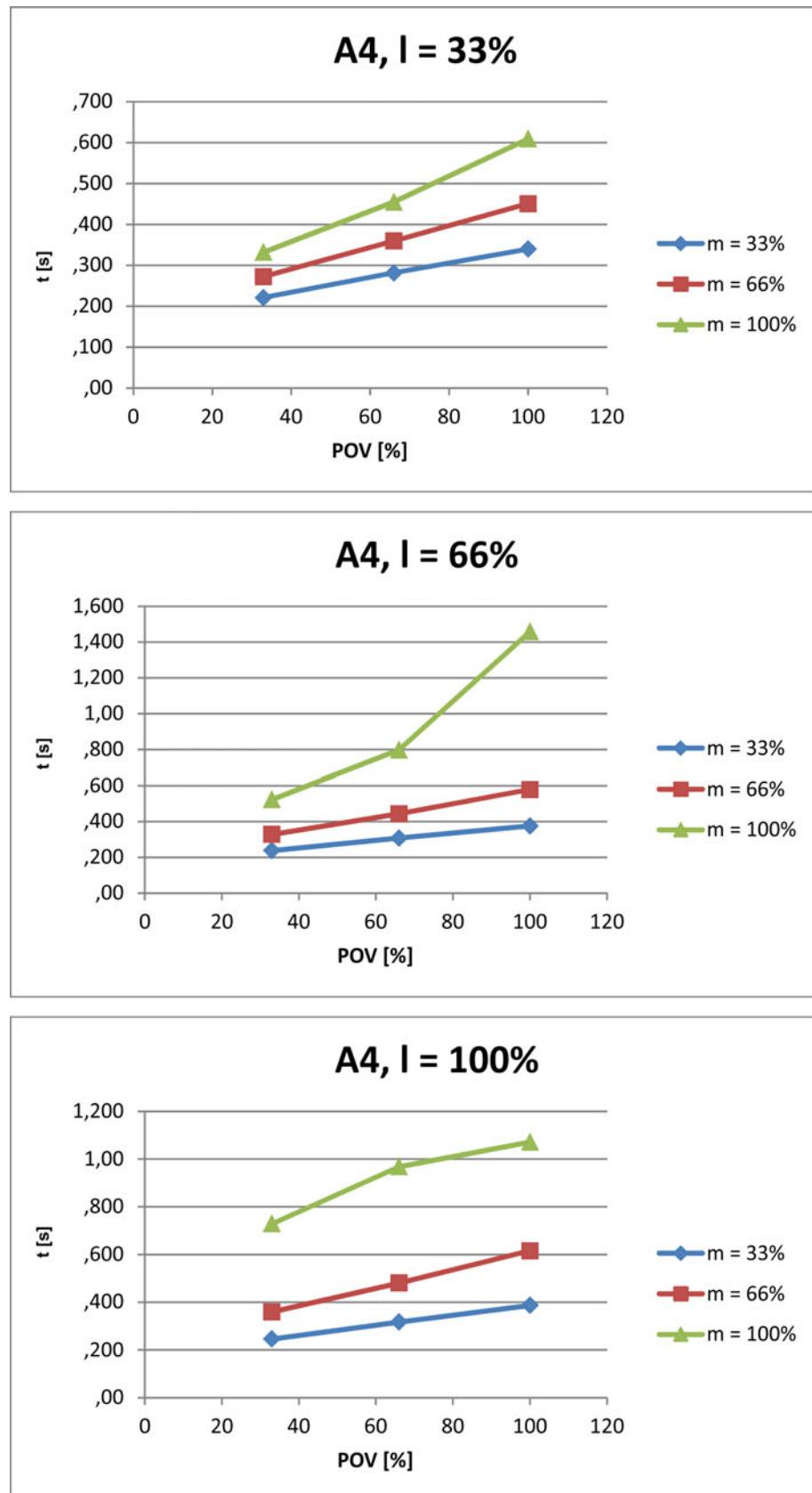
Fig. 4-136: Stopping times for STOP 1, axis 4
