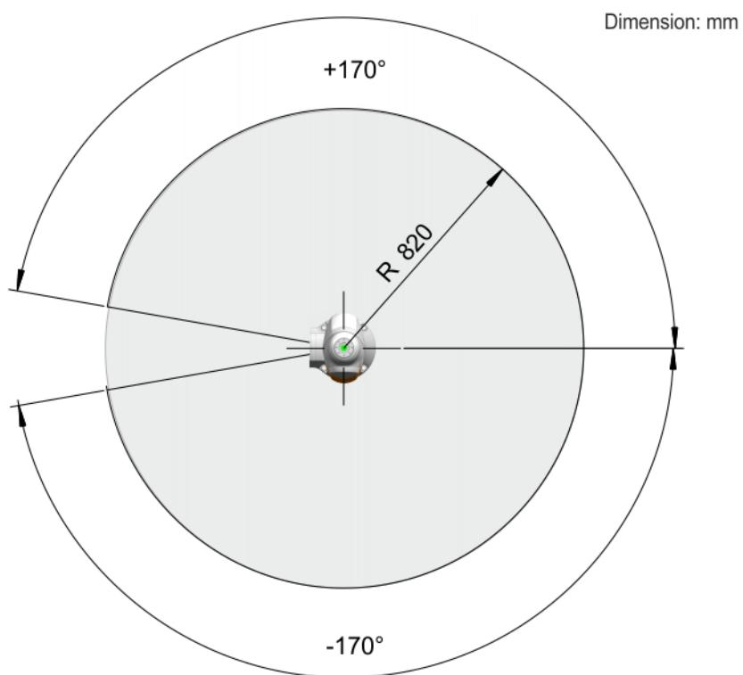
**Fig. 4-40: LBR iiwa 14 R820 working envelope, top view**
