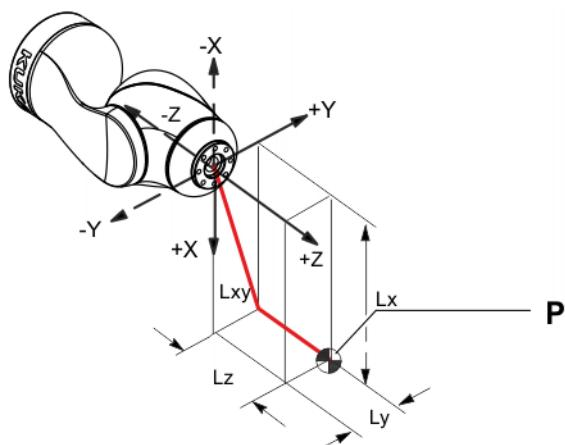
**Fig. 4-75: Load center of gravity**
