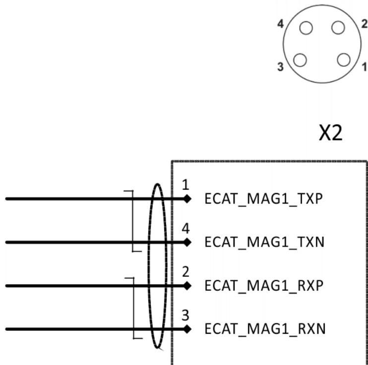
Fig. 6-30: Wiring diagram, connection X2
