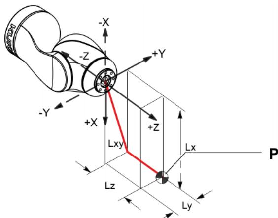
Fig. 4-13: Load center of gravity
