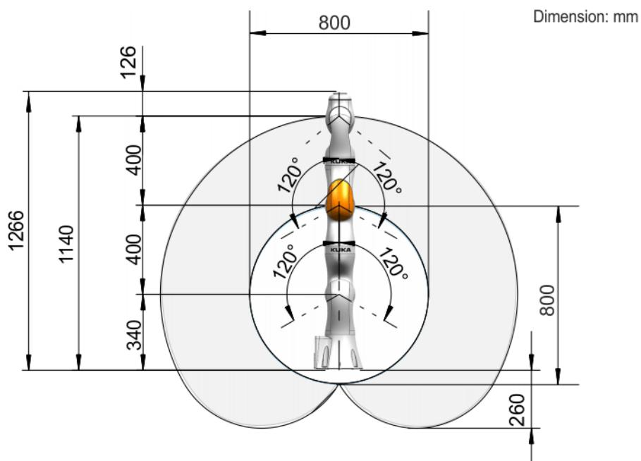
**Fig. 4-97: Working envelope, LBR iiwa 7 R800, side view**
