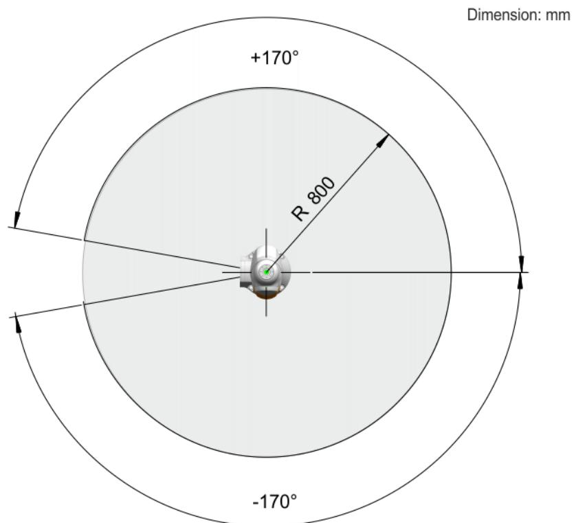
Fig. 4-68: LBR iiwa 7 R800 working envelope, top view
