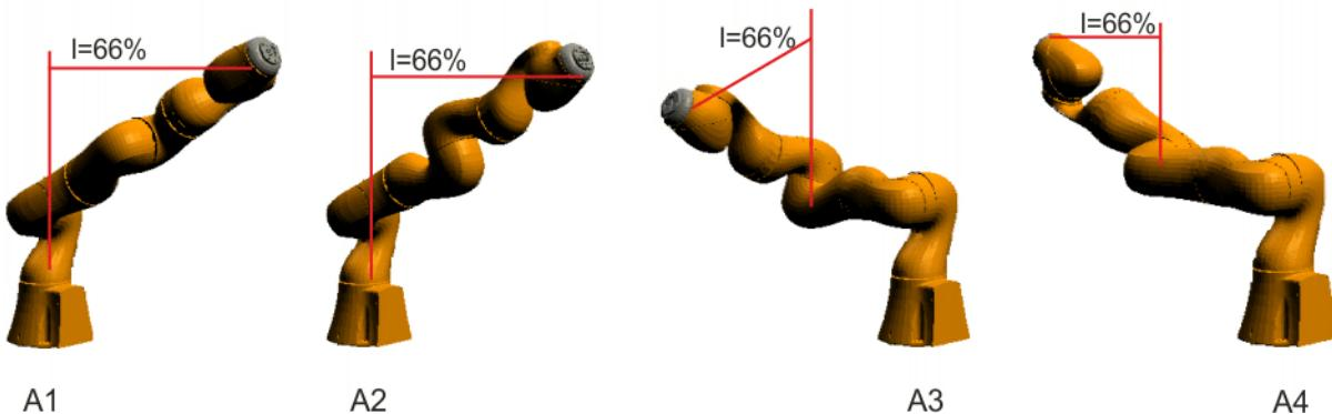
**Fig. 4-103: 66% extension, axis 1 - axis 4****Extension 100%**
