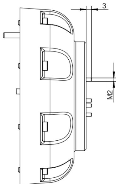
**Fig. 6-49: Dimensions, tool connector, side view**
