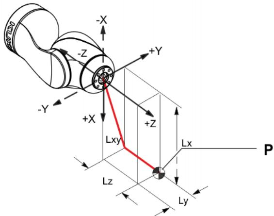
**Fig. 4-85: Load center of gravity**
