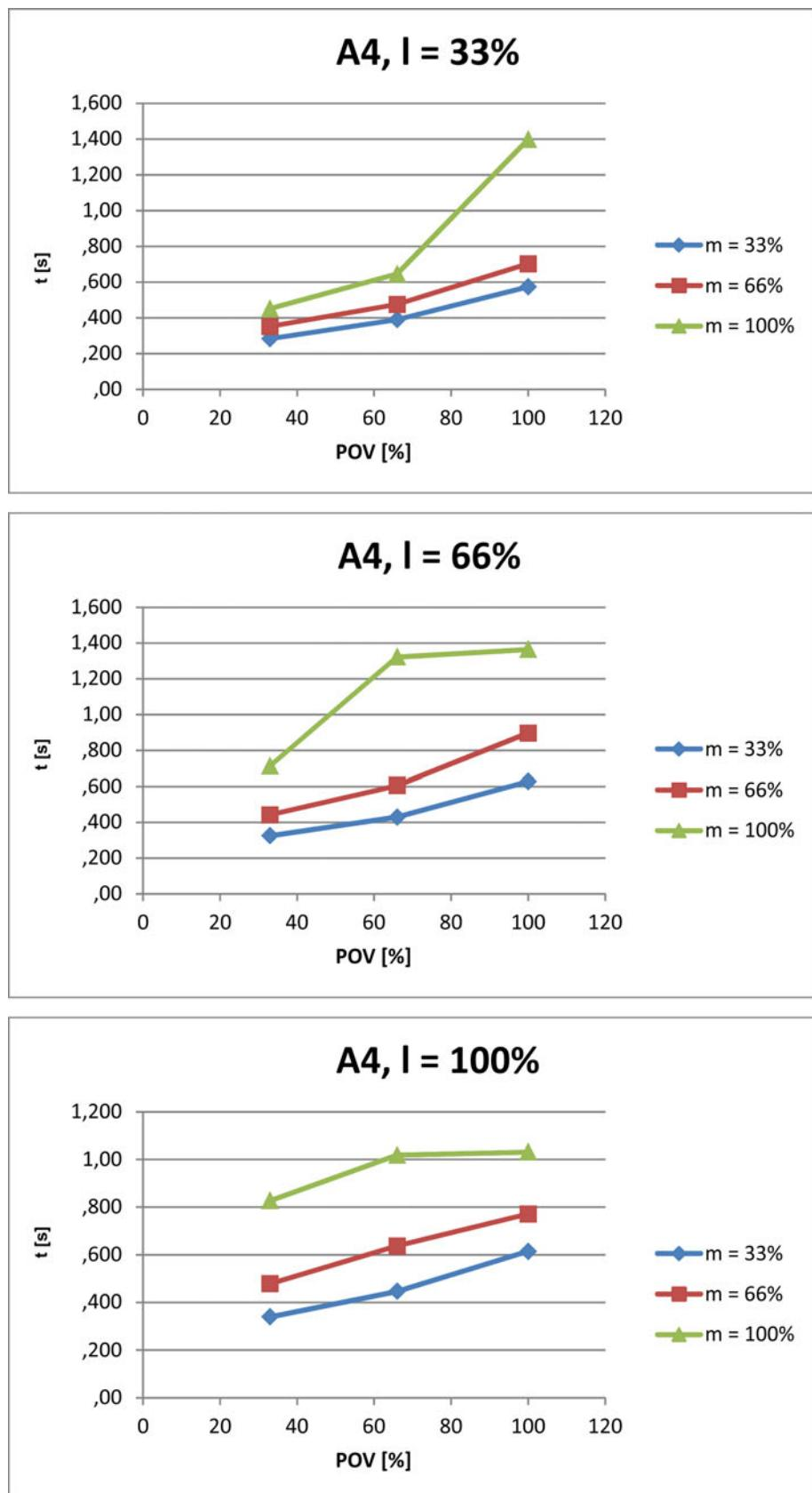
Fig. 4-128: Stopping times for STOP 1, axis 4
