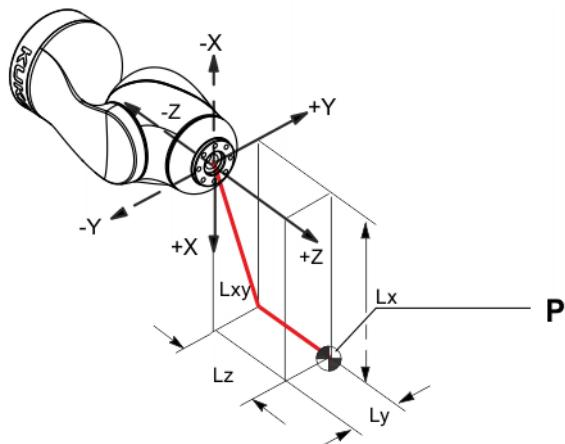
**Fig. 4-5: Load center of gravity**
