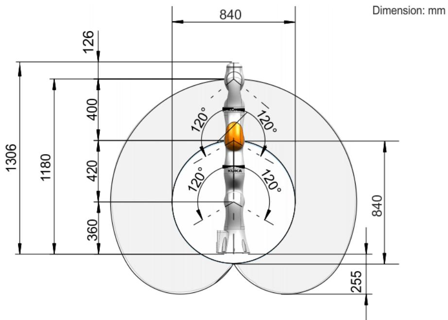
**Fig. 4-9: Working envelope, LBR iiwa 14 R820, side view**
