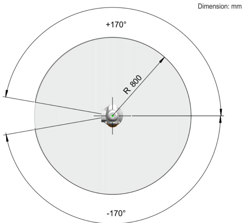
Fig. 4-100: LBR iiwa 7 R800 working envelope, top view
