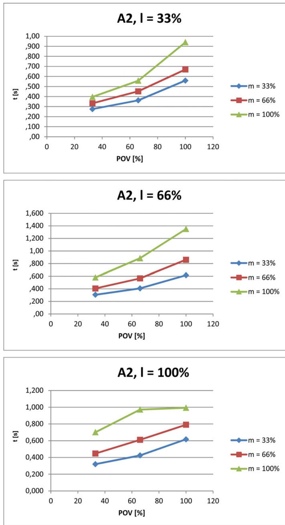
Fig. 4-132: Stopping times for STOP 1, axis 2
