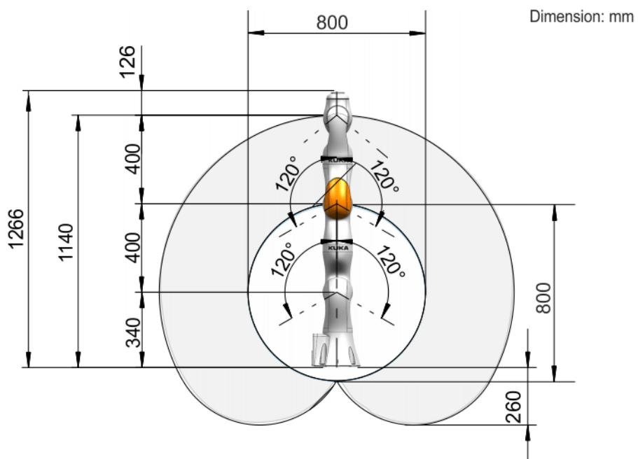
**Fig. 4-87: Working envelope, LBR iiwa 7 R800, side view**
