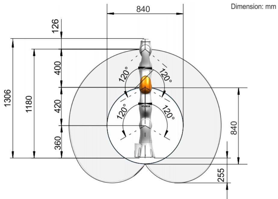
Fig. 4-89: Working envelope, LBR iiwa 14 R820, side view
