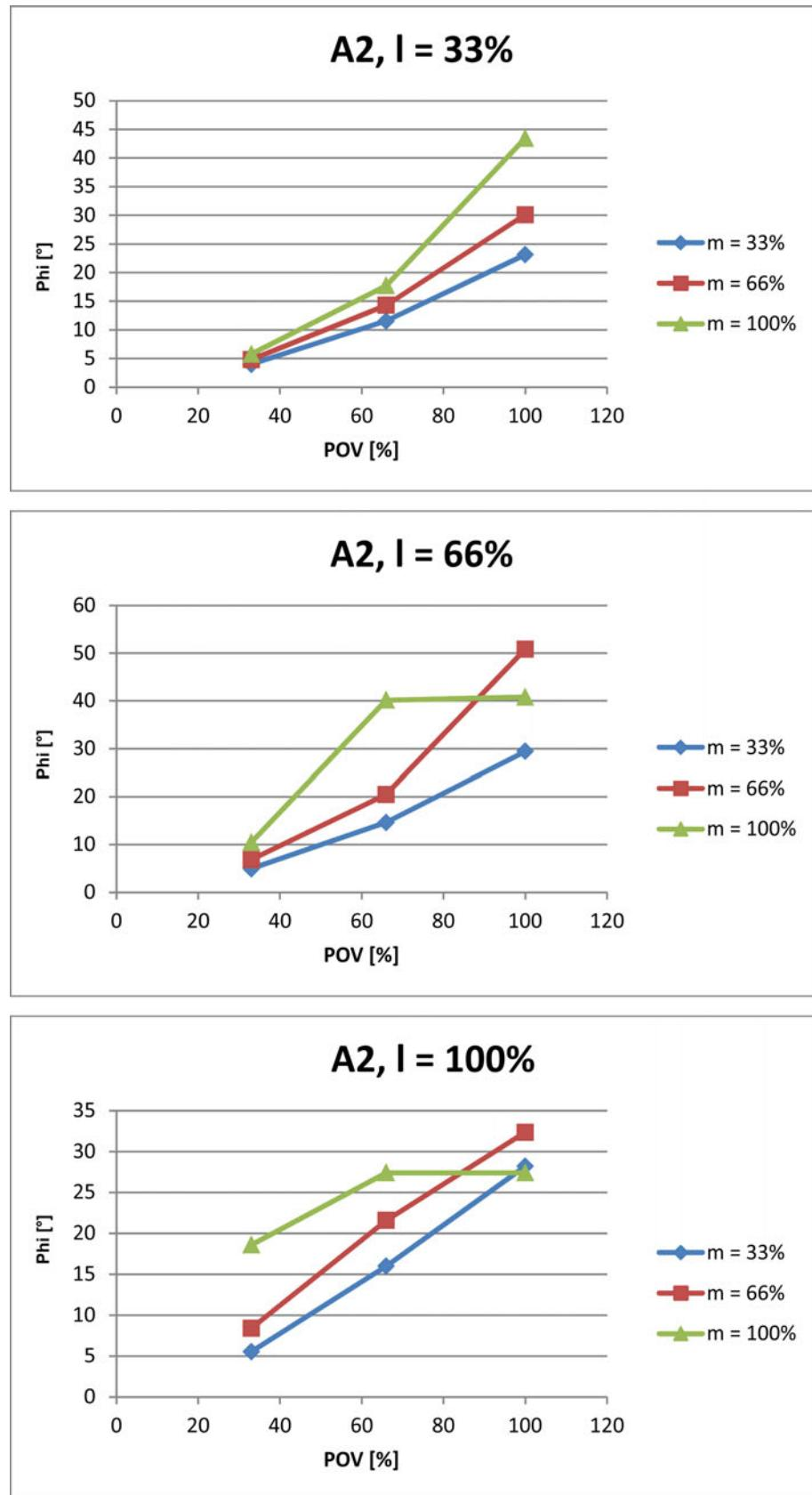
Fig. 4-123: Stopping distances for STOP 1, axis 2
