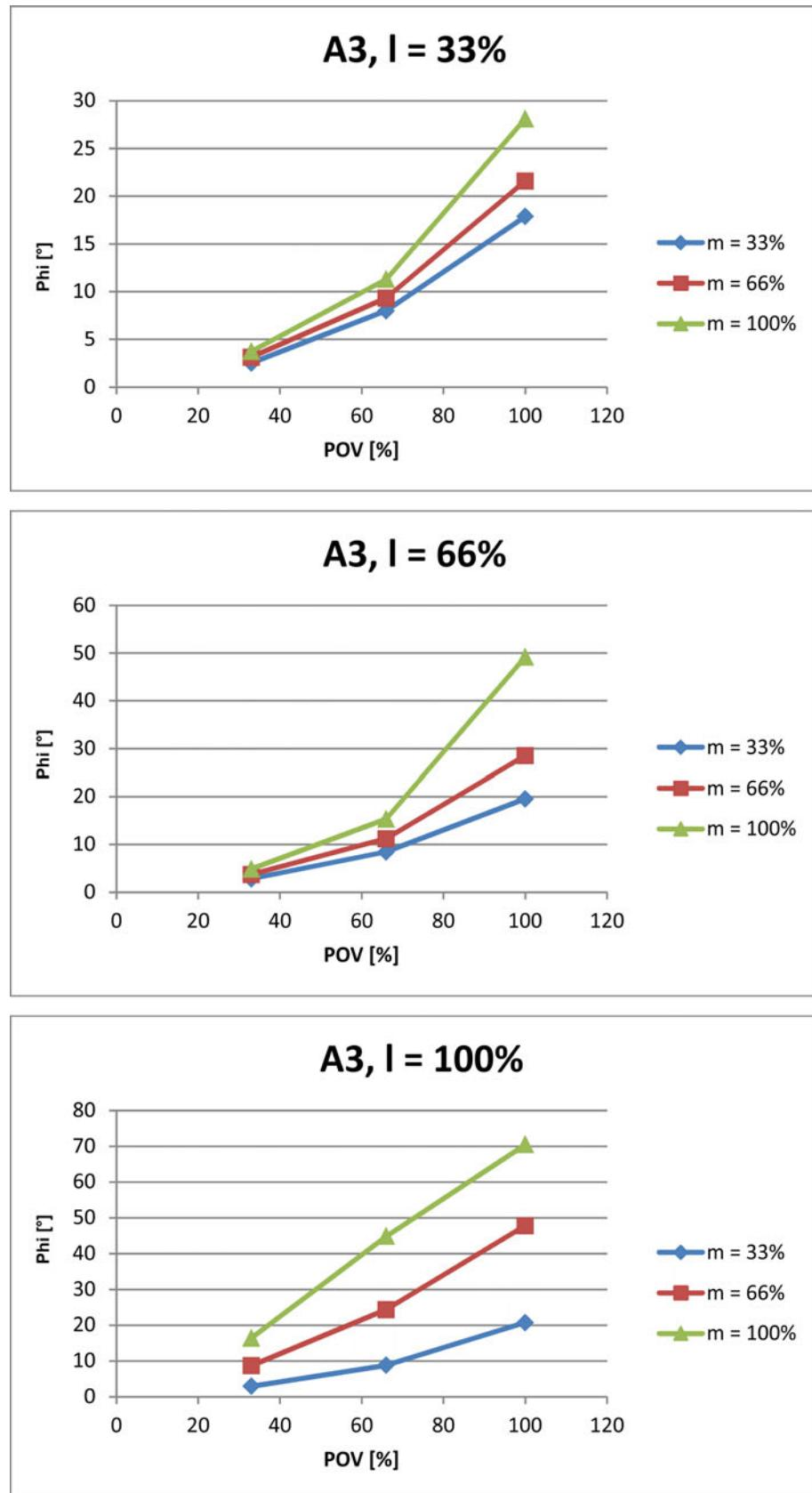
**Fig. 4-125: Stopping distances for STOP 1, axis 3**
