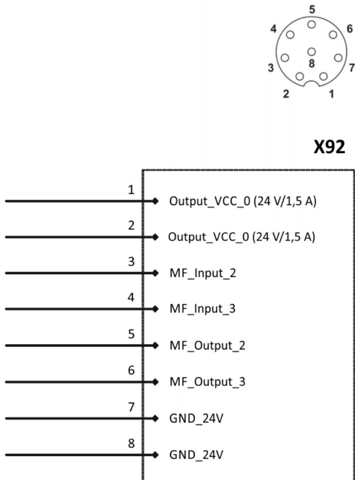
Fig. 6-34: Wiring diagram, connection X92
