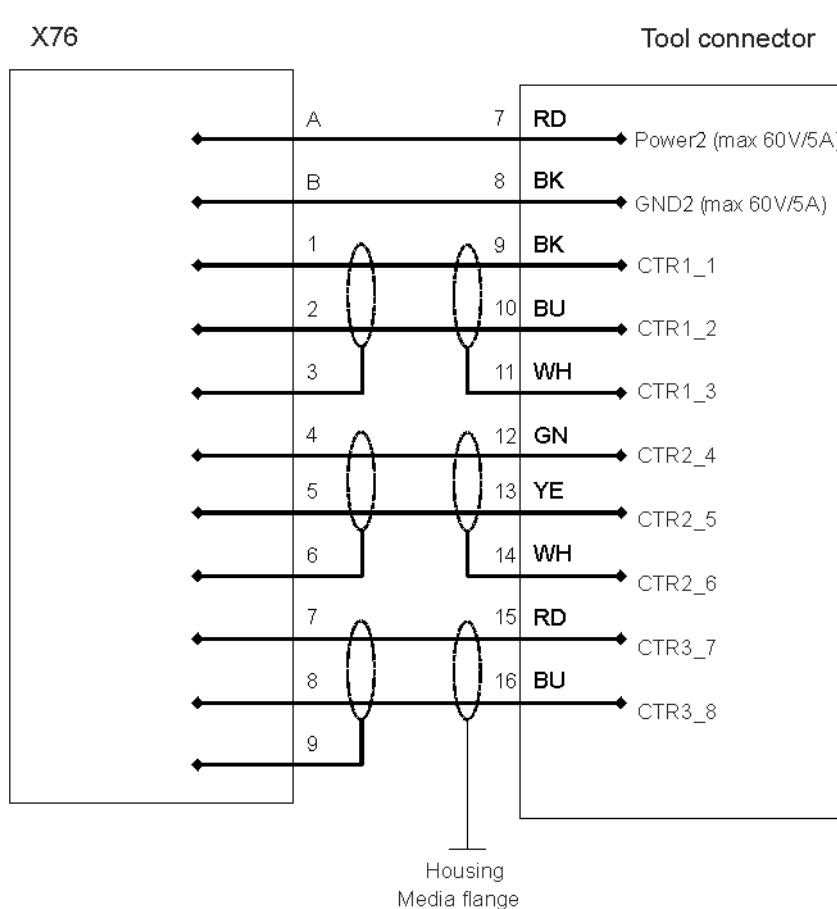
**Fig. 6-39: Wiring diagram, MF Inside electrical, X76, tool connector**
