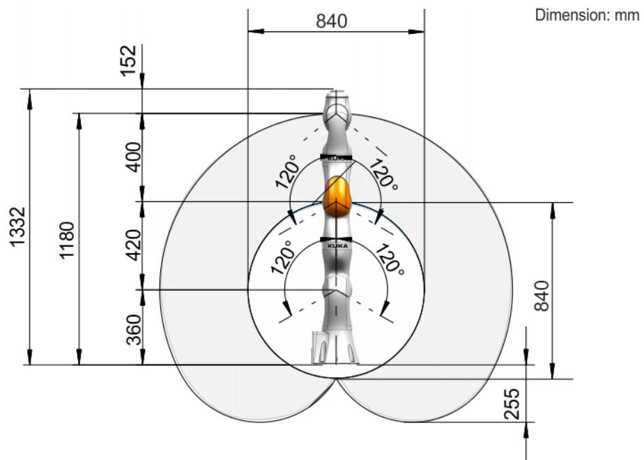
Fig. 4-79: Working envelope, LBR iiwa 14 R820, side view
