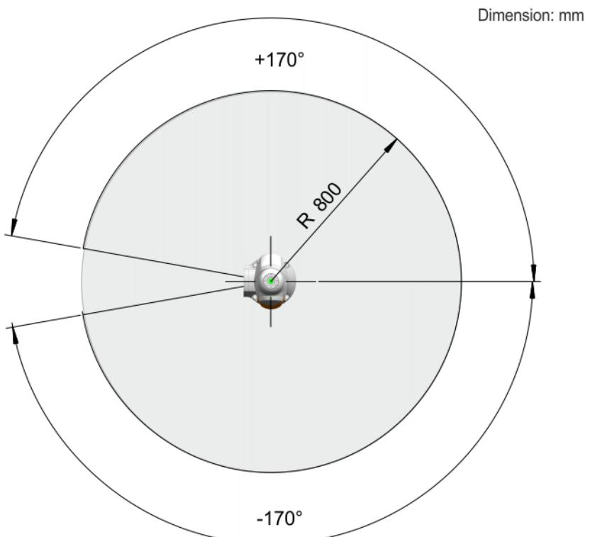
Fig. 4-18: LBR iiwa 7 R800 working envelope, top view
