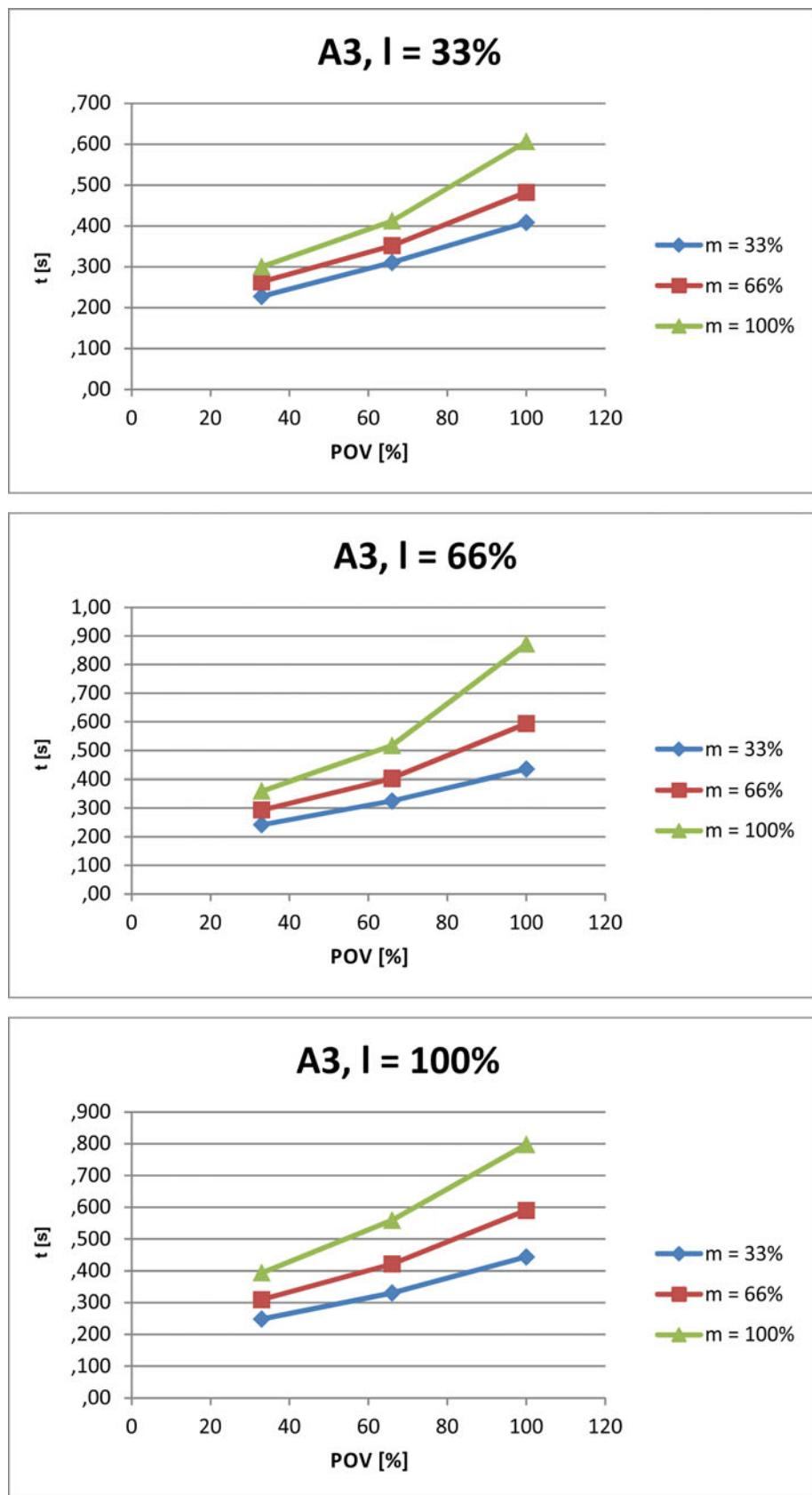
Fig. 4-110: Stopping times for STOP 1, axis 3
