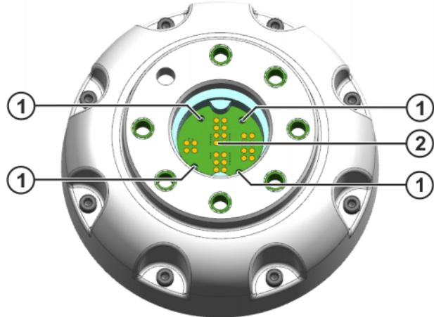
Fig. 6-37: Interface, media flange Inside electrical
