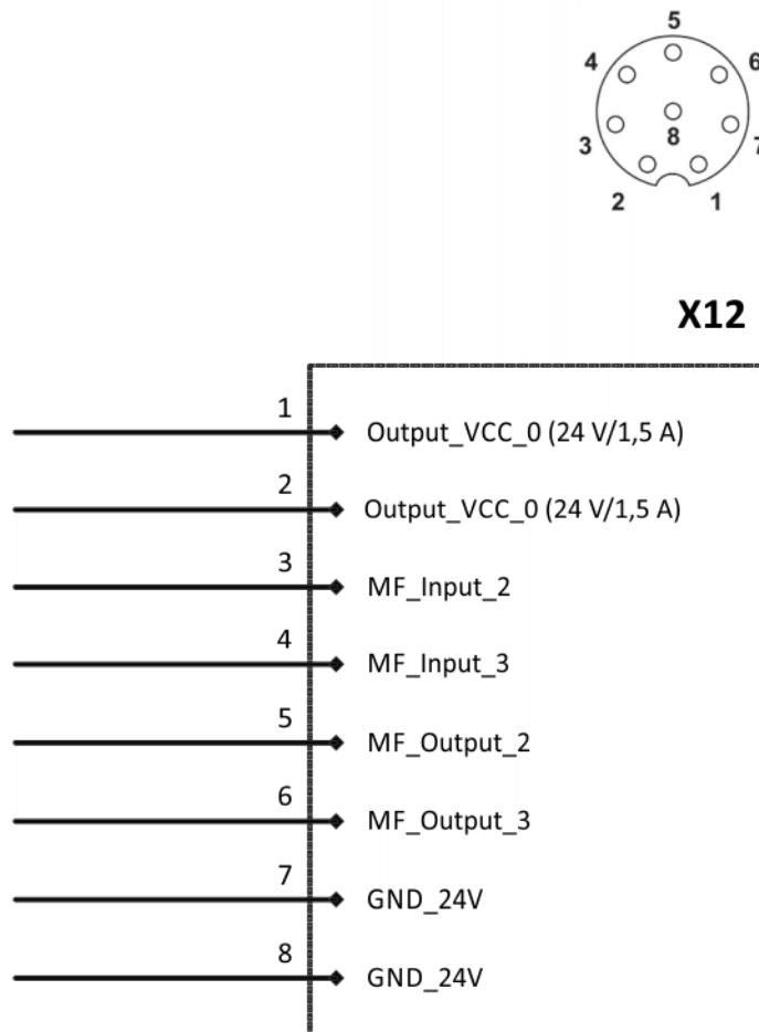
Fig. 6-13: Wiring diagram, MF IO pneumatic, X12
