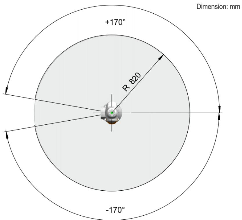
Fig. 4-80: LBR iiwa 14 R820 working envelope, top view
