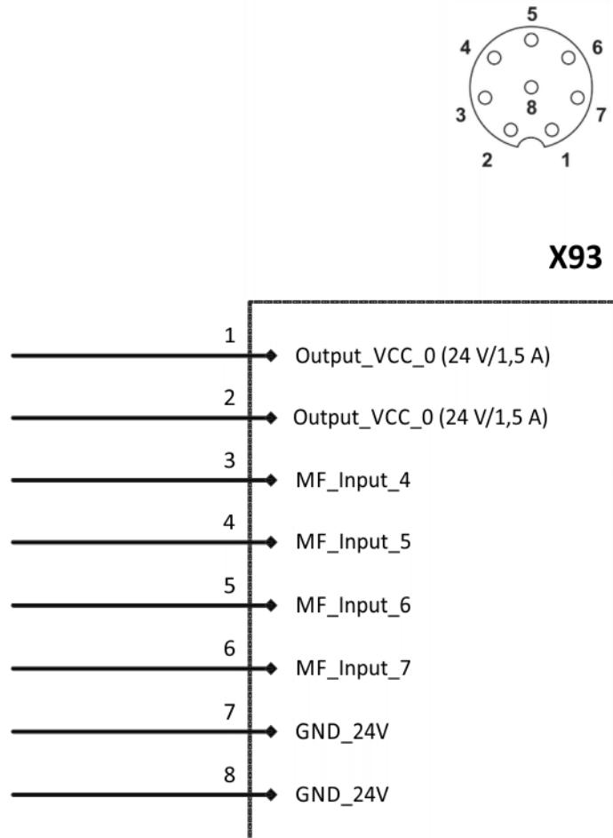
Fig. 6-35: Wiring diagram, connection X93
