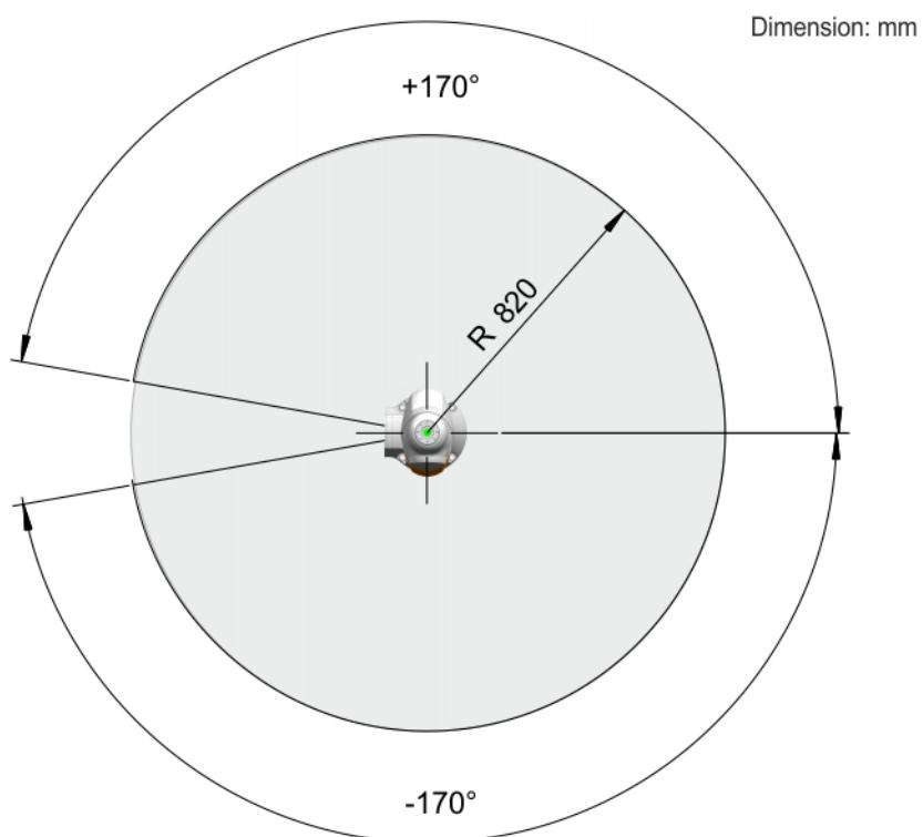
**Fig. 4-20: LBR iiwa 14 R820 working envelope, top view**
