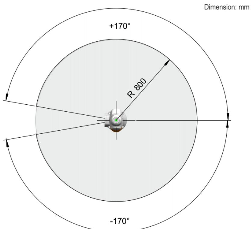
**Fig. 4-98: LBR iiwa 7 R800 working envelope, top view**
