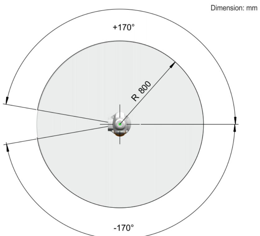
**Fig. 4-88: LBR iiwa 7 R800 working envelope, top view**
