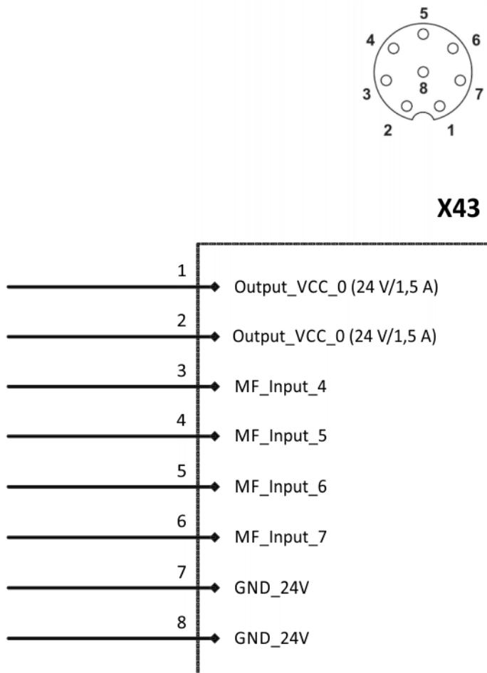
Fig. 6-27: Wiring diagram, connection X43
