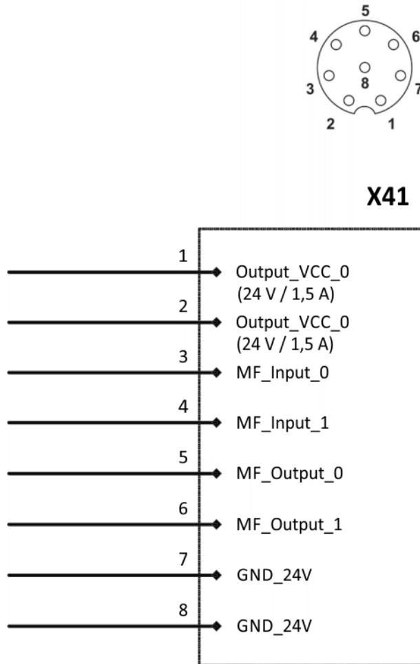
Fig. 6-25: Wiring diagram, connection X41
