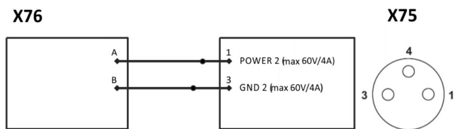
Fig. 6-22: Wiring diagram, X76, X75
