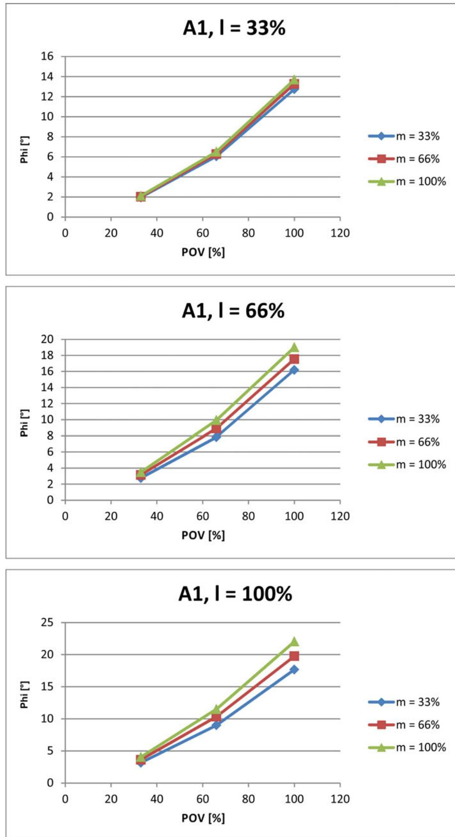
Fig. 4-105: Stopping distances for STOP 1, axis 1
