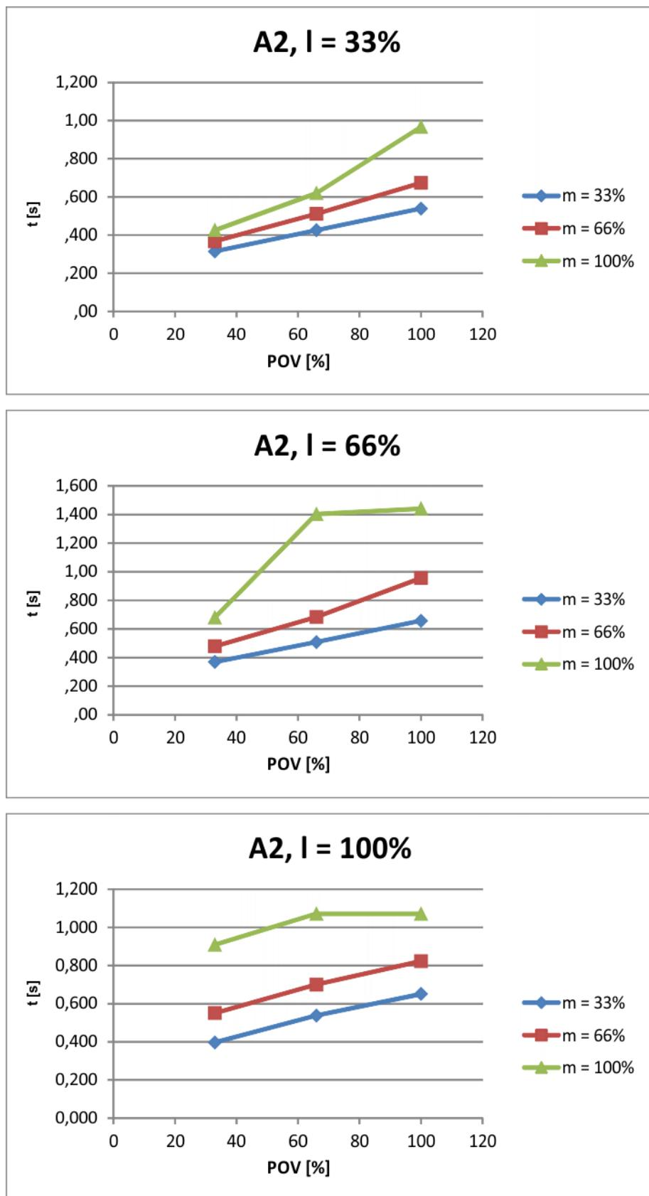
Fig. 4-108: Stopping times for STOP 1, axis 2
