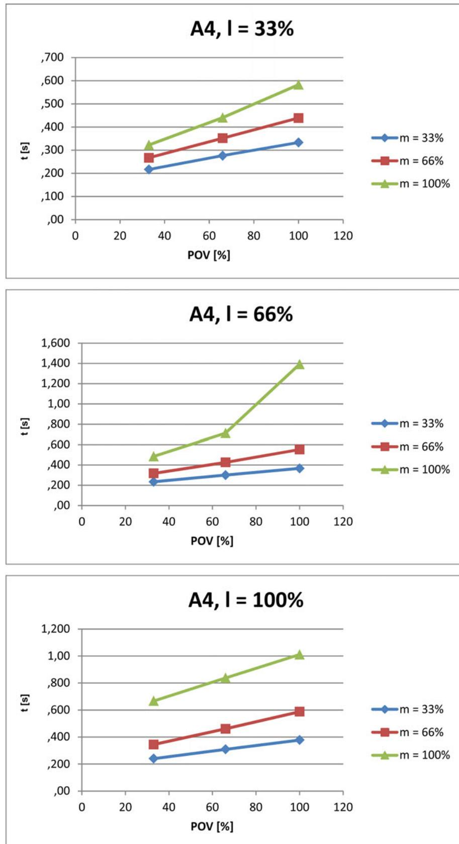
Fig. 4-120: Stopping times for STOP 1, axis 4
