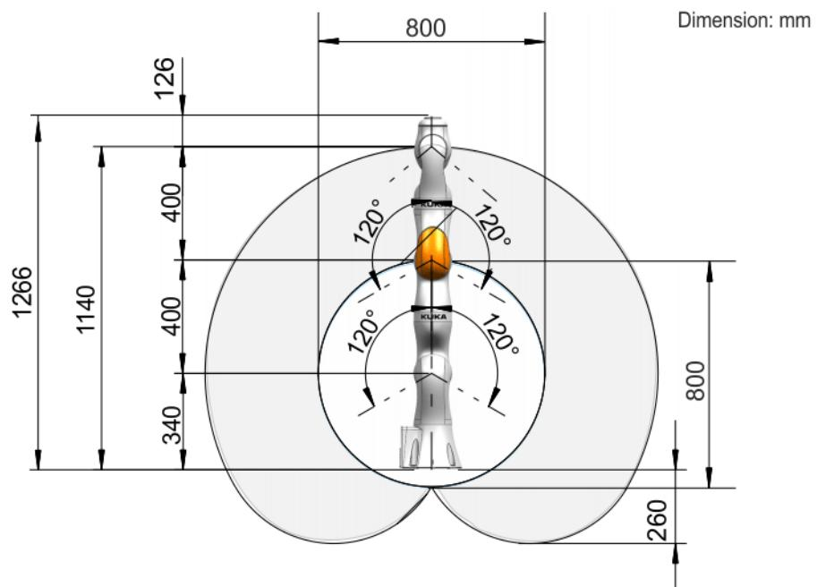
Fig. 4-67: Working envelope, LBR iiwa 7 R800, side view
