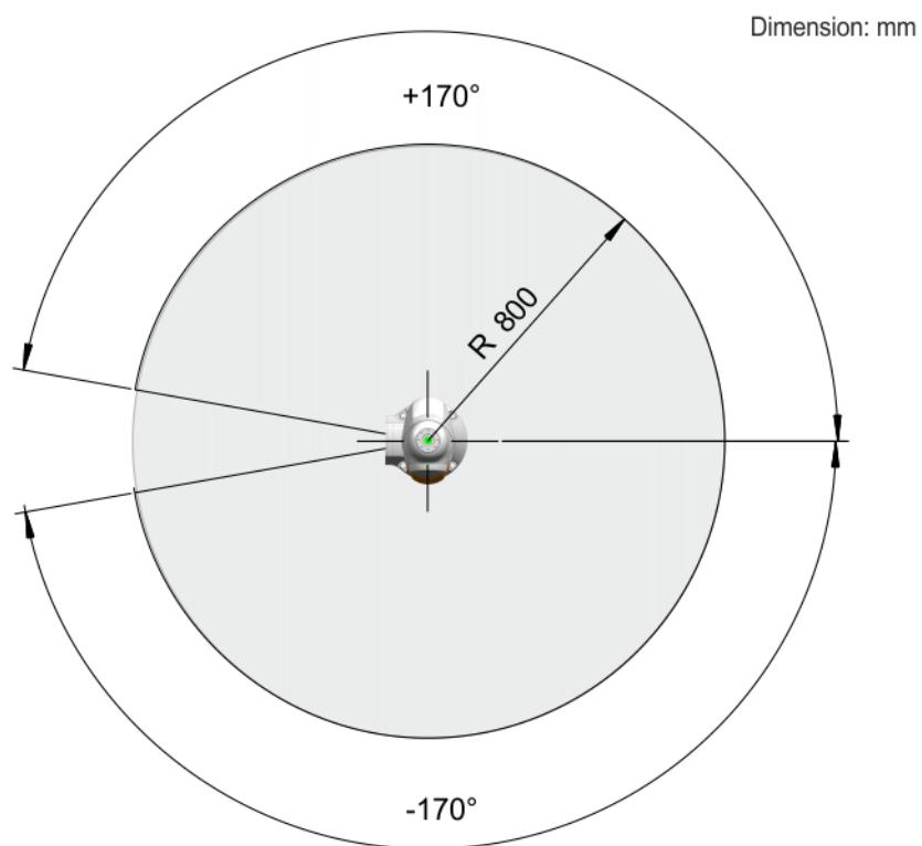
**Fig. 4-78: LBR iiwa 7 R800 working envelope, top view**
