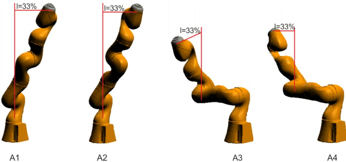
Fig. 4-102: Extension 33%, axis 1 - axis 4
