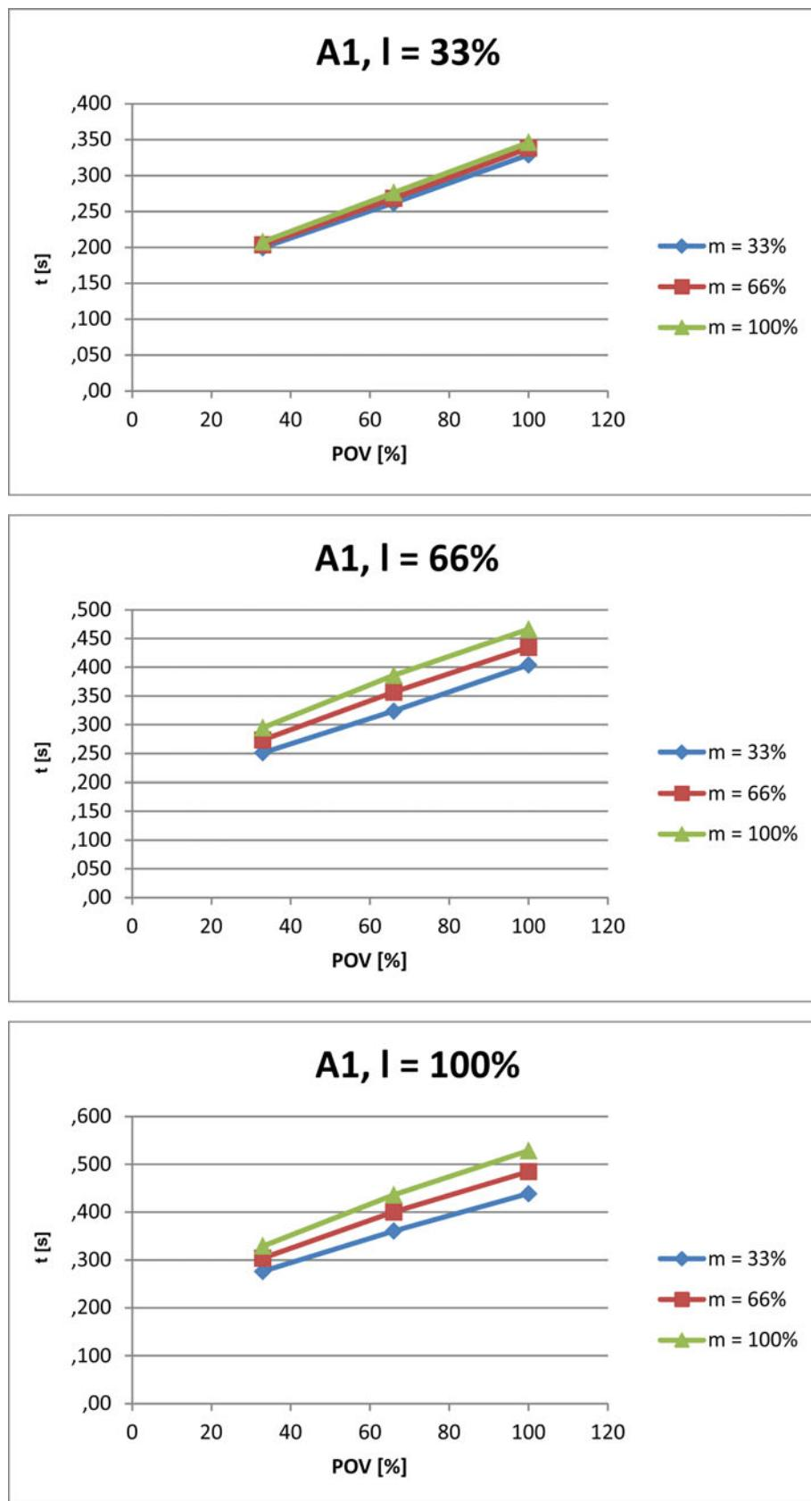
Fig. 4-122: Stopping times for STOP 1, axis 1
