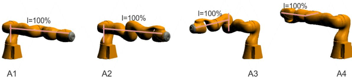
**Fig. 4-104: Extension 100%, axis 1 - axis 4****4.12.3 Stopping distances and stopping times for LBR iiwa 7 R800**
