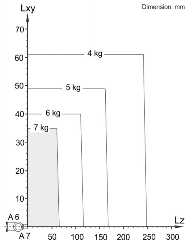
Fig. 4-74: Payload diagram, LBR iiwa 7 R800
