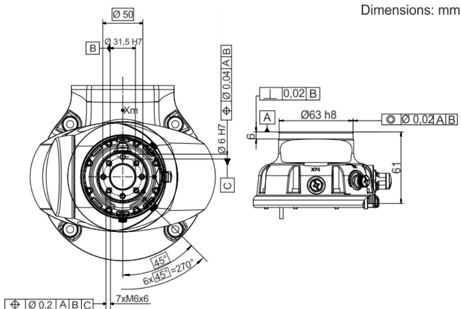
**Fig. 4-51: Dimensions, media flange Touch electrical**
