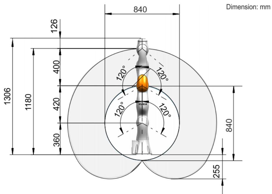
Fig. 4-69: Working envelope, LBR iiwa 14 R820, side view
