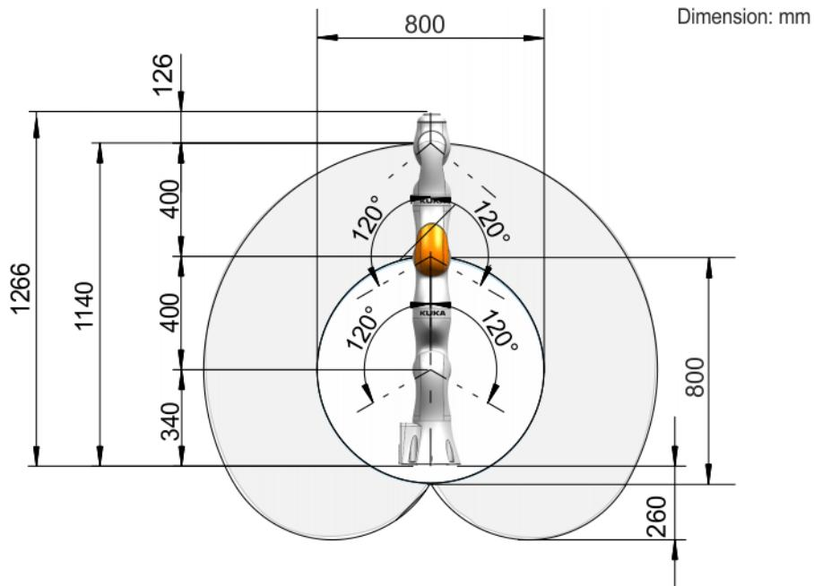
Fig. 4-17: Working envelope, LBR iiwa 7 R800, side view
