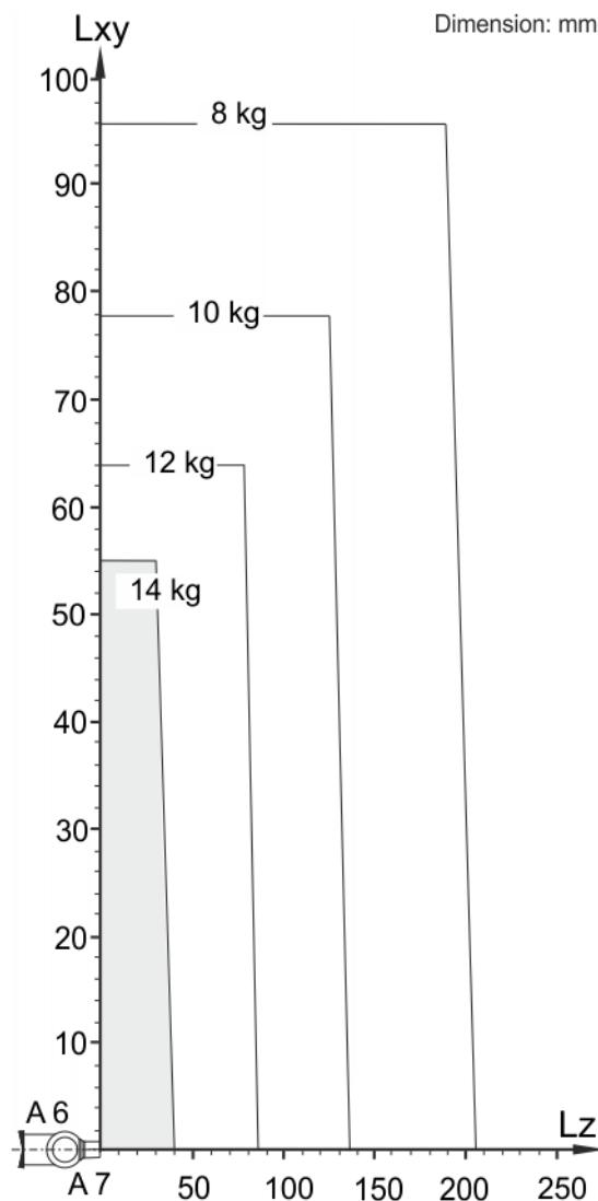
Fig. 4-76: Payload diagram, LBR iiwa 14 R820
