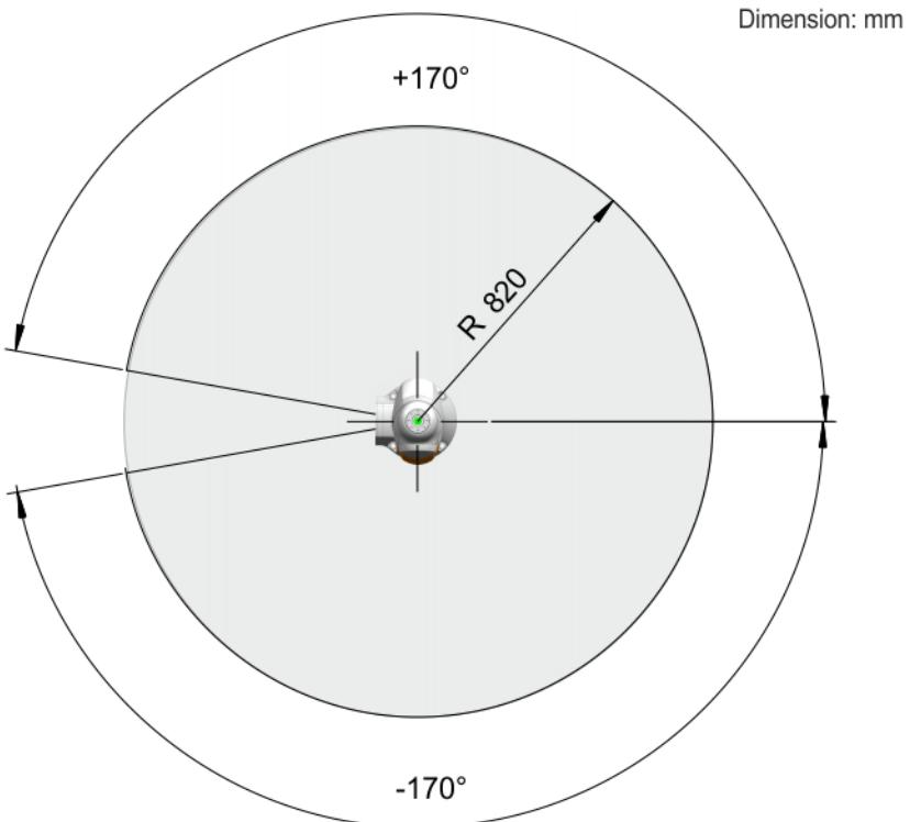
Fig. 4-60: LBR iiwa 14 R820 working envelope, top view
