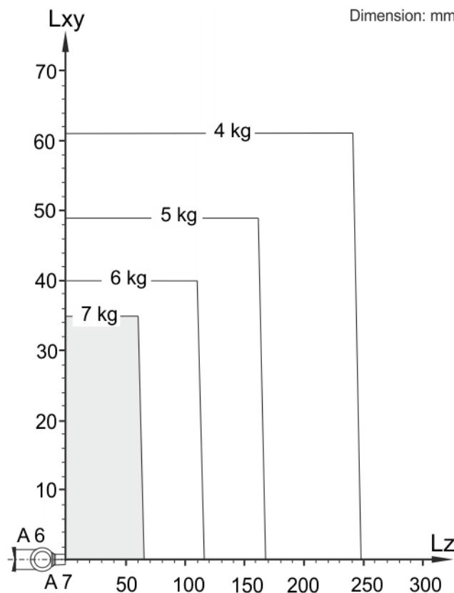
Fig. 4-44: Payload diagram, LBR iiwa 7 R800
