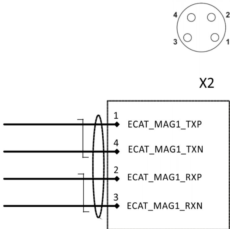
Fig. 6-18: Wiring diagram, connection X2
