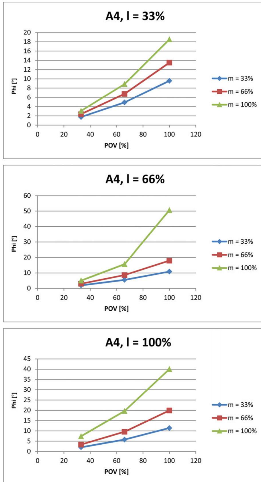
Fig. 4-119: Stopping distances for STOP 1, axis 4
