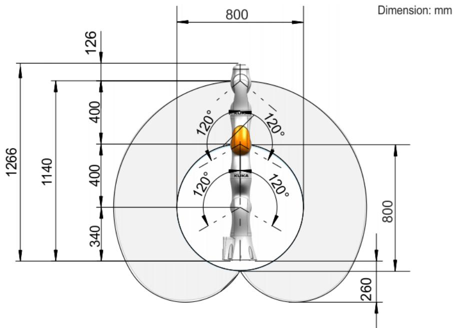
Fig. 4-27: Working envelope, LBR iiwa 7 R800, side view
