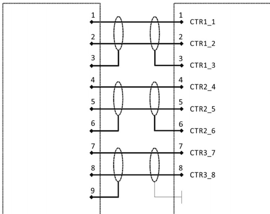
**Fig. 6-23: Wiring diagram, connection X76, X74**
