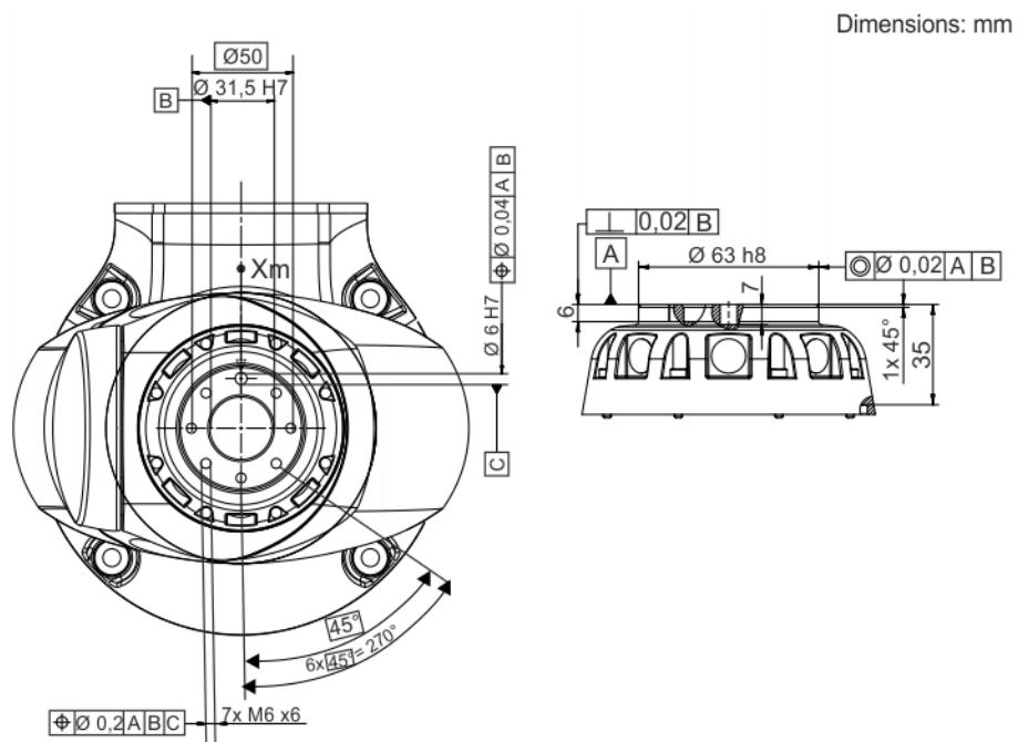
**Fig. 4-1: Dimensions, basic flange**
