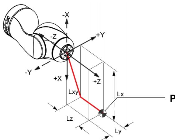
**Fig. 4-43: Load center of gravity**
