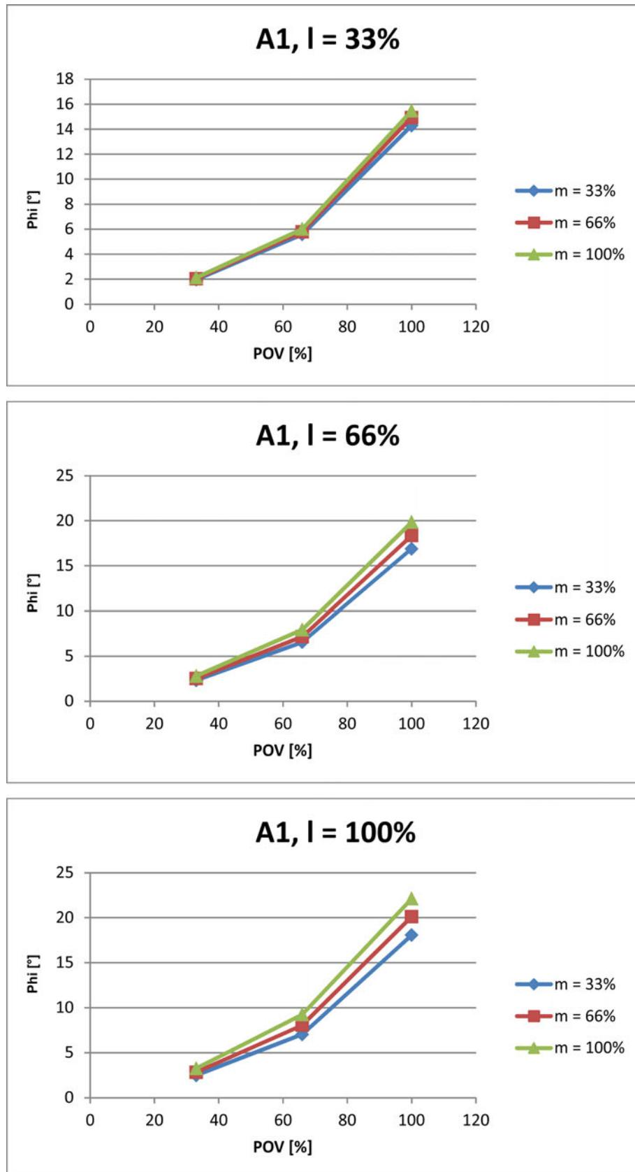
**Fig. 4-113: Stopping distances for STOP 1, axis 1**
