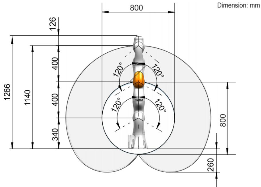
Fig. 4-37: Working envelope, LBR iiwa 7 R800, side view
