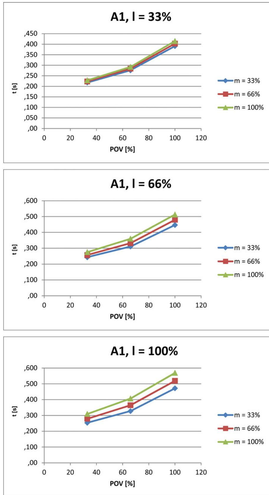
Fig. 4-114: Stopping times for STOP 1, axis 1
