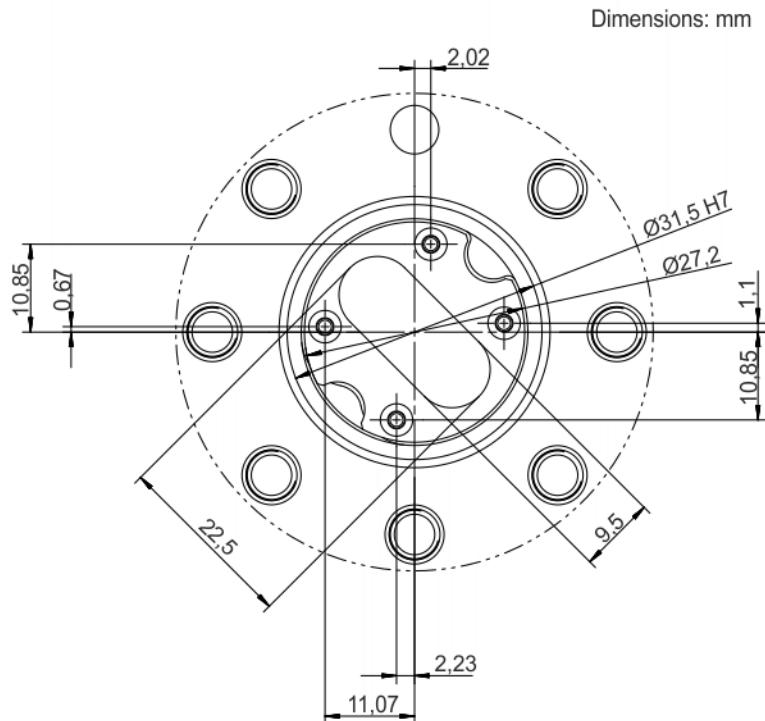
**Fig. 6-45: Dimensions, tool connector, top view**
