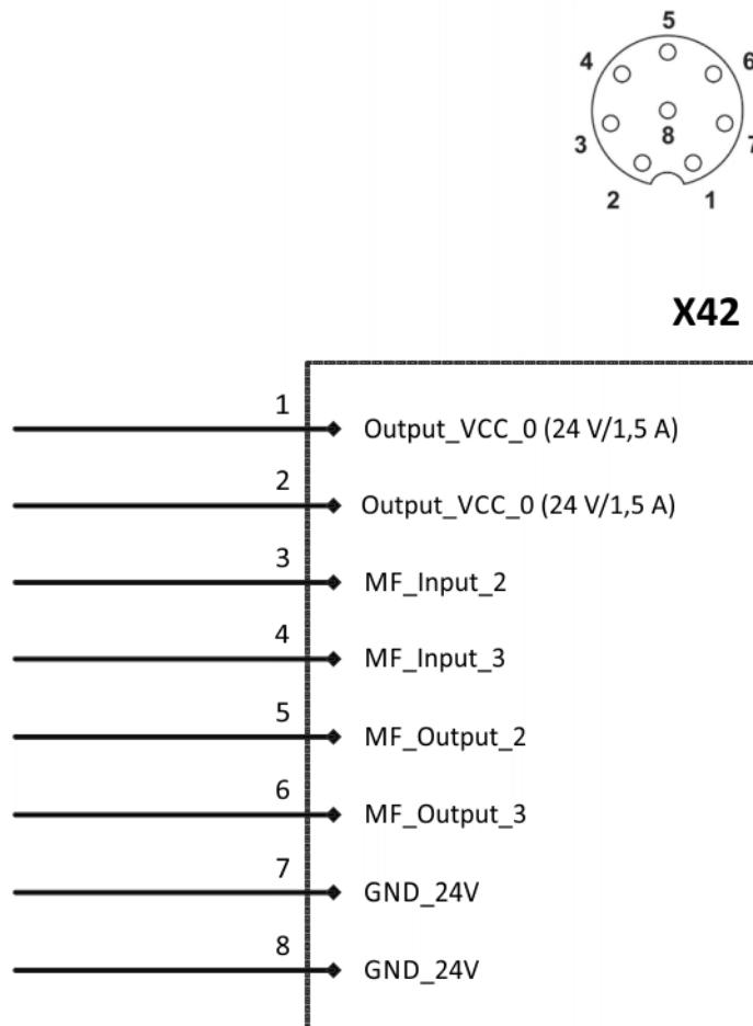
**Fig. 6-26: Wiring diagram, connection X42**
