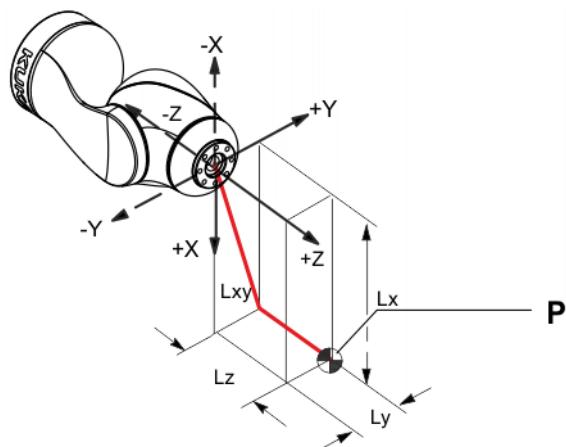
**Fig. 4-65: Load center of gravity**
