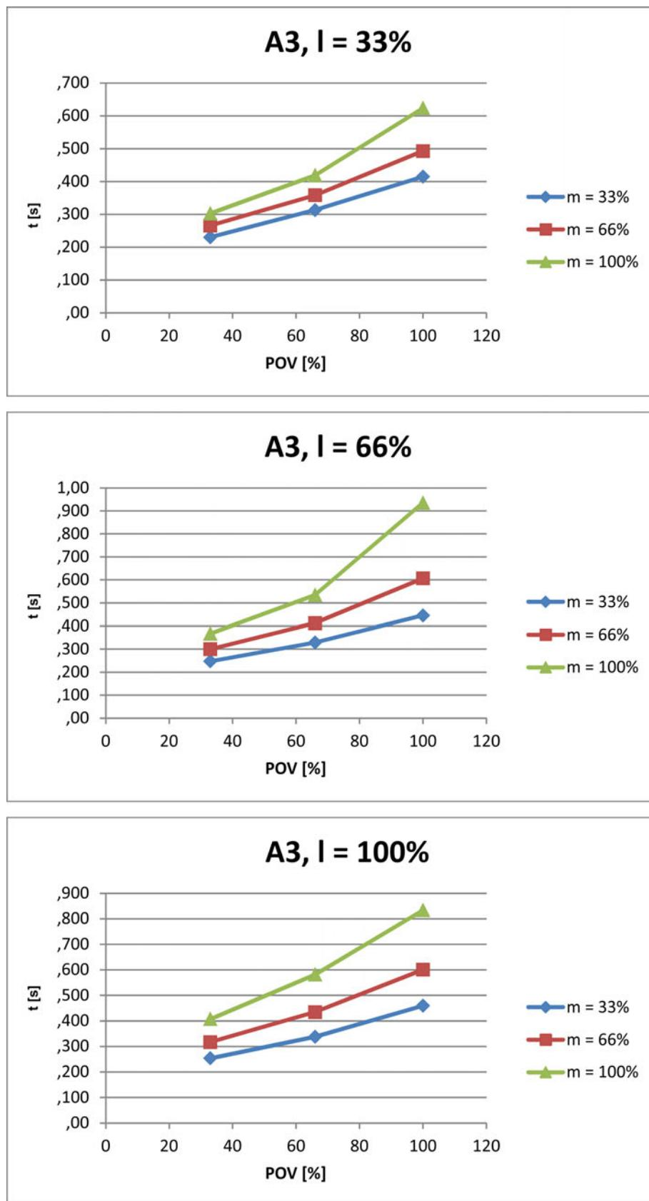
Fig. 4-126: Stopping times for STOP 1, axis 3
