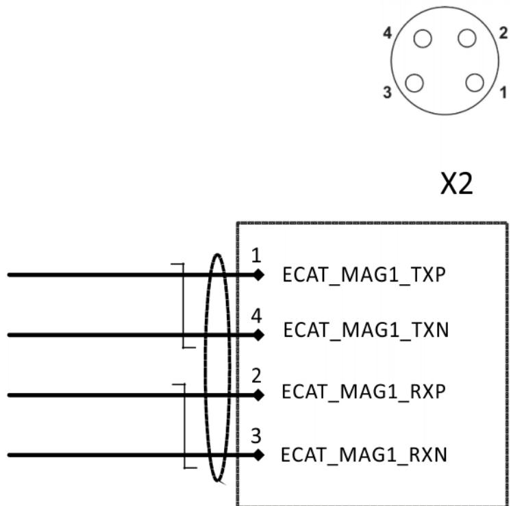
Fig. 6-21: Wiring diagram, connection X2
