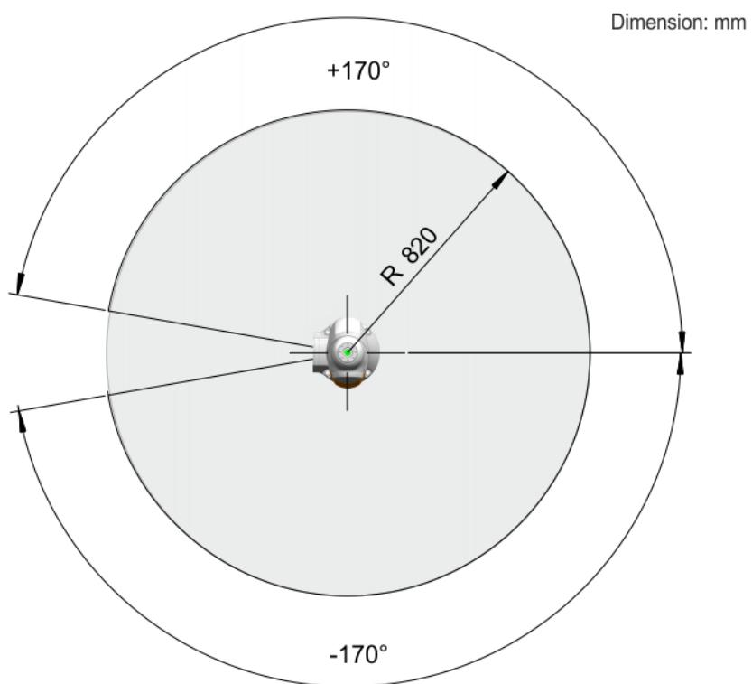
Fig. 4-90: LBR iiwa 14 R820 working envelope, top view
