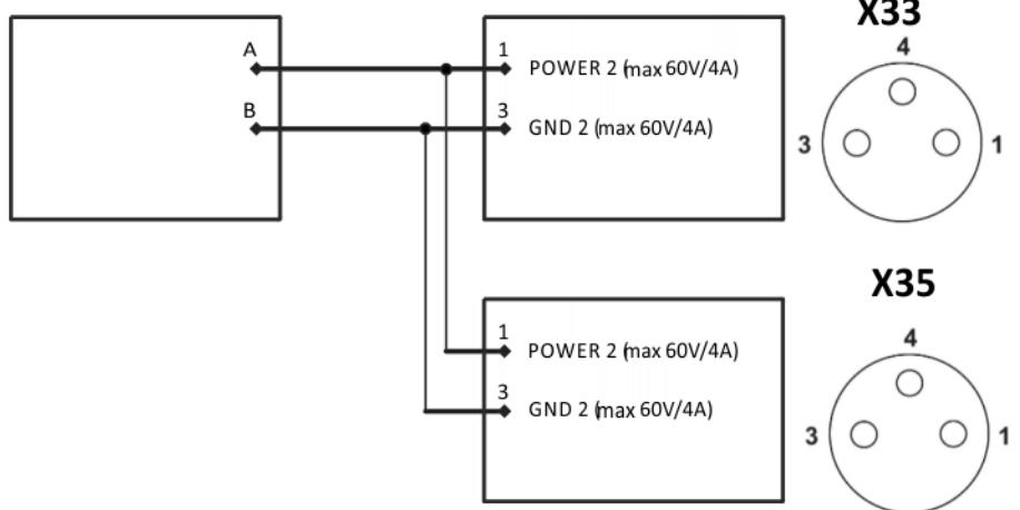
Fig. 6-6: Wiring diagram, MF electrical, X76, X33, X35
