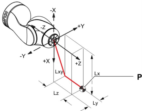
**Fig. 4-35: Load center of gravity**
