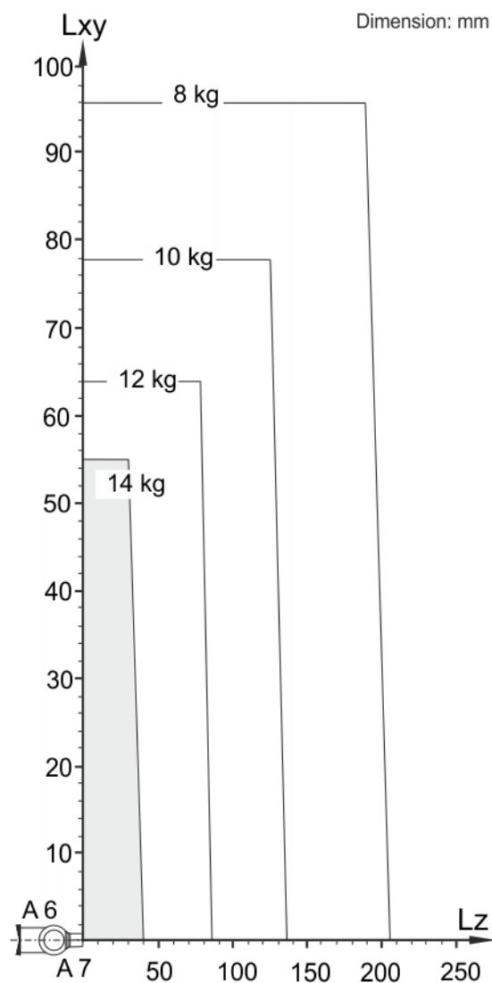
**Fig. 4-46: Payload diagram, LBR iiwa 14 R820**
