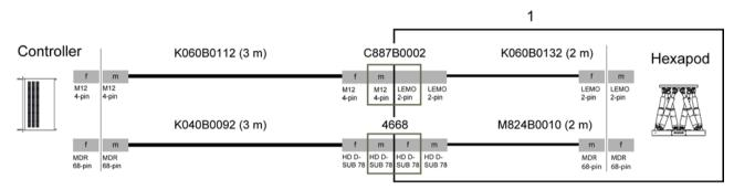
Figure 11: Connection diagram for C-887. V02 standard cable set for vacuum versions
