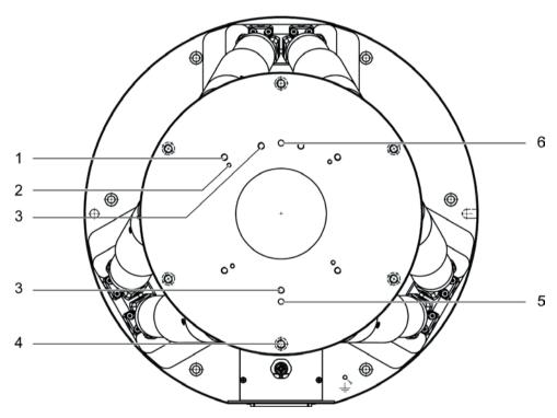
Figure 9: Mounting and locating holes in the moving platform
