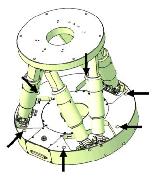
Figure 8: Mounting holes in the base plate
