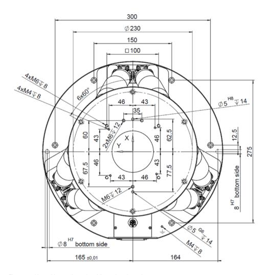
Figure 16: H-850 Hexapod top view (dimensions in mm)
