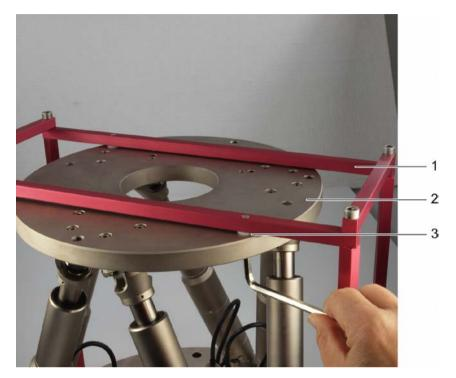
Figure 13: Transport lock on the moving platform
