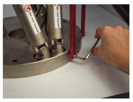
Figure 14: Transport lock on the base plate
