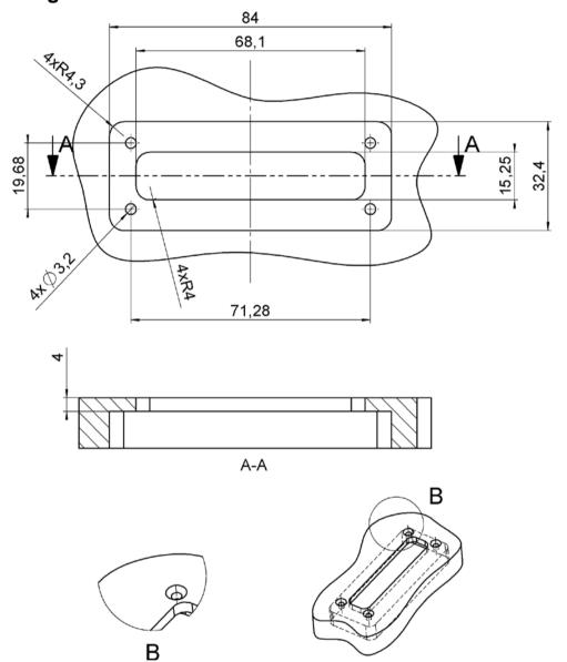
Figure 10: Dimensions of the vacuum feedthrough for data transmission (4668) (dimensions in mm)
