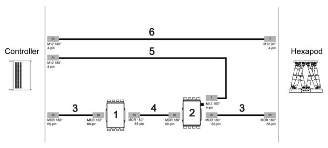
Figure 12: Connection diagram of cable set with line driver boxes
