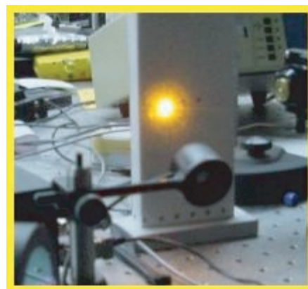
Figure 3. First-light result from system integration test. The 589-nm laser light was generated by sum-frequency mixing the 1583-nm and 938-nm fiber lasers in PPLN.
