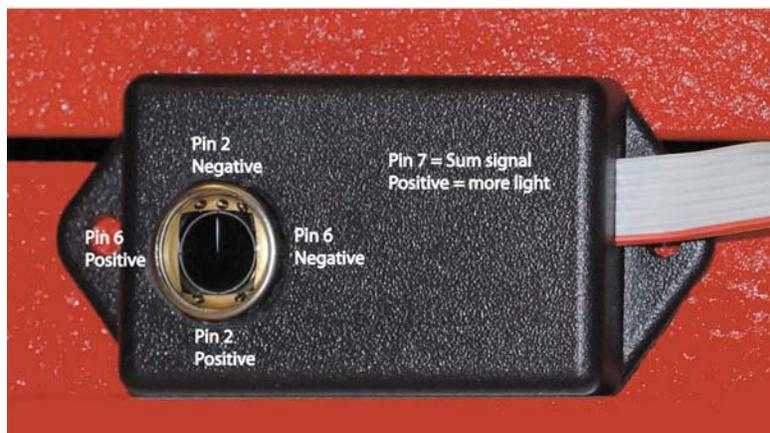
Figure 6. Quad Cell Orientation and Polarity
