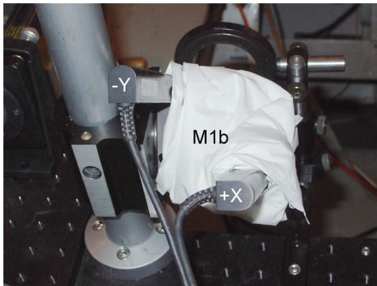
Figure 2. M1b Actuators
