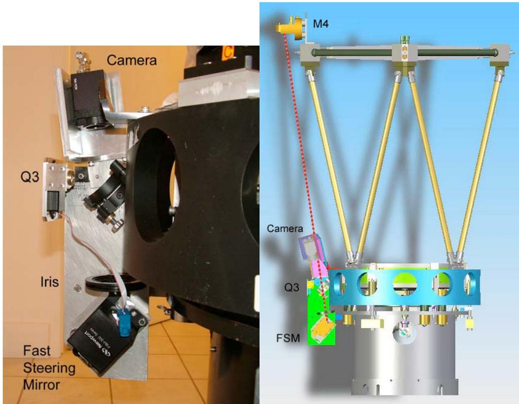
Figure 5. Laser Launch Telescope, with M4, Q3, FSM.
