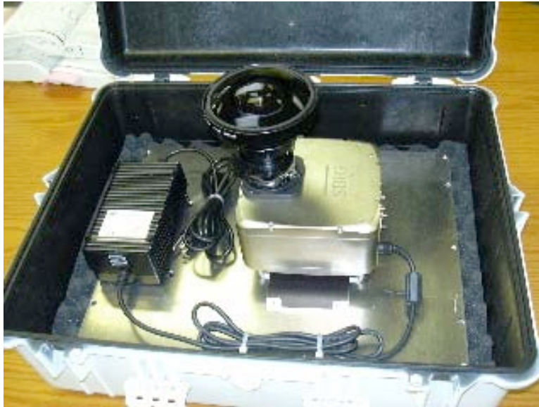
Figure 2: The All Sky Camera in its weather-proof case.
