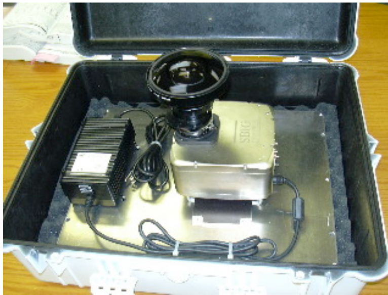
Figure 2: The All Sky Camera in its weather-proof case.
