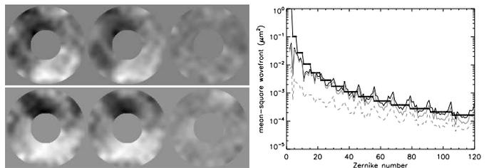
Figure 5: Left: two sample analysis frames, with the FSM loop closed on the HOWFS. Left pupils: wavefronts reconstructed from HOWFS ("truth" wavefront). Center pupils: wavefronts estimated from MGSU. Right pupils: residual wavefronts. Right: mean-square wavefront error per Zernike coefficient (pluses: Kolmogorov theory; solid: HOWFS estimate; dashed: residual error).
