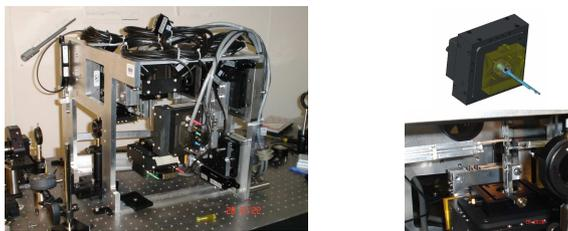
Figure 2: Left: MGSU as built: 4 WFSs mounted on X/Y translation stages. Right: 3D rendering of pick-off arm (top); closeup of three arms in position in the MGSU (bottom).
