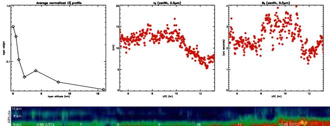
Figure 3: MASS/DIMM data for 10-11 Feb 2006 MGSU data collection run. Left: average normalized  $C_n^2$  profile. Center and right: time evolution of  $r_0$  and  $\theta_0$ . Bottom: evolution of  $C_n^2$  (logarithmic altitude scale).
