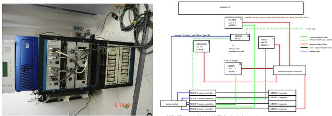
Figure 1: Left: MGSU electronics rack, 8-channel motion controller, test PC, camera controller, NPS, 4 1U Dell PCs, 3.2 TB of data storage on 2 RAID disks. Right: control schematics diagram.
