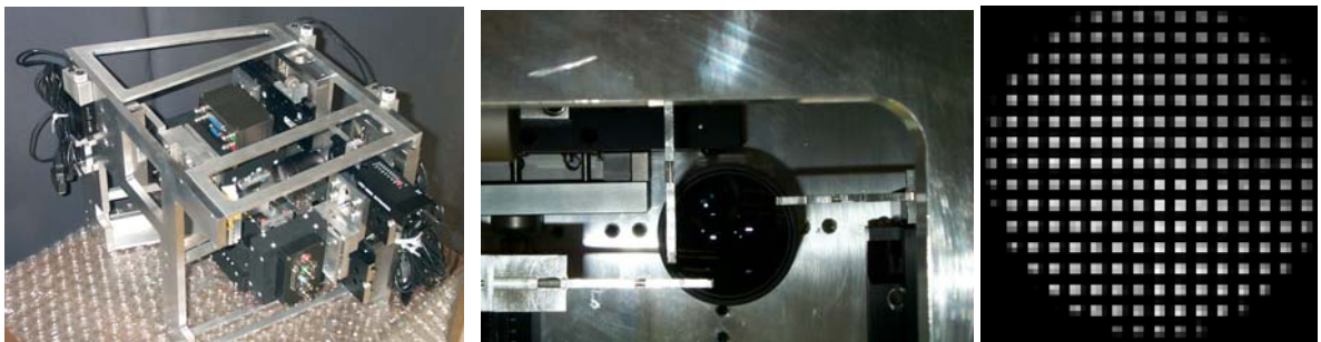
Figure 2. Tomograph hardware ( Left ) of the four channel tomographic wavefront sensor funded under AST-0096928. Four fast-frame, low-noise CCD cameras (each mounted on its own x-y positioning stages) are arranged symmetrically around a patrol field of 90 arcsec diameter. Optics on small (1.5mm) pick-off arms ( Center ) form 16x16 subaperture Shack-Hartmann images ( Right ).
