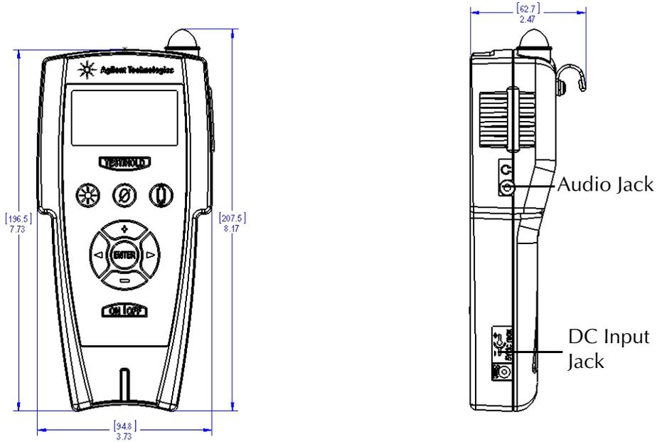
**Figure 1-1 Wireless Remote Dimensions, Connections and Controls**
