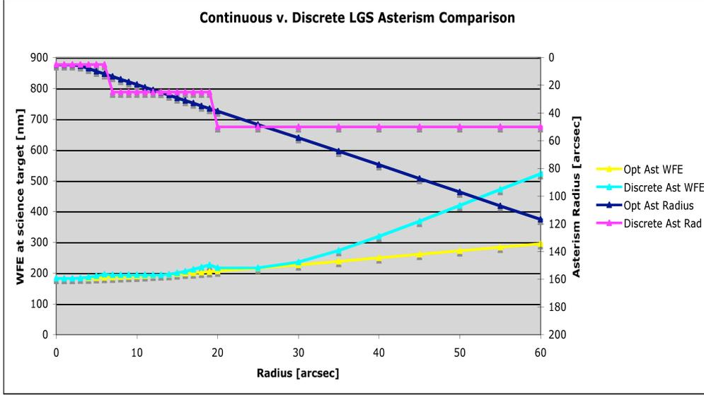
Figure 4: Wide field MOAO case where the science target is off-axis, with a brightest TT star of  $m_v=17$  are assumed to be within the field of 30 arcsec (corresponds to 10% sky coverage).
