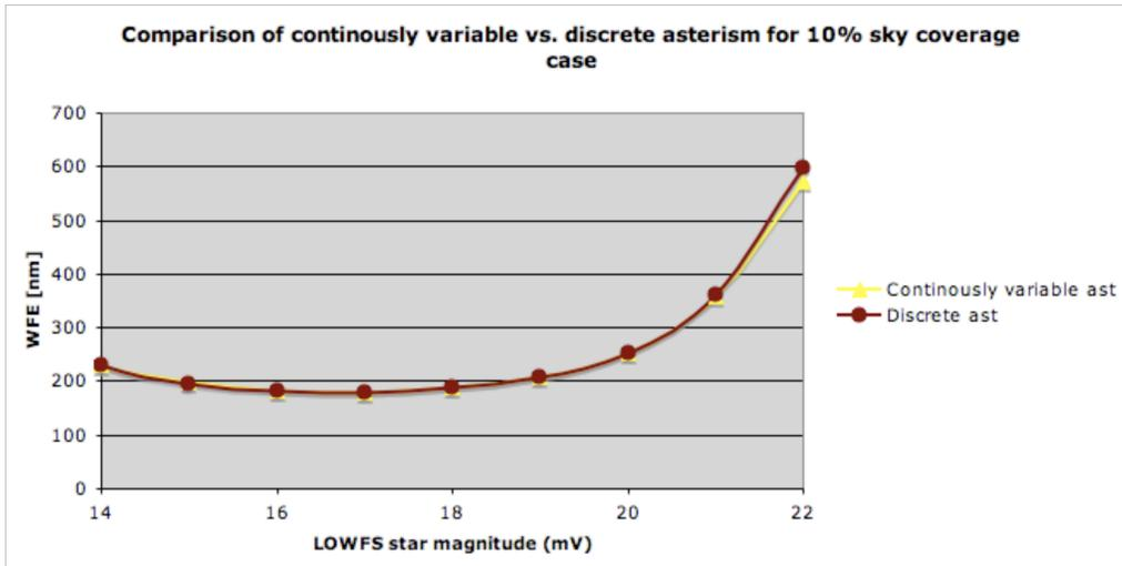
Figure 1: Wavefront error vs. TT star magnitude plot for 10% sky coverage case
