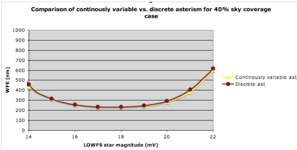
Figure 2: Wavefront error vs. TT star magnitude plot for 40% sky coverage case
