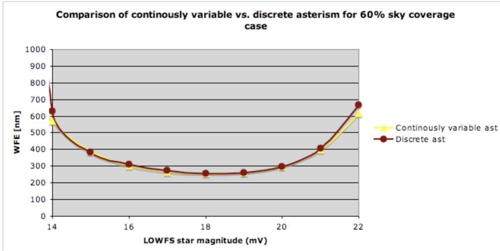
Figure 3: Wavefront error vs. TT star magnitude plot for 60% sky coverage case
