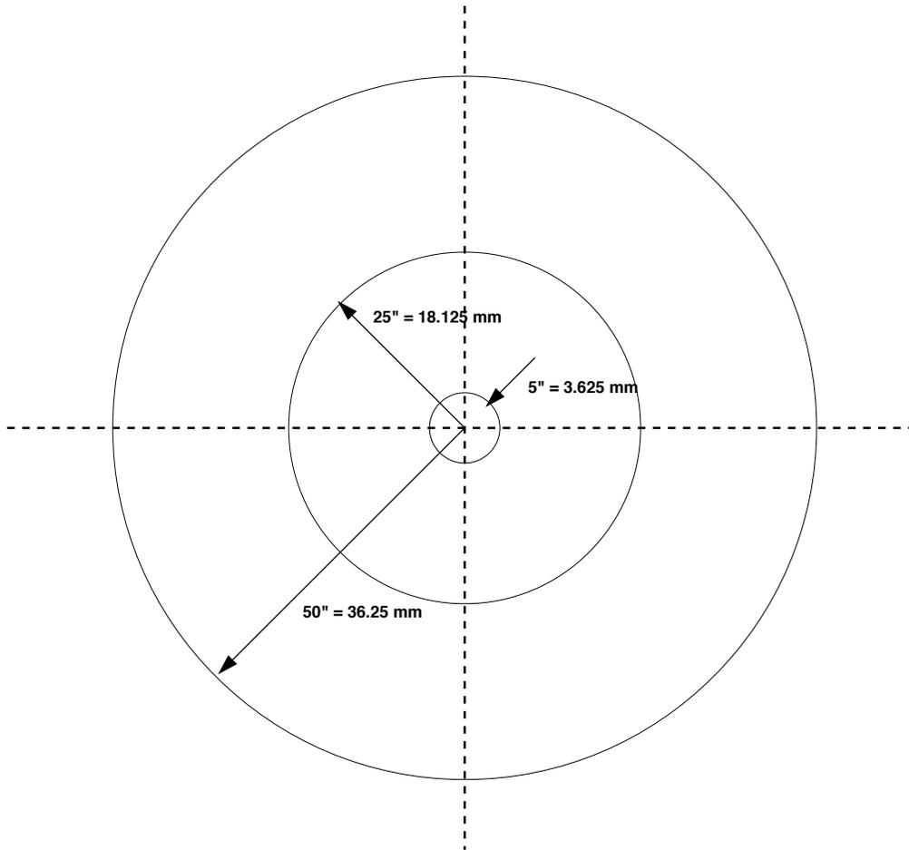
Figure 7: Schematic showing the asterism radii for 5, 25 and 50 arcsec at the focal plane.
