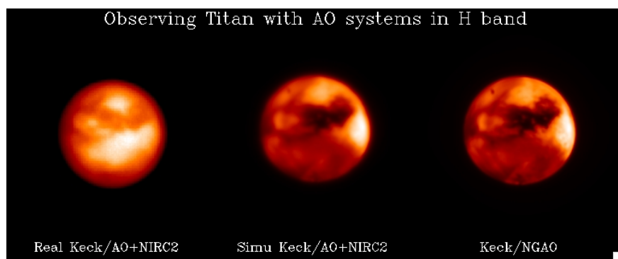
Figure 10 Validation of simulation with observations along with examples of expected NGAO performance. The Keck simulation is based on a 0.9 μm map generated through Cassini observations. Simulated image and observations may be slightly different because variation the color of surface feature, for instance the bright southern pole is rather dark on our simulation. The angular diameter of Titan is 0.8".
