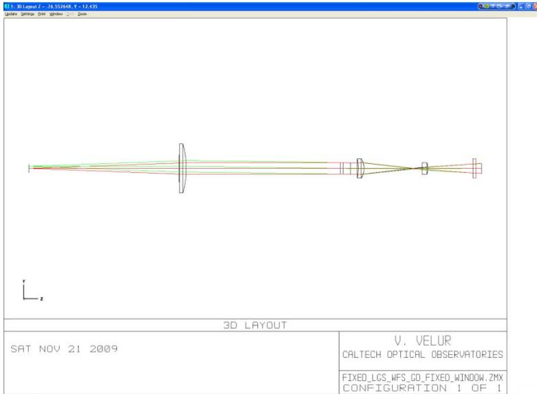
Figure 17 - layout of fixed LGSWFS, The total length of the sensor is 230 mm. The relay is composed of a best-form lens for a collimator, a custom lenslet array and a set of custom singlet relay lenses.
