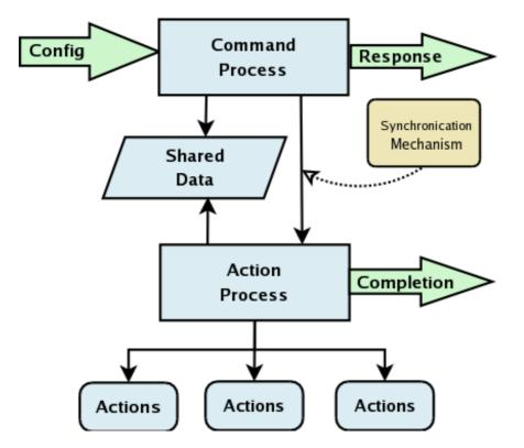
ATST Controllers use threads to implement both command and action processing.
