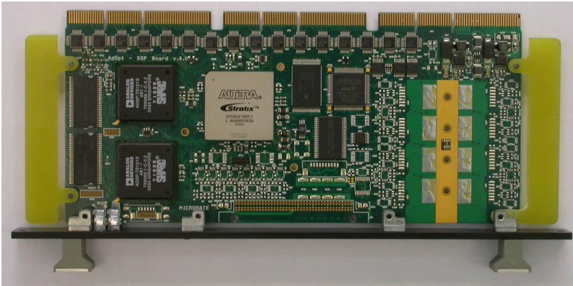
Figure 10 – DSP board V3.0. The board in this picture is completely mounted, including the analog parts used only on the HVC board.
