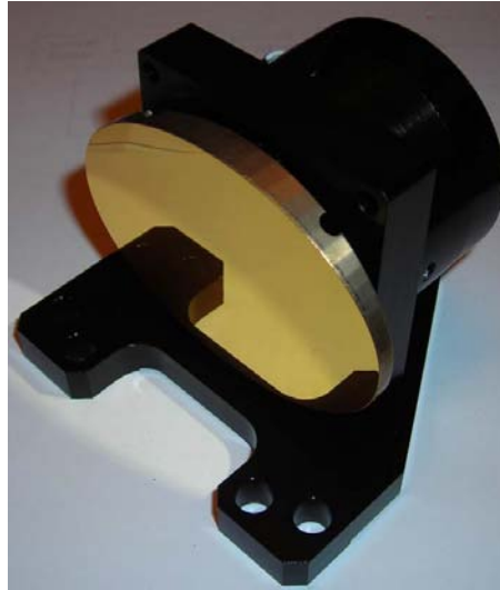
Figure 43: OIM102.3 elliptical fast steering mirror
