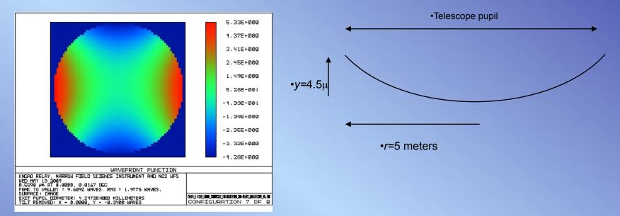
•The wavefront error on the extreme field points of the LGS WFS is dominated by astigmatism. •Use the slope of the wavefront to determine the maximum spot displacement on the wavefront sensor:  $125 \text{ m}^2 = 145 \text{ m}^{10^{-6}} \text{ m} = 25 \text{ m}^2 \text{ m}^2$
