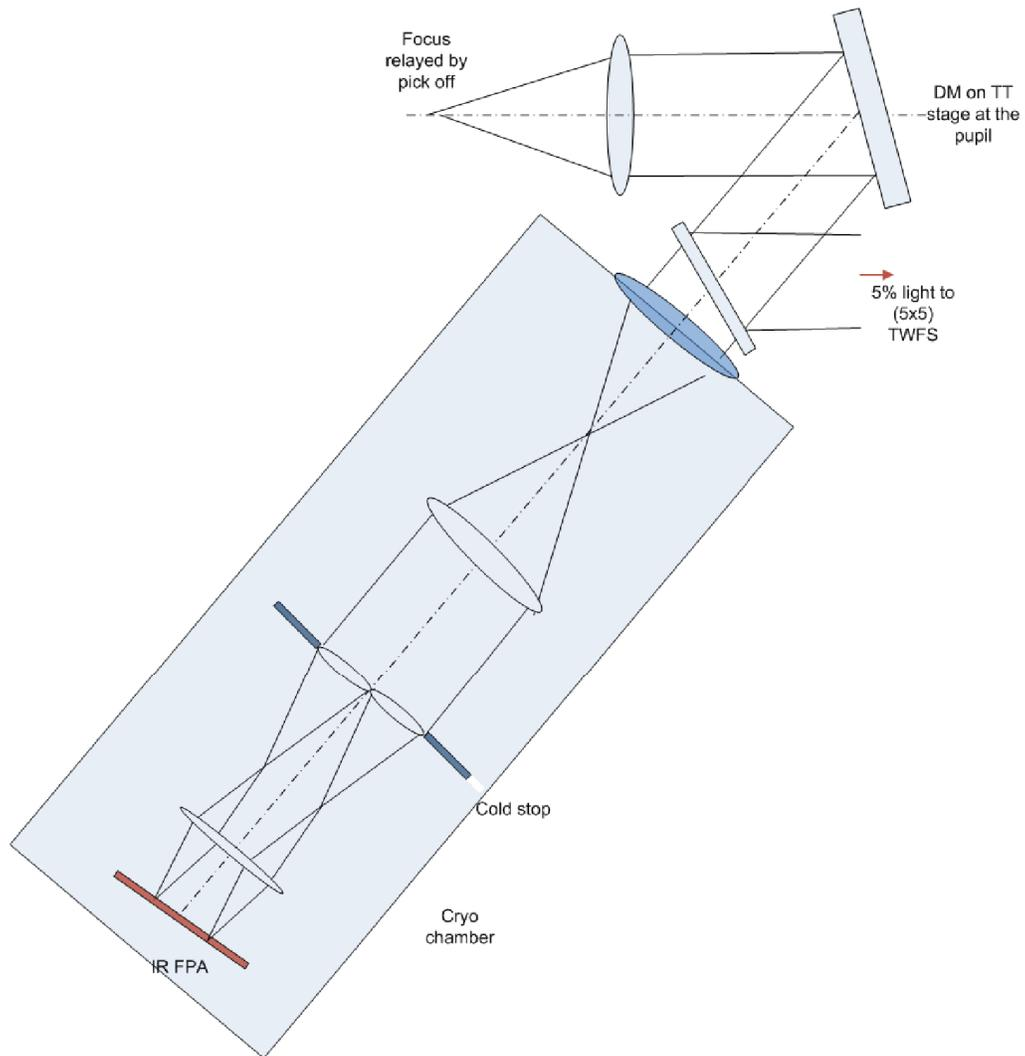
**Figure 1.** Schematic of the Keck NGAO TTFA sensor showing the cold stop and cryogenic part and the (-20 ° C) front end (there is a window between the cold and the cryogenic chamber). TWFS - Truth wavefront sensor, IR FPA - Infra-red Focal Plane Array.
