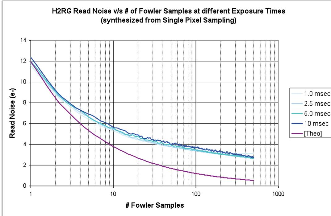
**Figure 7.** Hawaii 2RG measurements - 131,000 samples were acquired at 100 KHz on each of the 32 channels without resetting or clocking. Sequential (non-overlapping) Fowler sampled integration were synthesized from the data stream at various depths to simulate lower pixel visitation rate due to Region-Of-Interest (ROI) readout through a single channel, only every N-th sample.
