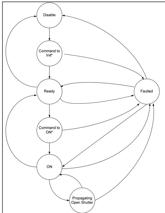
**Figure 4: Laser Controller Sequencer**
