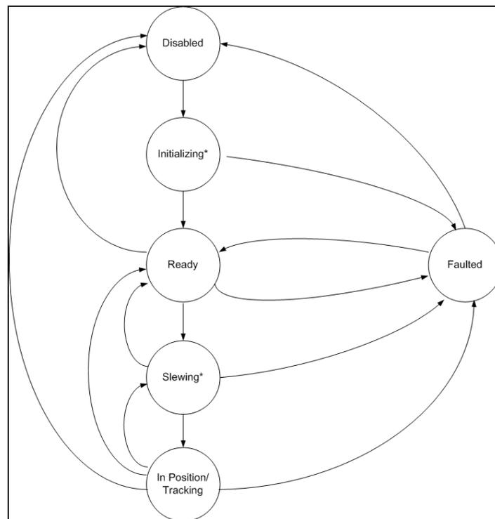
**Figure 2: Example of Sequencer**
