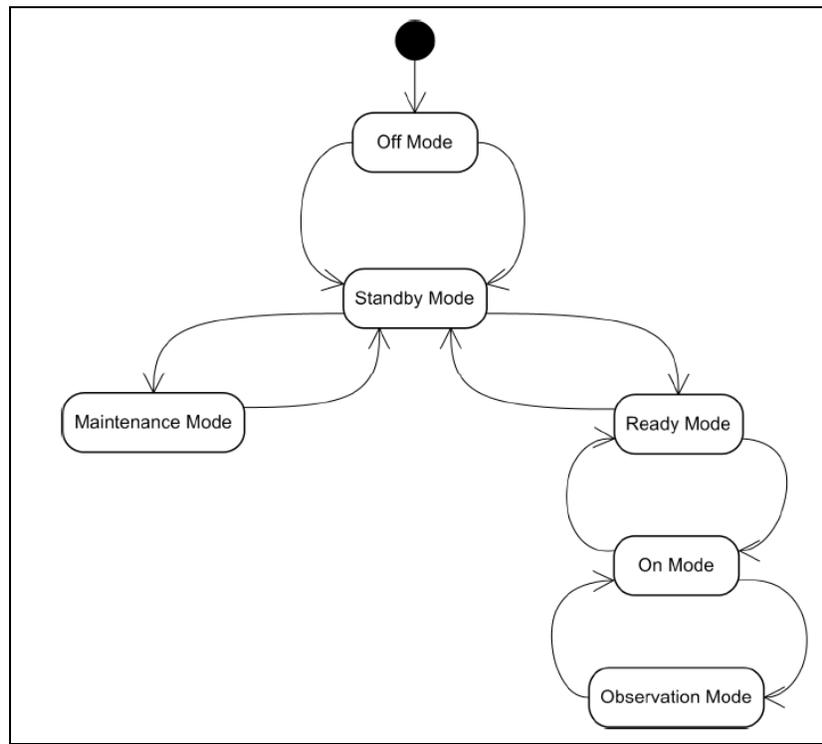
**Figure 3: Laser State Machine**
