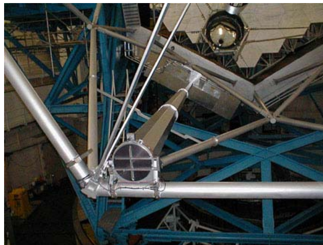
Figure 4: L4 Lens and Structure
