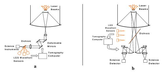
Figure 1 Configurations of astronomical adaptive optics systems: a) multiple conjugate, b) multiple object.
