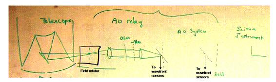
**Figure 3** Generic "conventional" architecture. The AO system is on the Nasmyth. Component blocks are the field rotation mechanism (K mirror), large AO relay which handles the largest field of regard for any downstream science instrument and containing one or more conjugate deformable mirrors, followed by the a possible secondary AO system that might be specialized to the science, e.g. MOAO units, then followed by the science instrument. The front-end relay can act as a common "woofer."
