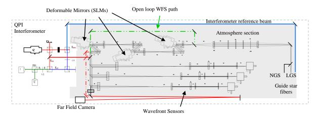
Figure 11 Laboratory for Adaptive Optics MCAO/MOAO testbed layout
