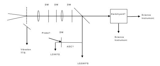
**Figure 4** Generic closed loop architecture. The laser and natural guidestar pickoffs occur after the deformable mirrors. In this configuration, the deformable mirrors must pass the entire technical field containing all the guidestars (exception being the bright guidestar used as a telescope vibration sensor).
