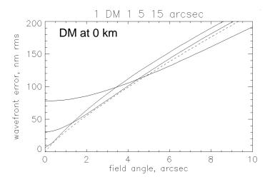
**Figure 9** Anisoplanatic error within an MOAO IFU field. Even though there is only a single DM, correction can be optimized for a prescribed field. The example atmosphere with  $r_0 = 15.6$  cm,  $\theta_0 = 3.1$  arcsec from Figure 3 is also used here.
