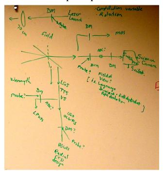
**Figure 5** Generic open loop architecture. Laser and natural guidestars are picked off at the telescope focal plane and sent to the various wavefront sensors. On the science leg are multi-conjugate or multi-object deformable mirror paths.
