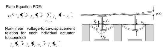
Figure 12 Open-loop modeling of MEMS displacement in response to command voltages.
