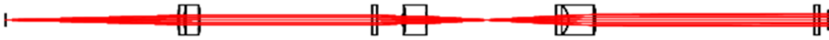
Figure 37: NGS WFS optical elements (field stop at left to CCD at right)
