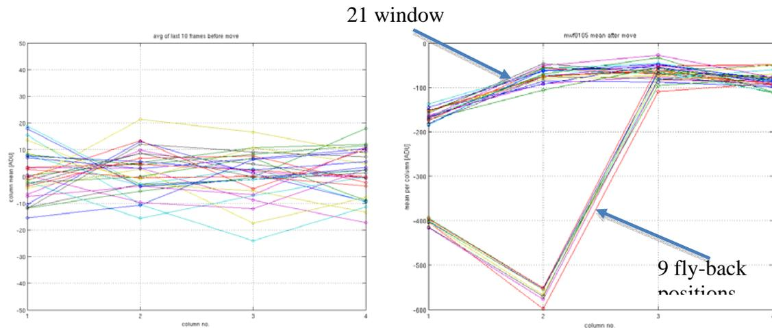
**Figure 7.** Column averages of last 10 frames before and first 10 frames after each window re-positioning. “Fly-back” is when the window moves from position 3 to position 1 again.
