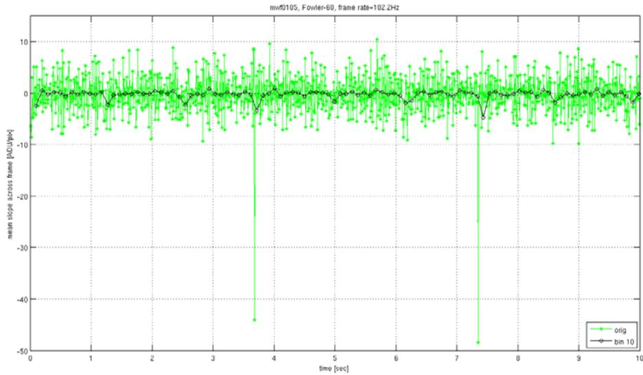
**Figure 15.** Mean slope across frame, per frame, shown as a function of time for the 100Hz synthesized frame rate. In green are shown the original data, 125 100Hz frames per position. A binning factor of 10 was applied, which is shown in black.
