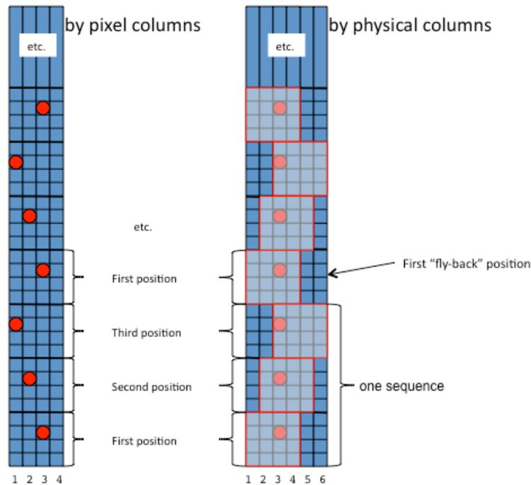
**Figure 3.** Graphical snapshot of the moving window filmstrip data for a 4x4 window. The red dot is a marker for illustrative purposes only, to make the moves visible in the figure. 7500 frames were recorded at each of three window positions (whereas only one frame per position is depicted in this figure), ten sequences of which were recorded in a single FITS file.
