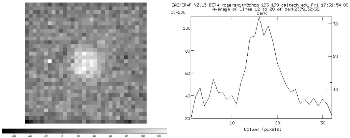
**Figure 1.** At left, evidence of rastering an 8x8 window is seen in a 32x32 window taken immediately after the smaller ROI. At right is a profile taken through the middle of the left-hand image. This is an extreme case where 480,000 8x8 frames (475 $\mu$ sec frame time) were recorded prior to the 32x32.
