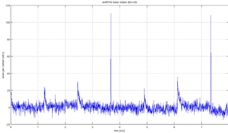
**Figure 8.** Mean slope (bin=20) across frame as a function of time, fitted using four column averages per frame. The two largest, narrow peaks are fly-back positions. The position change around 2.5 seconds is shown enlarged in **Figure 9**. Note this is for raw data in the  $n^{\text{th}}$  frame minus the last frames, a time span much greater than for the actual exposure duration.
