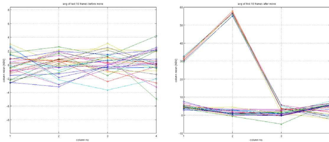
**Figure 18.** Column averages of last ten 1kHz synthesized frames before and first ten frames after a position change. The upper group in the right-hand panel represents the fly-back positions, with the greatest change (on average) being in the 2<sup>nd</sup> column.
