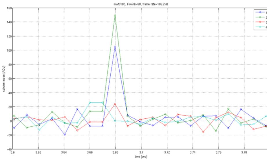
**Figure 12.** A zoom-in of one of the “fly-back” moves for 100Hz synthesized frame rate. From this it appears that only the first two columns are affected, and that they recover in only one frame time.
