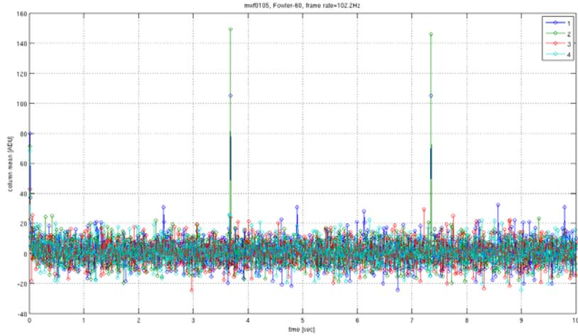
**Figure 11.** Column averages per frame for 100Hz synthesized frame rate for 10s of time that spans eight position changes. The moves at (approximately) 1.25s, 2.5s, 4.75s, 6.25s are barely visible but the “fly-back” moves at 3.75s and 7.5s are easily seen here.
