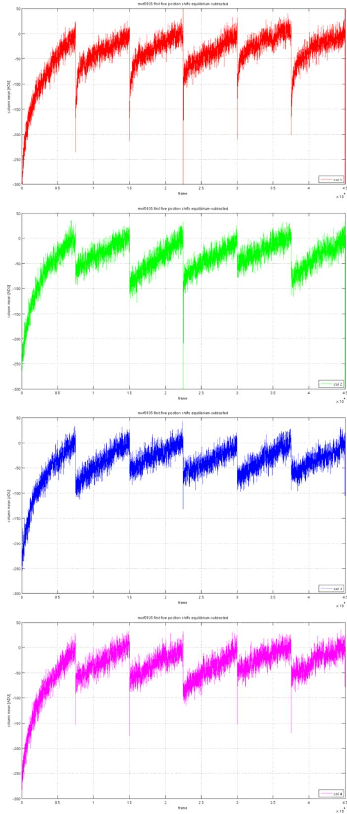
**Figure 6.** Equilibrium-subtracted columns (averaged per frame) for the four pixel columns.
