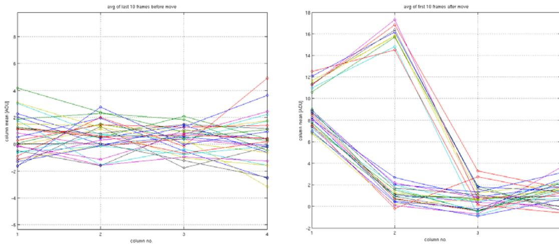
**Figure 14.** Column averages of last ten 100Hz synthesized frames before and first ten frames after a position change. The upper group in the right-hand panel represents the fly-back positions, with the greatest change (on average) being in the 2<sup>nd</sup> column.
