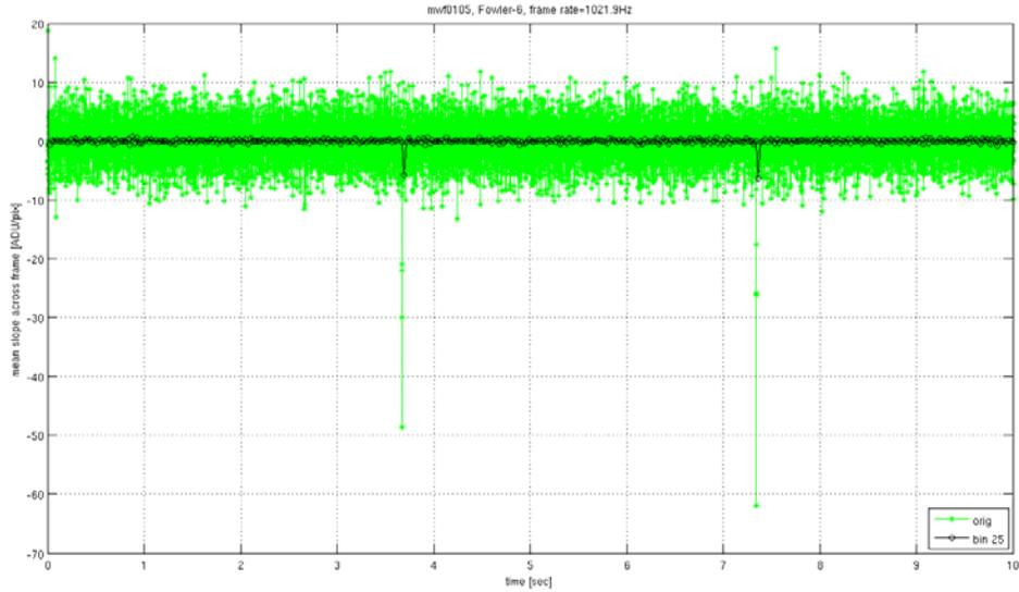
**Figure 19.** Mean slope across frame, per frame, shown as a function of time for the 1kHz synthesized frame rate. In green are shown the original data, 1250 1kHz frames per position. A binning factor of 25 was applied, which is shown in black.
