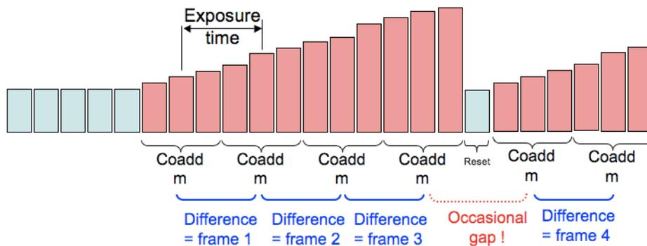
**Figure 10.** In “Differential Multi-Accumulate” readout mode the detector is reset only when necessary to avoid saturation to obtain ~100% duty cycle. Non-destructive reads are averaged and exposures are synthesized by differencing averaged frames.
