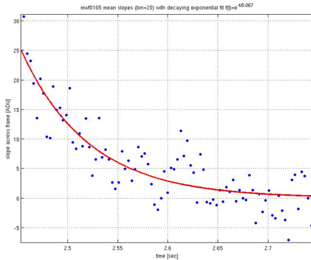
**Figure 9.** Enlarged view of region of **Figure 8** (mean slope across frame as a function of time). An exponential curve is fit to this region with an exponential decay time constant of  $\sim 70\text{msec}$ . For exposure times much less than this characteristic time constant the effect will be significantly attenuated.
