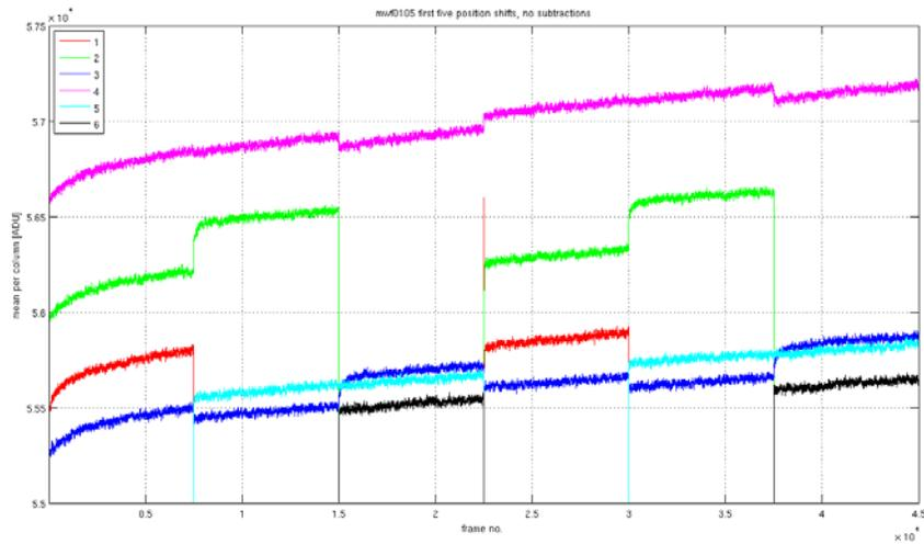
**Figure 4.** Raw data for the first five position shifts. The columns are treated independently; each trace is the mean pixel value in a column, shown as a function of frame. The six traces refer to the six physical columns depicted in **Figure 3**. Gaps for some columns correspond to time that the ROI did not fall on that column.
