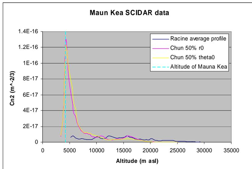
**Figure 2.** Comparison of Average  $C_n^2$  Profile from Racine compared to  $\theta_0$  50% and  $r_0$  50% profiles from Chun, note this is a linear scale. The scale is adjusted to better show the boundary layer, also see Figure 1.
