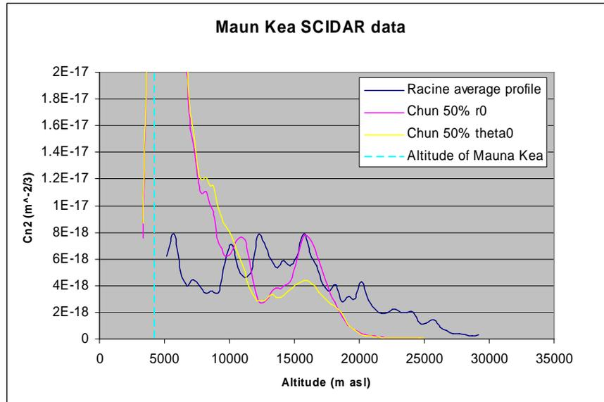
**Figure 1.** Average  $C_n^2$  Profile from Racine compared to  $\theta_0$  50% and  $r_0$  50% profiles from Chun, note this is a linear scale. The scale is adjusted to better show the high-altitude layers, also see Figure 2.
