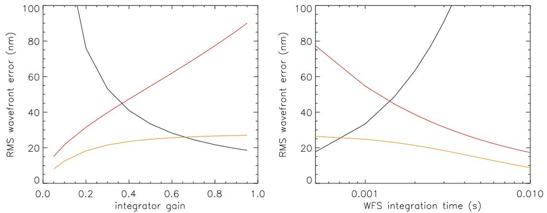
Figure 3: Servo-lag (black line), noise (red) and aliasing (orange) wavefront errors as functions of the integrator gain  $g$  (left) and the WFS integration time  $t_i$  (right).
