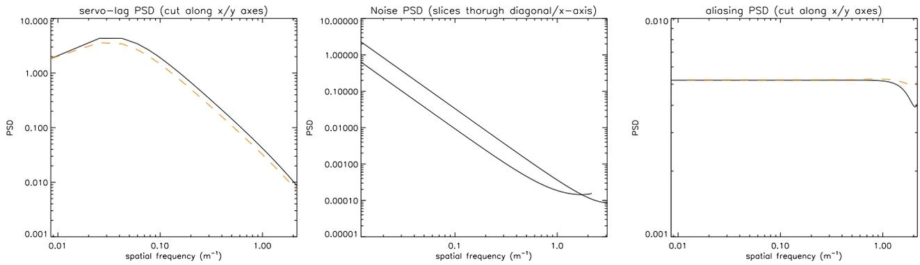
Figure 2: One-dimensional cuts through the 2D PSDs in Figure 1. Servo-lag and noise can be approximated over the majority of the frequency range by  $-5/3$  and  $-2$  power laws, respectively. Aliasing is essentially flat.
