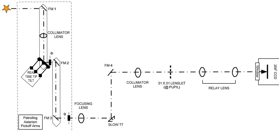
**Figure 8: Schematic of Single LGS WFS Channel (adapted from KAON 692)**
