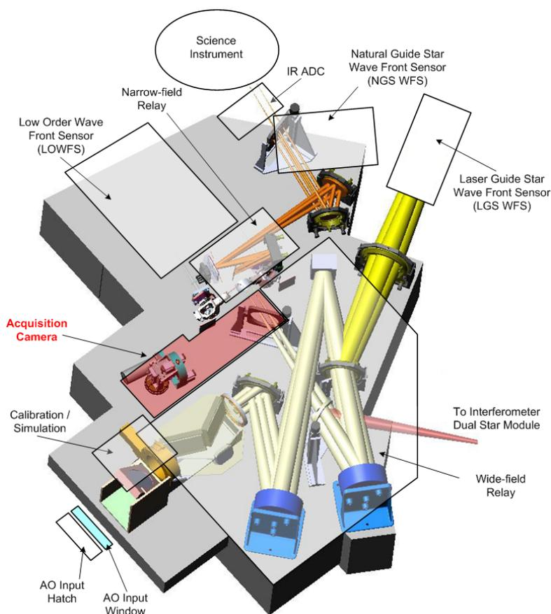
**Figure 9: Location of Acquisition Camera and related optics**
