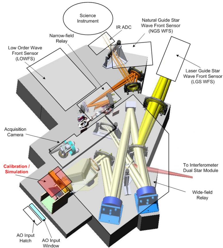
**Figure 7: Location of LGS Wave Front Sensor**
