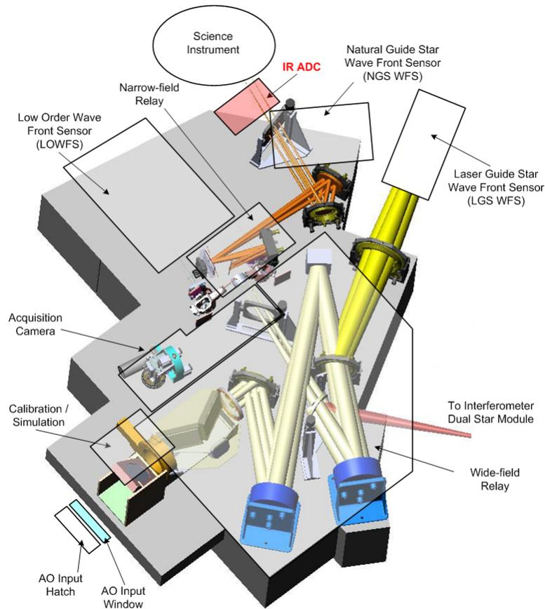
**Figure 16: Location of Atmospheric Dispersion Compensator**
