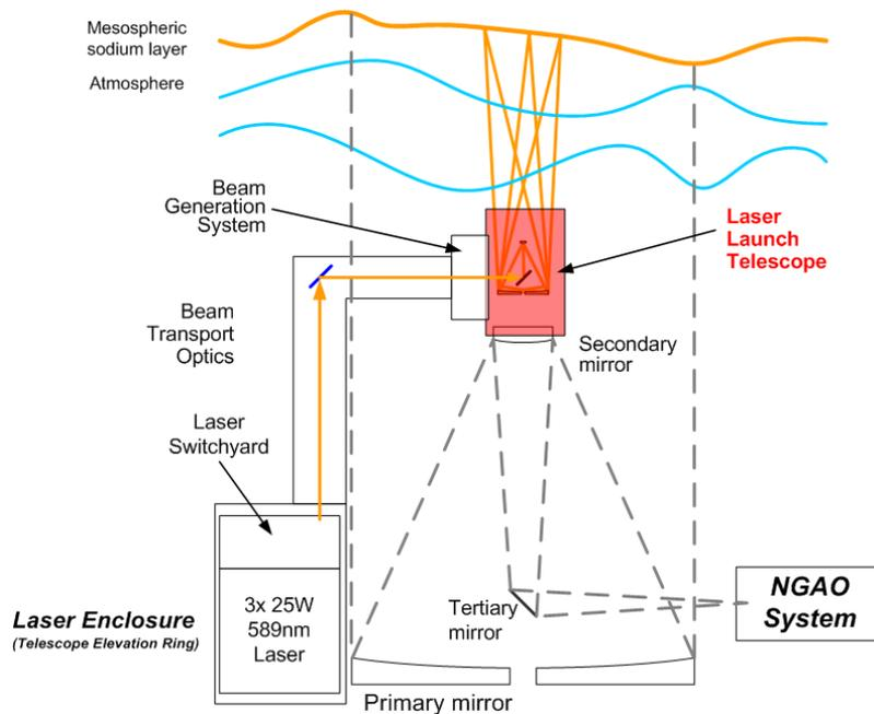
**Figure 21: Location of Laser Launch Telescope**
