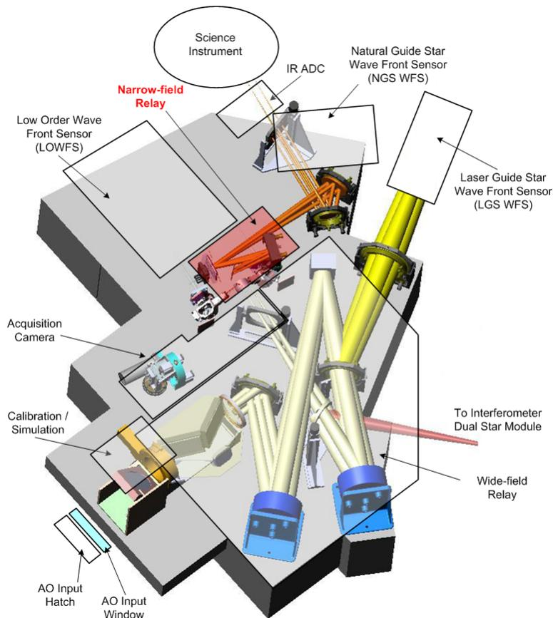
**Figure 12: Location of Narrow-field Relay**
