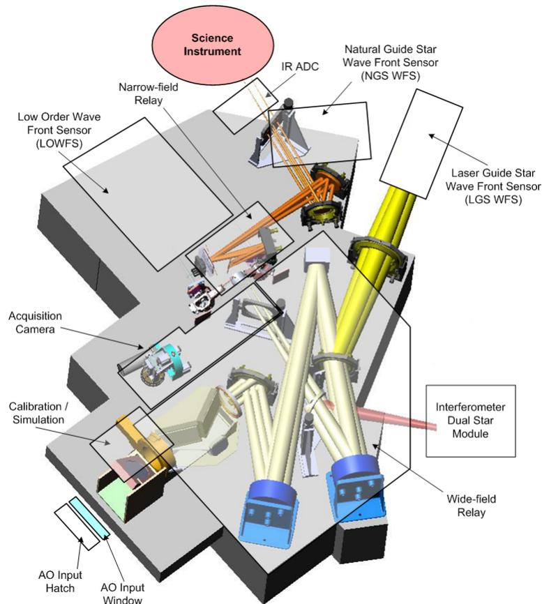
**Figure 23: Location of Narrow-field Science Instrument**
