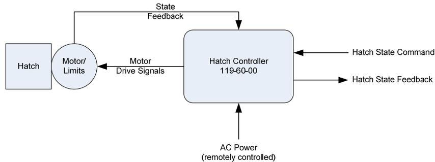
**Figure 3: Schematic of AO Hatch**
