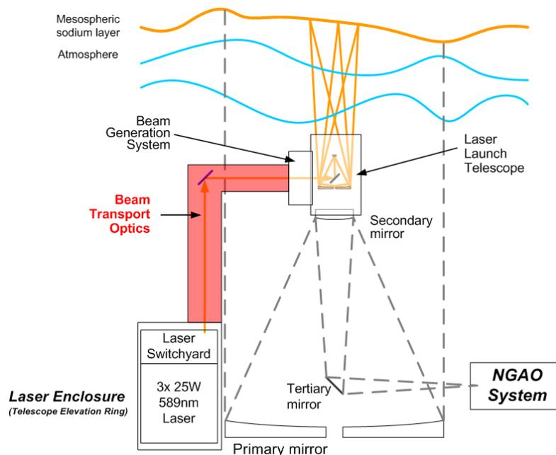
**Figure 19: Location of Beam Transport Optics**
