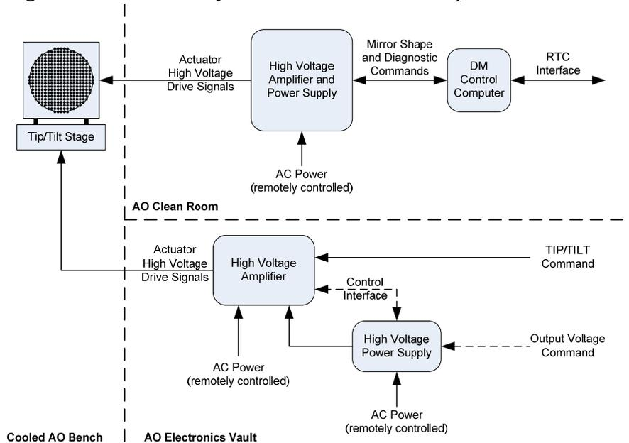
**Figure 13: Schematic of Narrow-field Relay**
