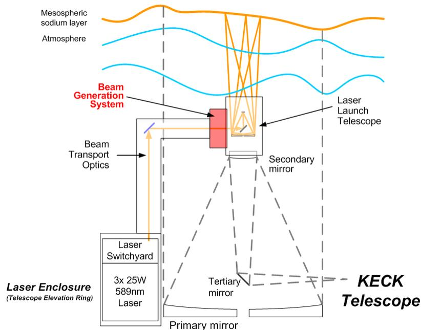
**Figure 20: Location of Beam Generation System**
