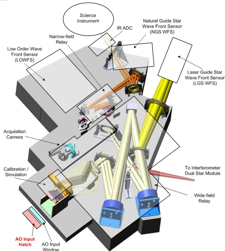
**Figure 2: Location of AO Input Hatch**
