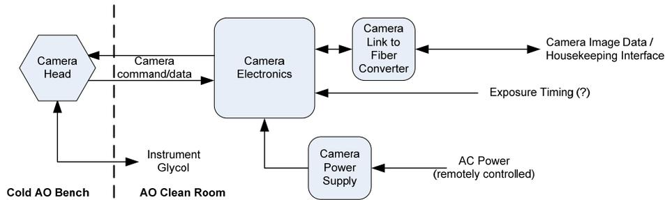
**Figure 10: Schematic of Acquisition Camera**
