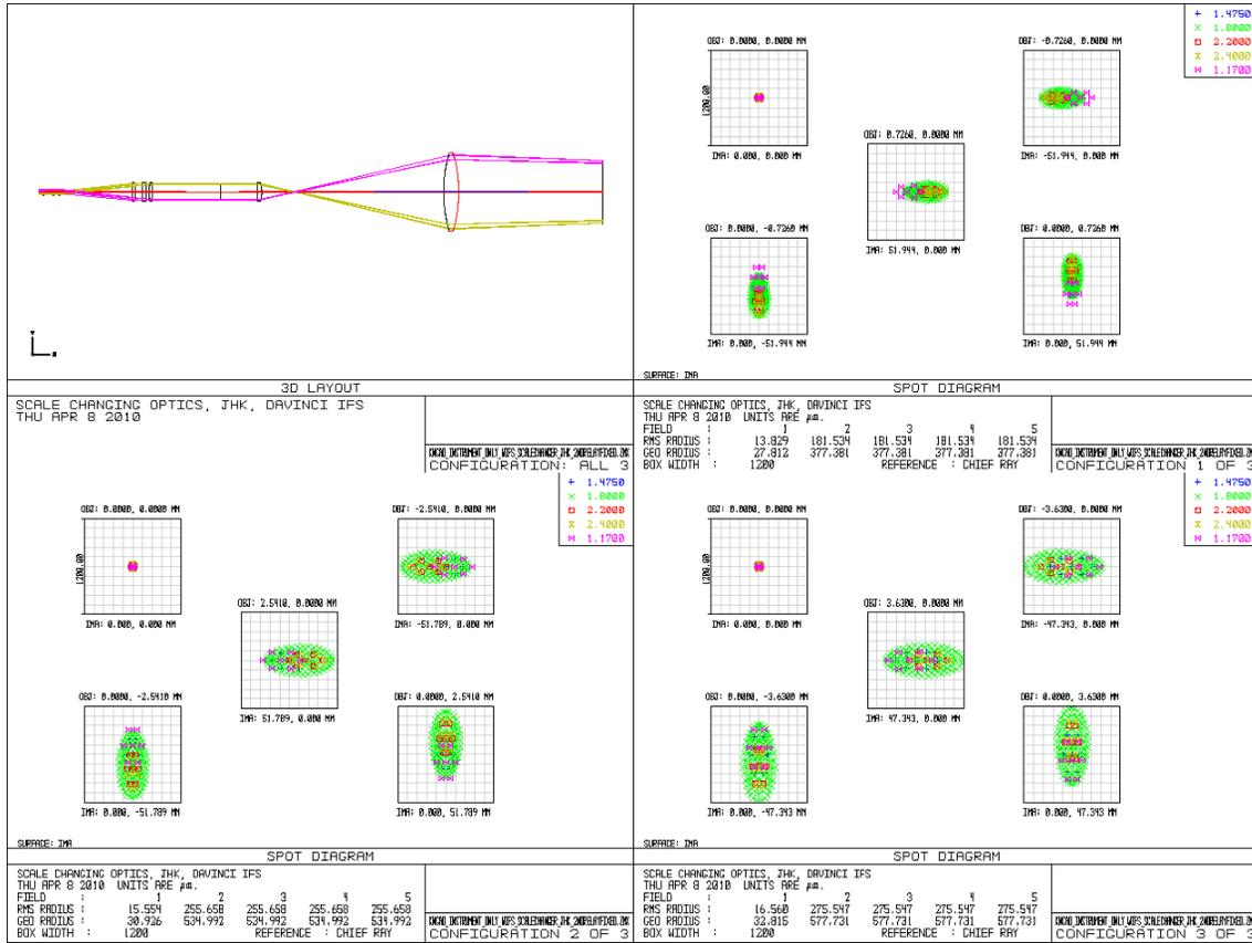
Figure 18: Geometrical spot analysis, JHK band scale changer
