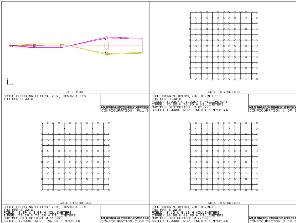
**Figure 19: Grid distortion analysis, JHK-band scale changer**
