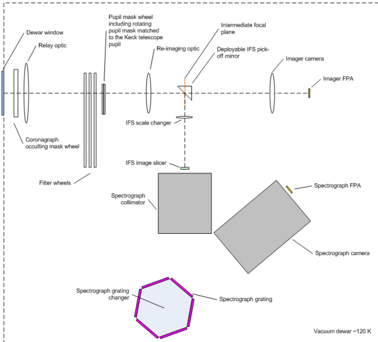
Figure 4: DAVINCI opto-mechanical block diagram (not to scale)
