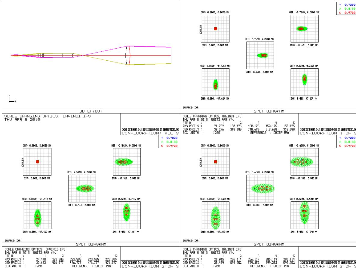
Figure 16: Geometric spot analysis of visible scale changer
