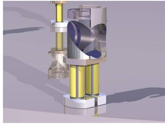
Fig. 2. Left; A representation of a generic Starbug concept for a focal plane pickoff system with Starbugs and base station unit pairs, this basic concept is also applicable to the MOMSI instrument concept. Right; A detailed representation of a Starbug unit carrying a mirror and lens payload.
