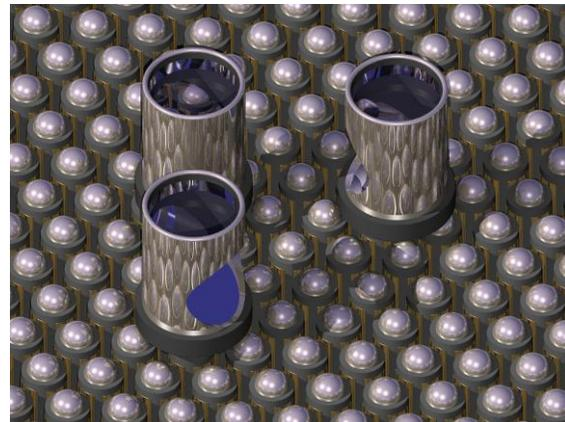
Fig. 3. Left; Starbug-CS, with passive bugs on an active field plate comprised from a “field” of quadrant piezo tubes. Right; Detail of the passive Starbugs of the “Crowd Surfer” concept, each with a lens and fold mirror payload.
