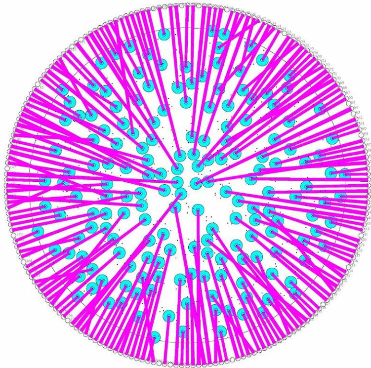
Fig. 9. Simulation of a Starbug allocation given 800 possible targets over field plate 260mm across, with 2mm collimator lenses, 4mm pick-up lenses, 10mm bug diameters. In this case 178 out of 200 Starbugs are allocated.
