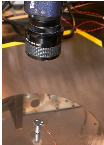
Fig. 8. Metrology and feedback control system for the Starbug prototype. The camera/lens combination is at the top of the photograph and in the lower part of the photograph Res-J has a positioning target attached on top sitting on the test field plate.
