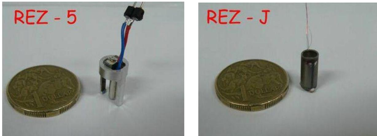
Fig. 5. Left; Rez-5, a late generation piezo stack resonance based Starbug prototype next to an Australian dollar coin (~24mm in diameter). Right; Rez-J, a quadrant piezo tube resonance based Starbug prototype next to an Australian dollar coin.
