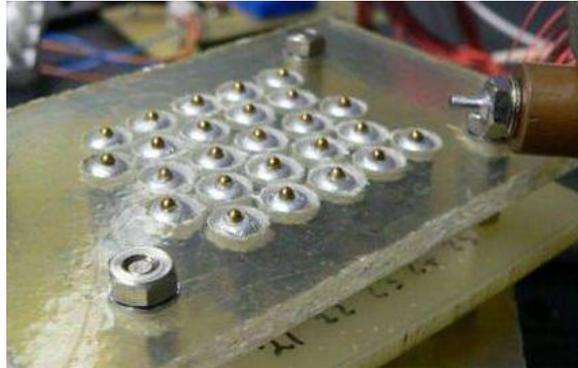
Fig. 7. A photograph of the Crowd Surfer active plate, a quadrant piezo tube based active focal surface. The passive Starbug units that sit on top of the quadrant tubes are not shown in this photograph.
