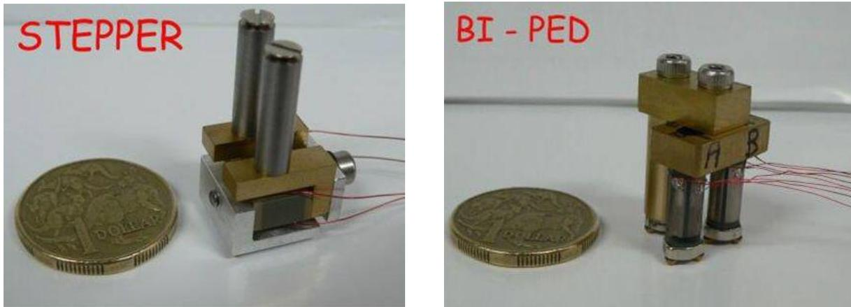
Fig. 6. Left; Stepper, a piezo stack inertial stick-slip based Starbug prototype, photographed next to an Australian dollar coin. Right; Bi-Ped, a quadrant piezo tube inertial stick-slip based Starbug prototype photographed next to an Australian dollar coin.
