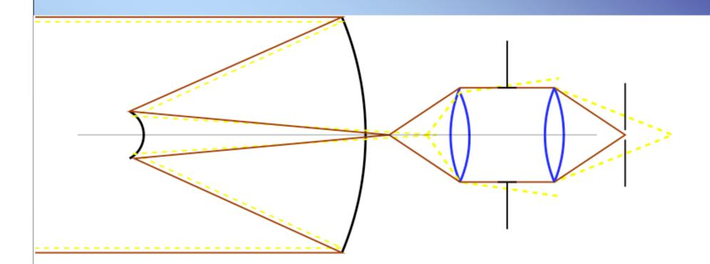
Pupil stop and baffles around the optics of the AO system to prevent stray light problems
