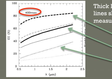
Thick lines show GLAO and thin lines show seeing-limited measurements.
