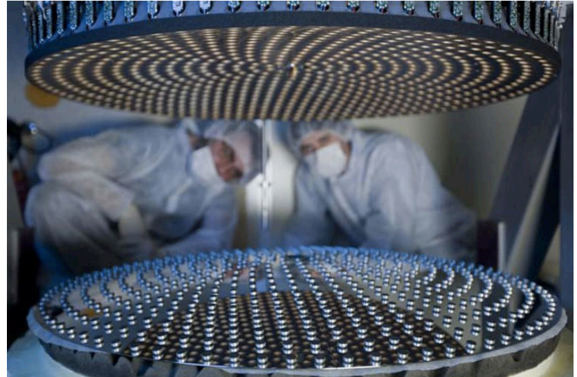
Reference body (top) and thin shell (bottom) showing the magnets on the rear of the shell.
