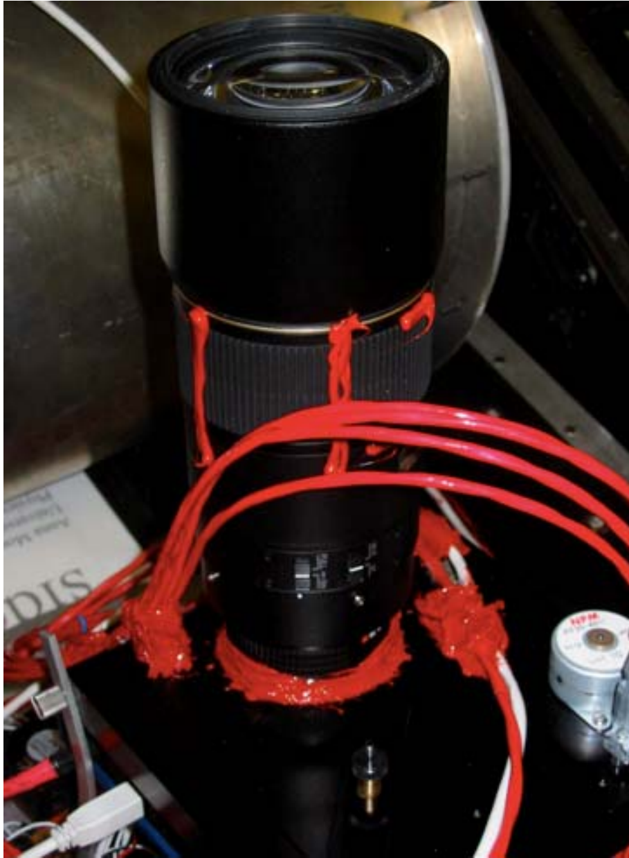
Figure 7 : The Gattini DomeA SBC camera seen without the acrylic dome in place.
