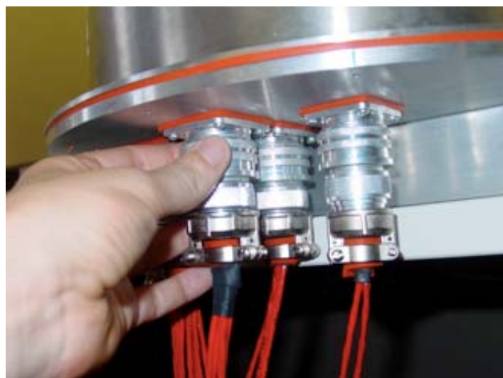
Figure 10 : The cable connectors for the camera enclosures shown before color coding
