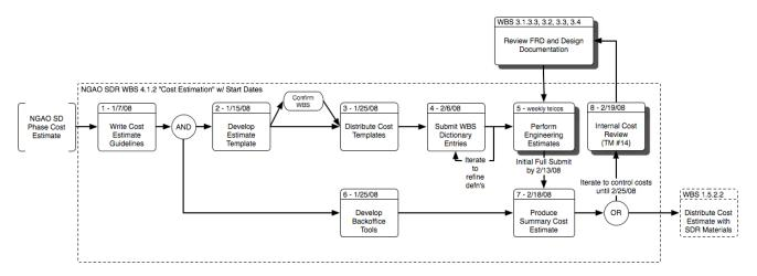
**Figure 1.** NGAO System Design Phase Cost Estimation WBS 4.1.2 Process Flow. Shadowed processes involve all NGAO team Estimators.
