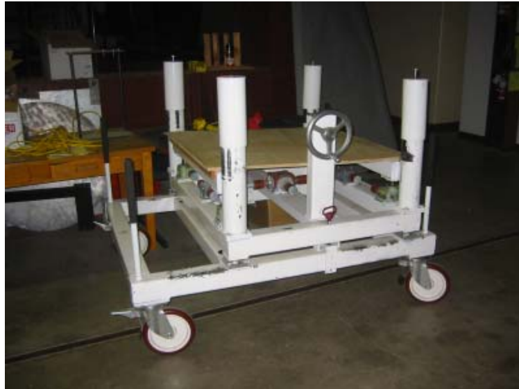
Figure 20: The PALAO handling cart allows adjustment of the PALAO optical bench in X/Y and Z directions. This facilitates quick alignment of the 4 guide pins of the PALAO optical bench with the 4 guide holes of the Cassegrain ring
