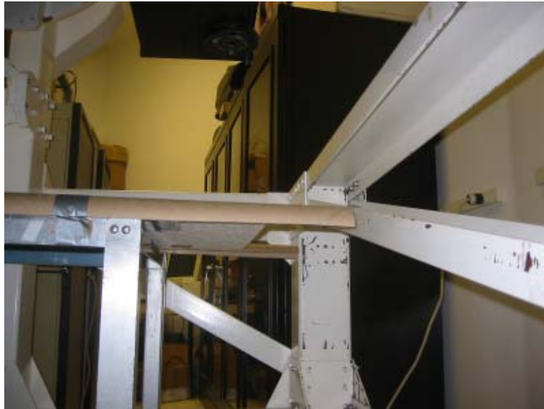
Figure 19: Sufficient clearance exists between the rails and rear cross-member of the AO spit
