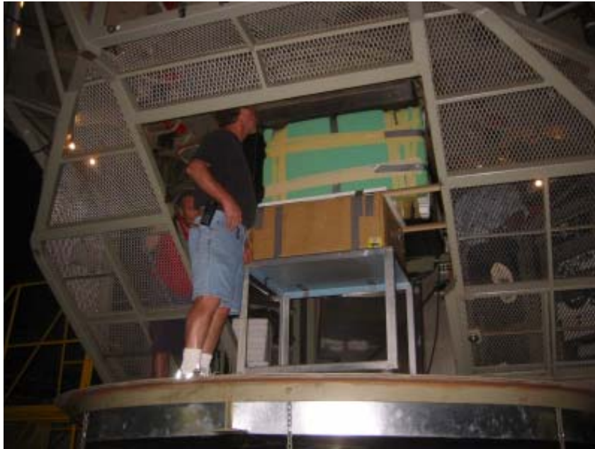
Figure 12: Final adjustment of the SWIFT position to align with the 3 mounting pads located permanently on the AO bench (representative in this photo)
