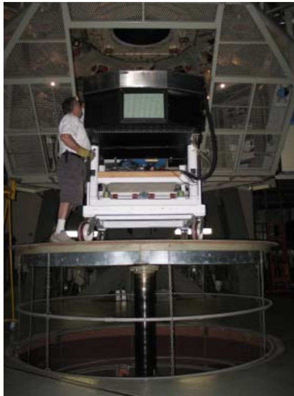
Figure 5: Careful lifting of the AO cart with PALAO system through the entrance of the Cassegrain cage under careful supervision by Steve Kunsman.
