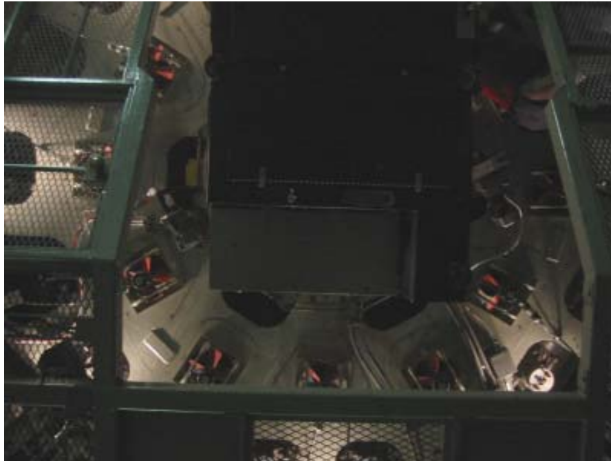
Figure 8: A view of the PALAO bench mounted on the Cassegrain ring of the 200'' Hale telescope immediately after installation. No science instrument is mounted to the bench.
