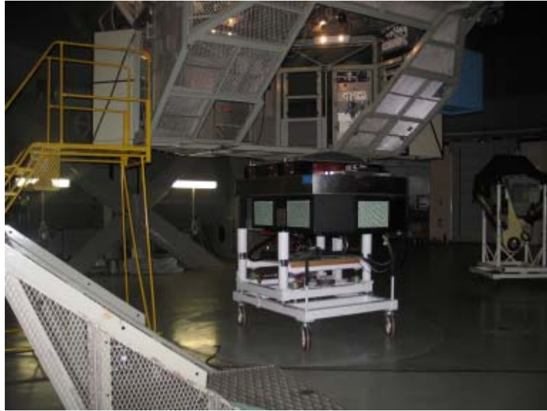
Figure 4: The PALAO optical bench supported by the AO cart prior to lifting into the Cassegrain cage. The AO cart is orientated into the correct position on the hydraulic platform.
