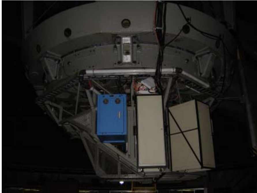
Figure 2: Electronics racks mounted to the outside of the Cassegrain cage. Instrument specific racks are removed with the instrument to allow testing off the telescope.
