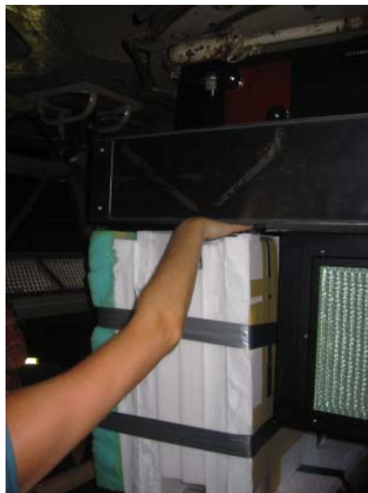
Figure 13: There is 20mm of clearance between the SWIFT enclosure and the PALAO optical bench to allow insertion of a tool that secures the 3 mounting pads.
