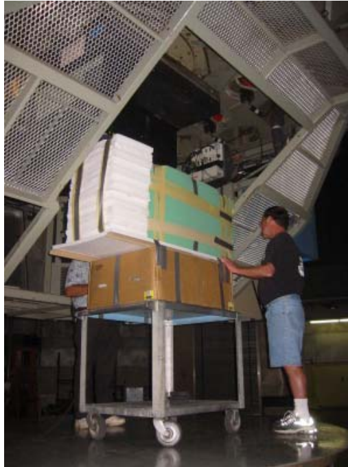
Figure 10: A mock-up of the SWIFT handling cart and instrument, placed on the hydraulic platform in the correct orientation
