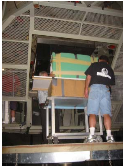
Figure 11: The SWIFT handling cart is adjusted in position when the widest dimension has cleared the narrowest section of the cage opening. Note that part of the foam section representing SWIFT has been removed to avoid conflict with the current AO enclosure
