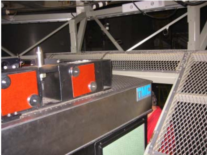
Figure 6: The PALAO optical bench entering the Cassegrain cage. One of the 4 guide pins is shown top-left
