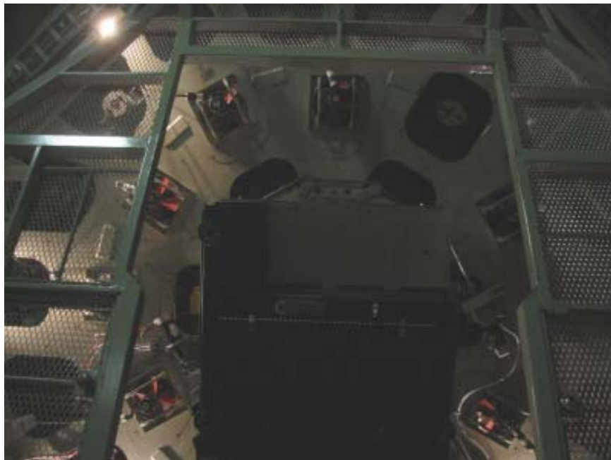
Figure 9: The PALAO bench is rotated on the Cassegrain ring by 180° prior to installation of the SWIFT instrument
