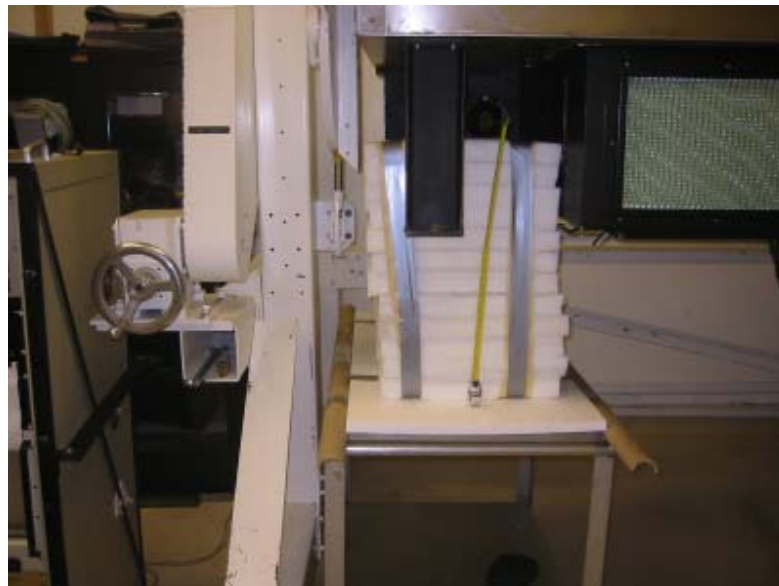
Figure 18: Sufficient clearance exists between the left-hand (cardboard) rail and the AO spit support frame
