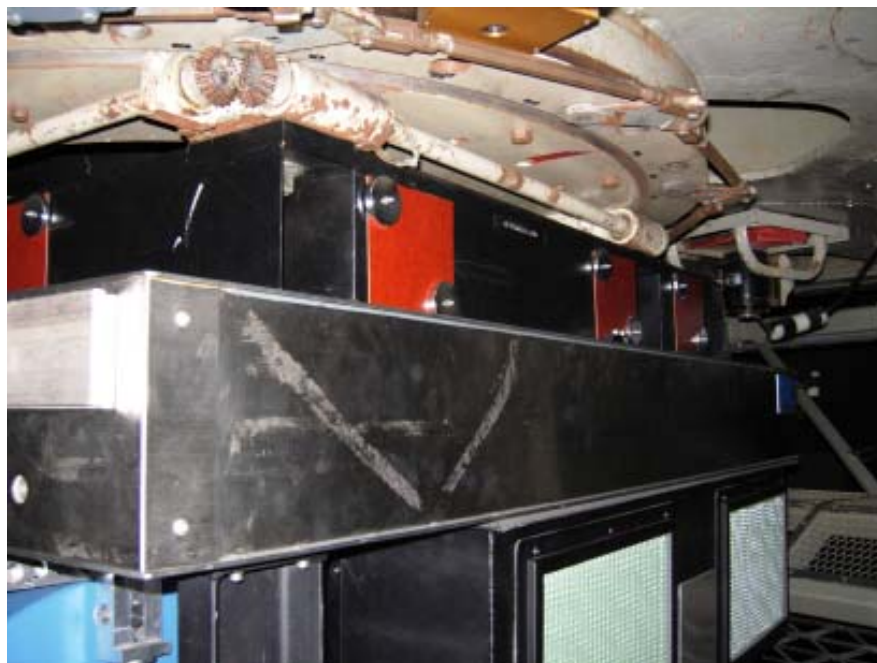
Figure 7: The PALAO bench locked onto the Cassegrain ring
