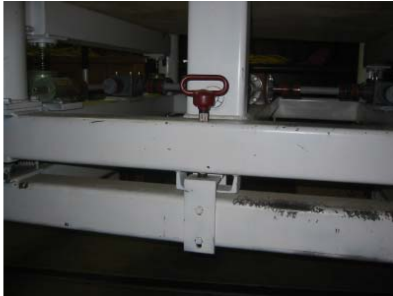
Figure 22: The upper support frame of the PALAO handling cart is locked relative to the lower frame for transport within the dome.
