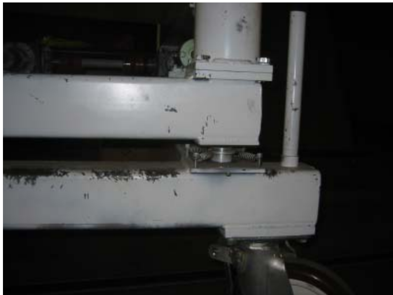
Figure 21: The upper support frame of the PALAO handling cart can move in the X/Y plane relative to the lower frame by means of 4 spring loaded ball bearings, one of which is shown above
