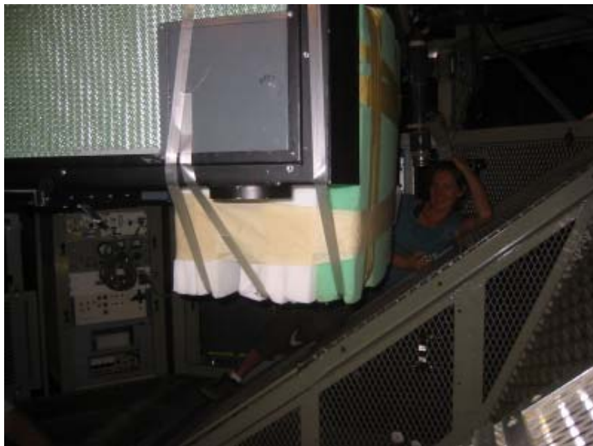
Figure 15: The mock-up SWIFT instrument on the PALAO bench with the Cassegrain cage door in place
