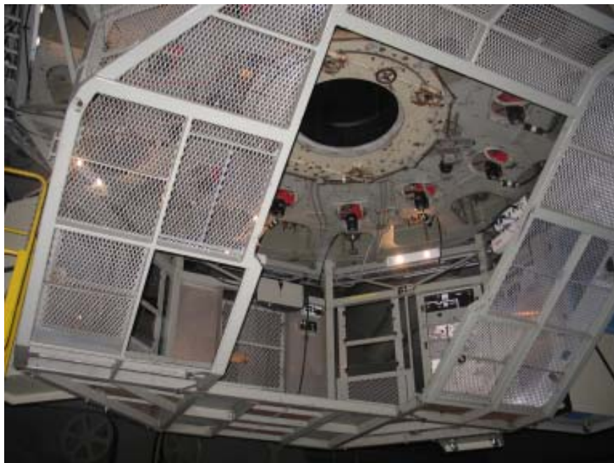
Figure 3: The Cassegrain mounting ring of the 200'' Hale telescope with cage in place. The door of the cage has been removed to permit instrument change.
