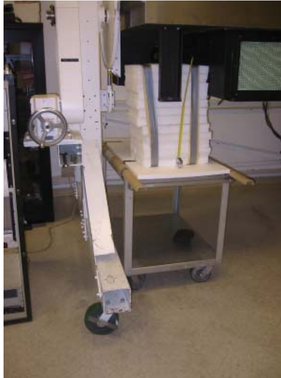
Figure 17: The SWIFT handling cart positioned underneath the AO spit at a suitable height to mount the SWIFT instrument to the PALAO optical bench.
