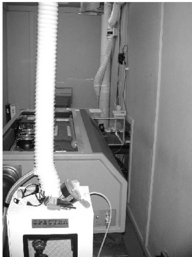
FIG. 4.—Photograph of the Questek laser with the top cover removed. In the foreground is a sealed cabinet holding the fluorine gas with a vent hose exiting the top of the cabinet. The chamber that holds the lasing gas mixture is just to the right of the vent hose, and the laser capacitor banks are below the fans visible on the left of the vent hose. The laser beam exits on the far side of the laser cabinet.
