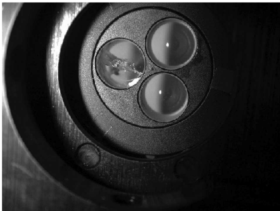
FIG. 9.—Greatly enlarged image of the diverging lens holder. While three lenses are held by a single mount, only one is used at a time. Two pristine diverging lenses can be seen on the right, and the one damaged diverging lens is on the left. The damage occurred when the energy density sent into the lens exceeded 6 \text{ J cm}^{-2} at the rear surface of the lens. To set a scale for this image, each lens has a diameter of 7.4 mm.
