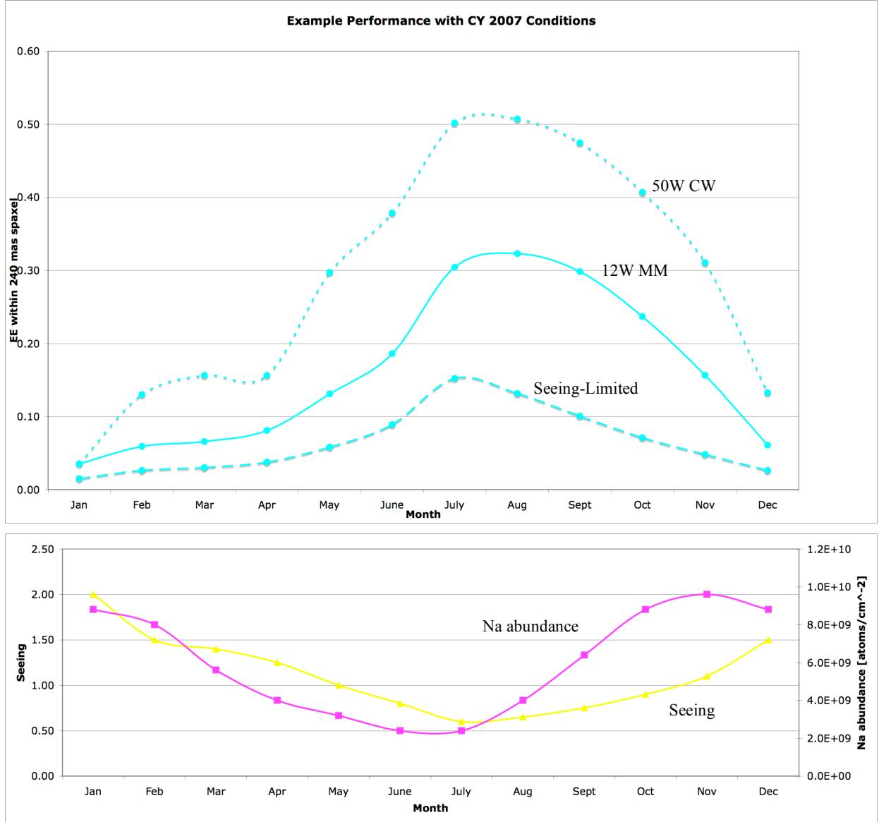
Figure 2. Example PALM-3000 + SWIFT Z-Band (882 nm) Performance vs. Month based upon CY2007 MASS/DIMM seeing and Na abundance estimated from measured CSFL mesospheric photoreturn<sup>5</sup>. The bottommost (dashed) curve represents the 240 mas spaxel EE for seeing-limited PSF. The middle (solid) curve represents what might have been seen in the same spaxel with PALM-3000 (interim LOWFS) with
