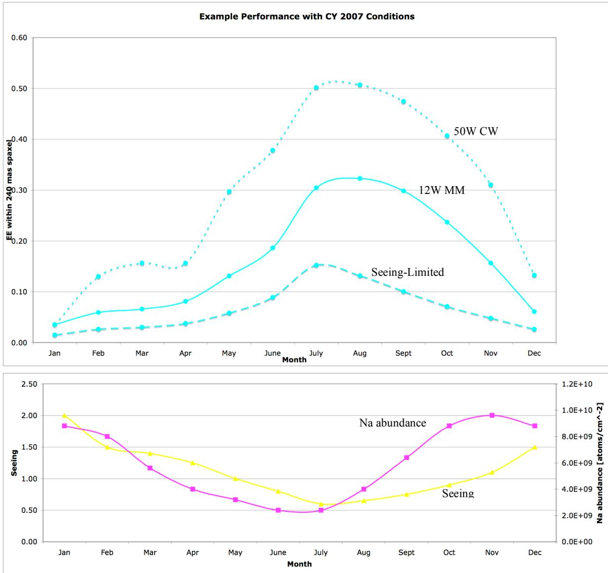
Figure 2. Example PALM-3000 + SWIFT Z-Band (880 nm) Performance vs. Month based upon CY2007 MASS/DIMM seeing and Na abundance estimated from measured CSFL mesospheric photoreturn<sup>1</sup>. The bottommost (dashed) curve represents the 240 mas spaxel EE for seeing-limited PSF. The middle (solid) curve represents what might have been seen in the same spaxel with PALM-3000 (interim LOWFS) with
