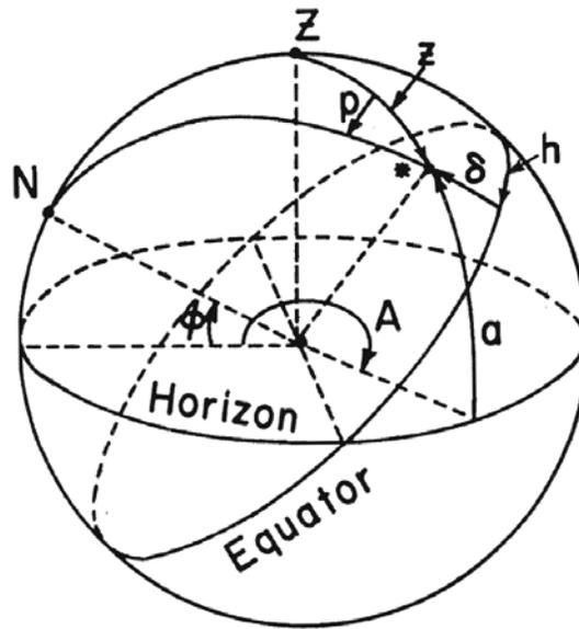
**Figure 2:** Standard altitude-azimuth coordinate system. The azimuth ( $A$ ) angle above is defined to start at north moving through east as the positive direction. This is the standard at Keck [1,4]. Other references have different conventions [2,3].
