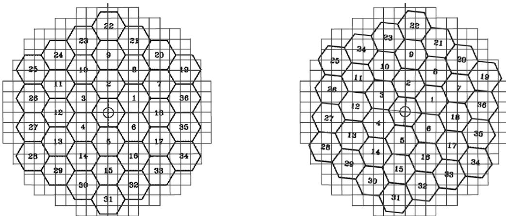
**Figure 1:** The pattern of the 36 segments (hexagons) superimposed on the subapertures of the current Keck wavefront sensors. The image on the right has a rotation of the Keck Pupil of 6 degrees with respect to the left hand image. An example of a dramatic illumination change is the subaperture at the top left side of segment 22. It goes from partial illumination to almost no illumination as the pupil rotates in the images above.
