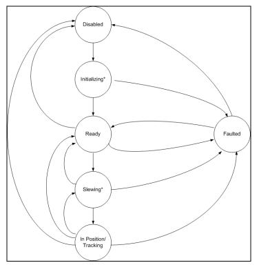
Figure 2: Example of Sequencer
