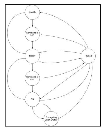
Figure 4: Laser Controller Sequencer
