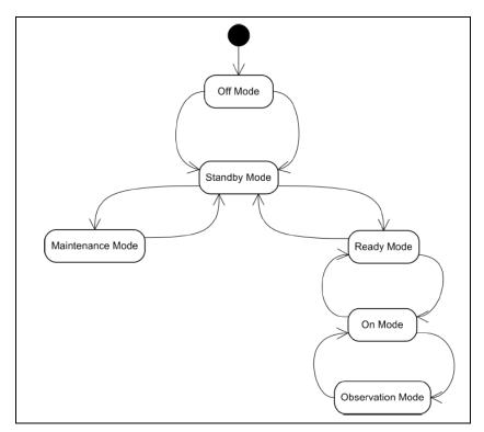
Figure 3: Laser State Machine
