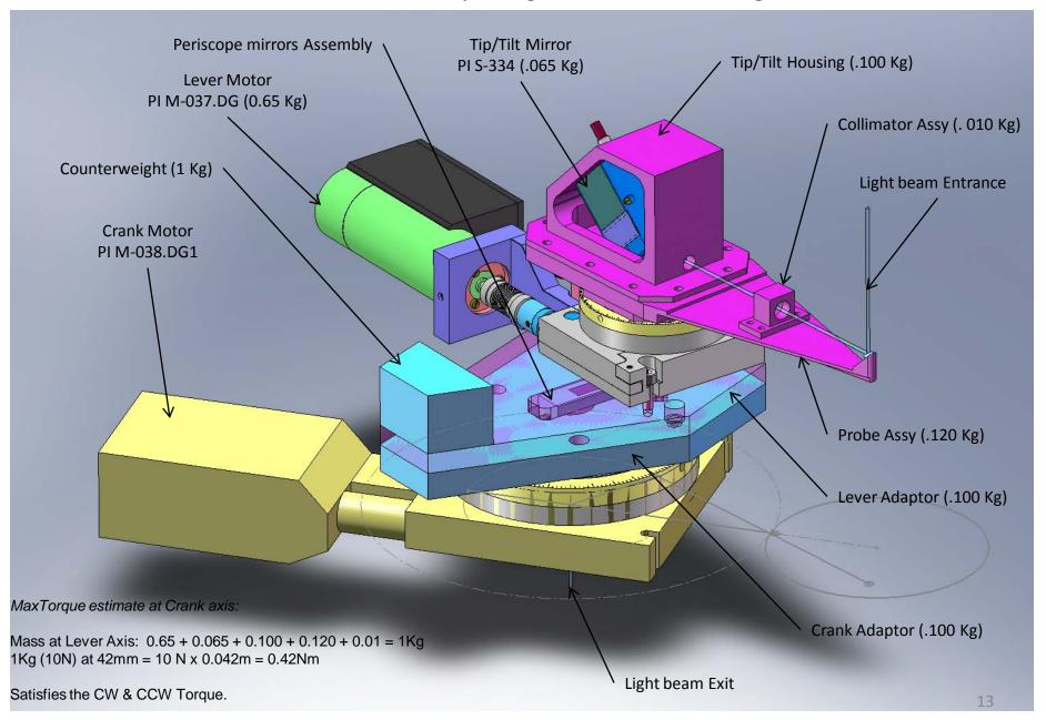
Crank & Lever Motor @ 0°: Probe at 0° (Arm Fully Retracted)
