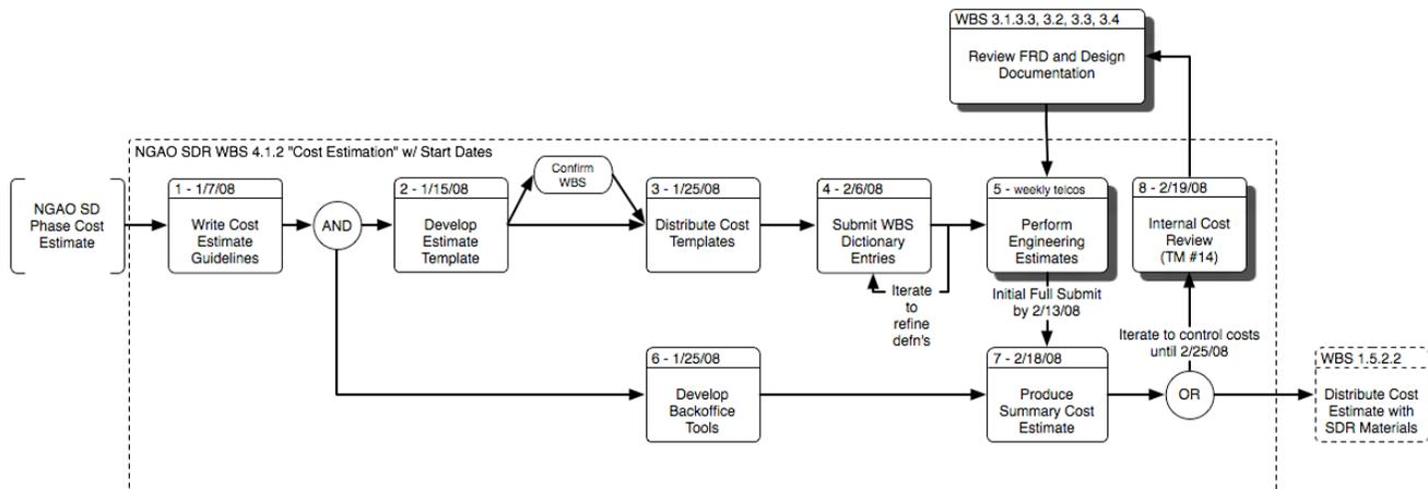
**Figure 1.** NGAO System Design Phase Cost Estimation WBS 4.1.2 Process Flow. Shaded processes involve all NGAO team Estimators.
